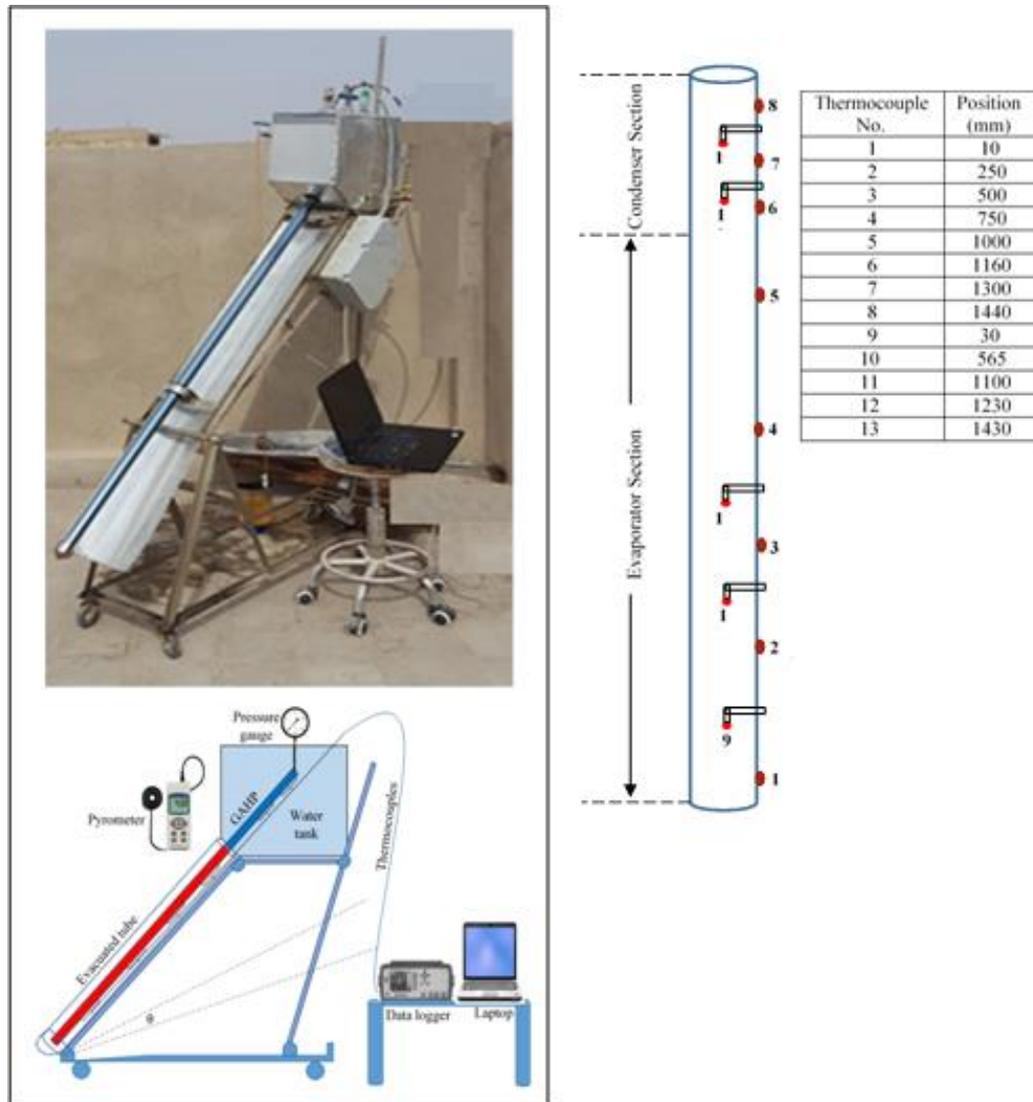
**Fig. 1:** The schematic diagram and a photo of experimental set up of HP-ETSC.**Fig. 2:** GAHP thermocouple positions (surface wall and core)
