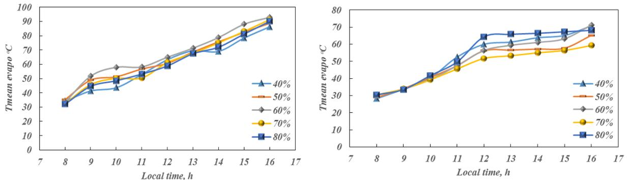
**Fig. 3:** Variation of mean wall temperature of evaporator with fill ratio during solar time at title angle 30°
