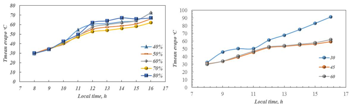
**Fig. 5:** Variation of mean wall temperature of evaporator with fill ratio during solar time at title angle 60°.
