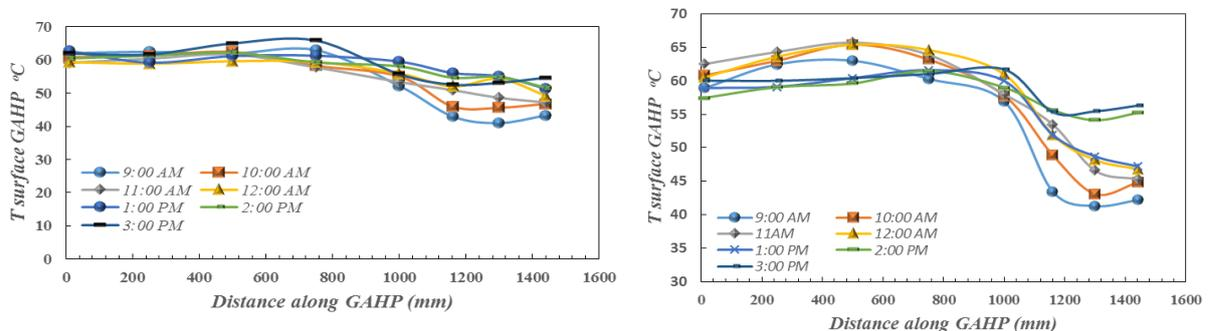
**Fig. 9:** Variation of temperature with the distance along the wall of GAHP at optimal fill ratio 70% during solar time at title angle 45°.
