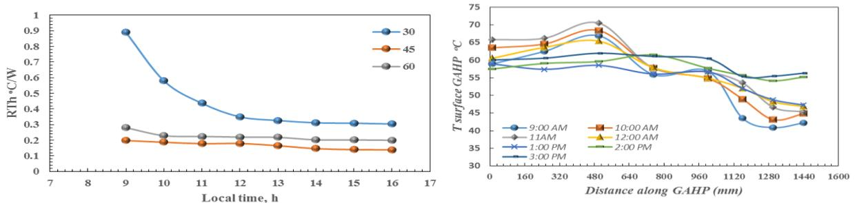
**Fig. 7:** Variation of GAHP thermal resistance for the three angles at optimal filling ratio 70%.
