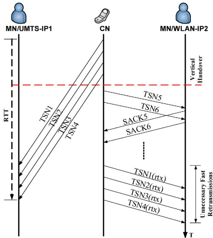
Fig. 4. The packet reordering problem caused by changing the main link to the alternate link. (The colors are visible in the online version of the article.)
