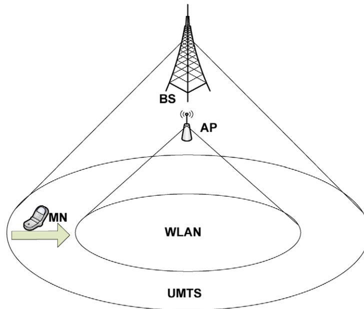
Fig. 2. Vertical handover heterogeneous network. (The colors are visible in the online version of the article.)
