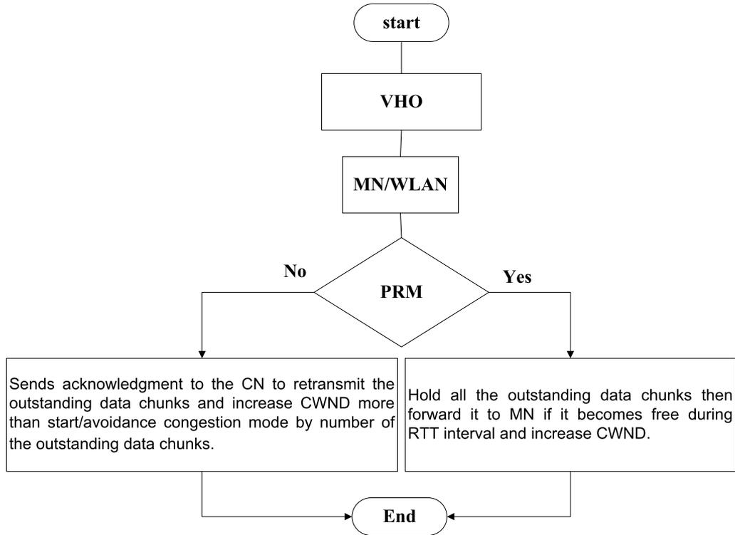
Fig. 6. Flowchart of the procedure of PRM when VHO occurs in UMTS/WLAN networks.
