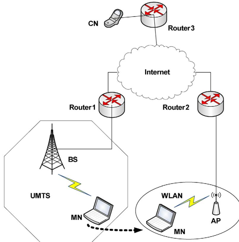
Fig. 3. Vertical handover between UMTS/WLAN networks. (The colors are visible in the online version of the article.)
