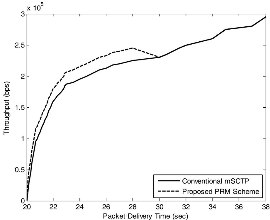
Fig. 7. Throughput of conventional mSCTP and proposed PRM scheme.
