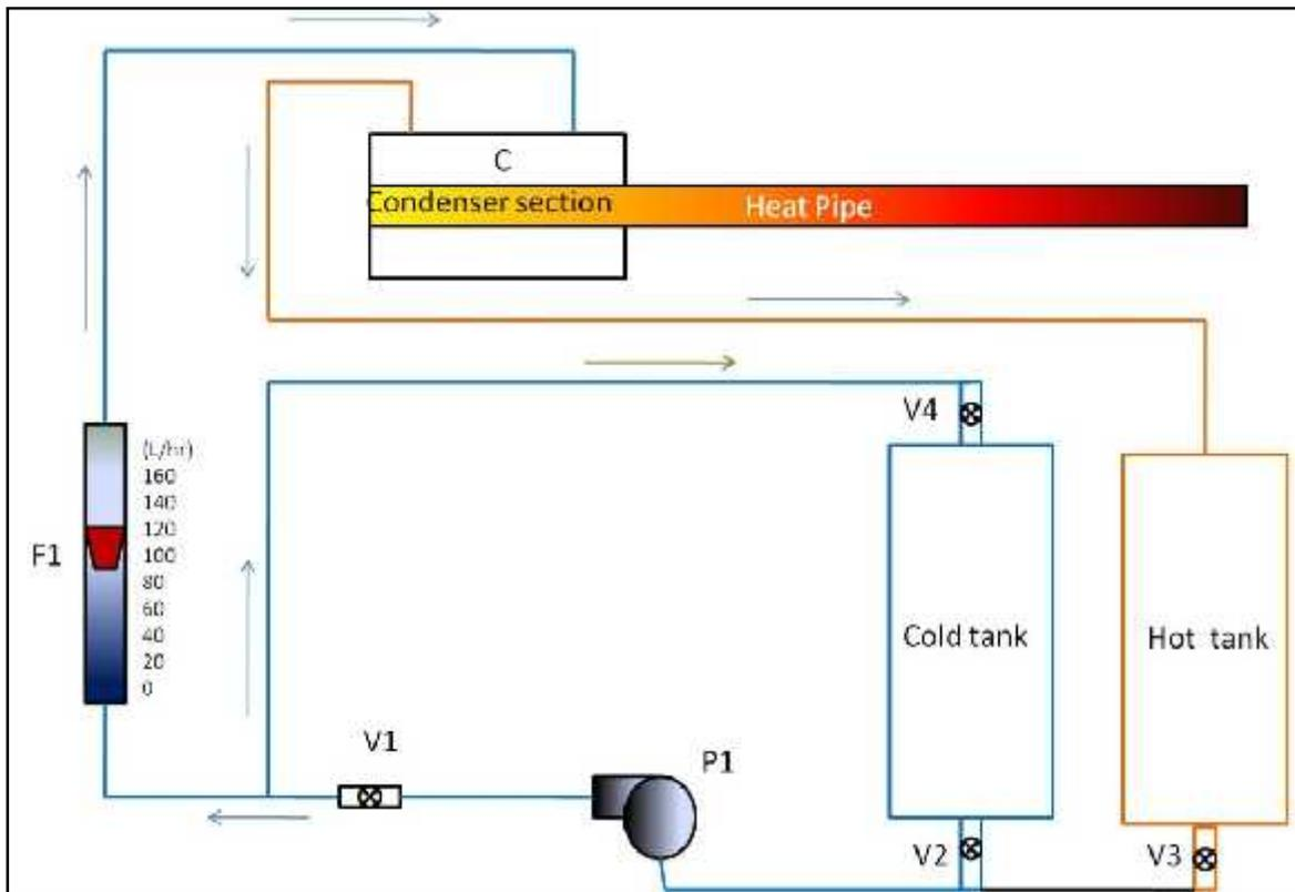
**Fig.5:** Cooling System of heat pipe [Present work]
