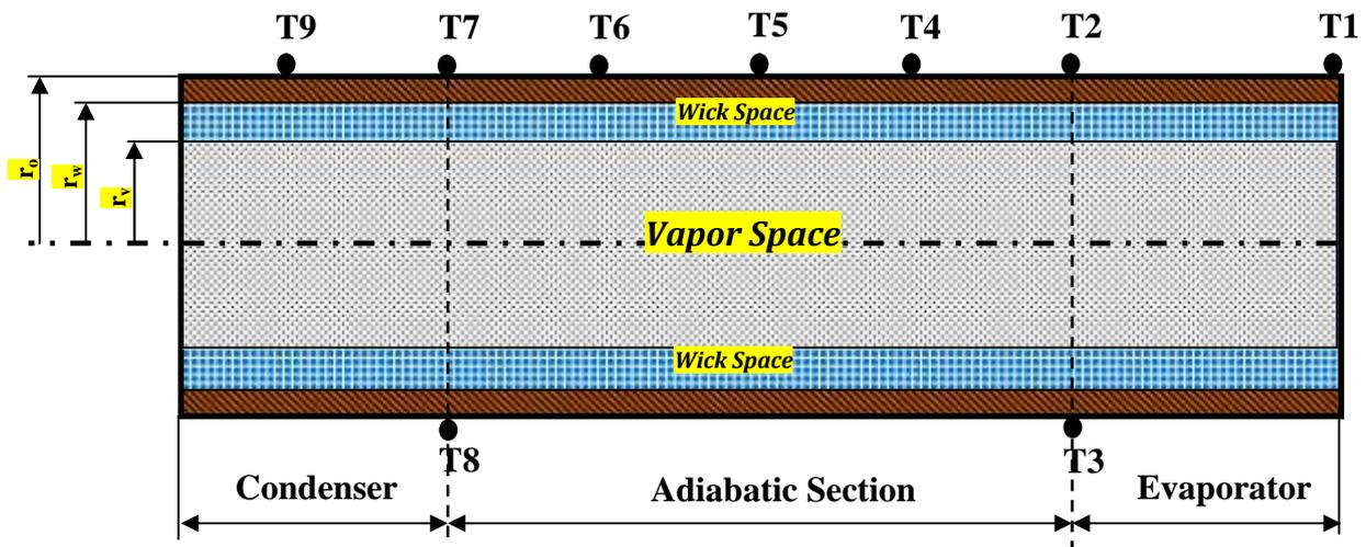
**Fig.6:** heat pipe thermocouples locations [Present work]
