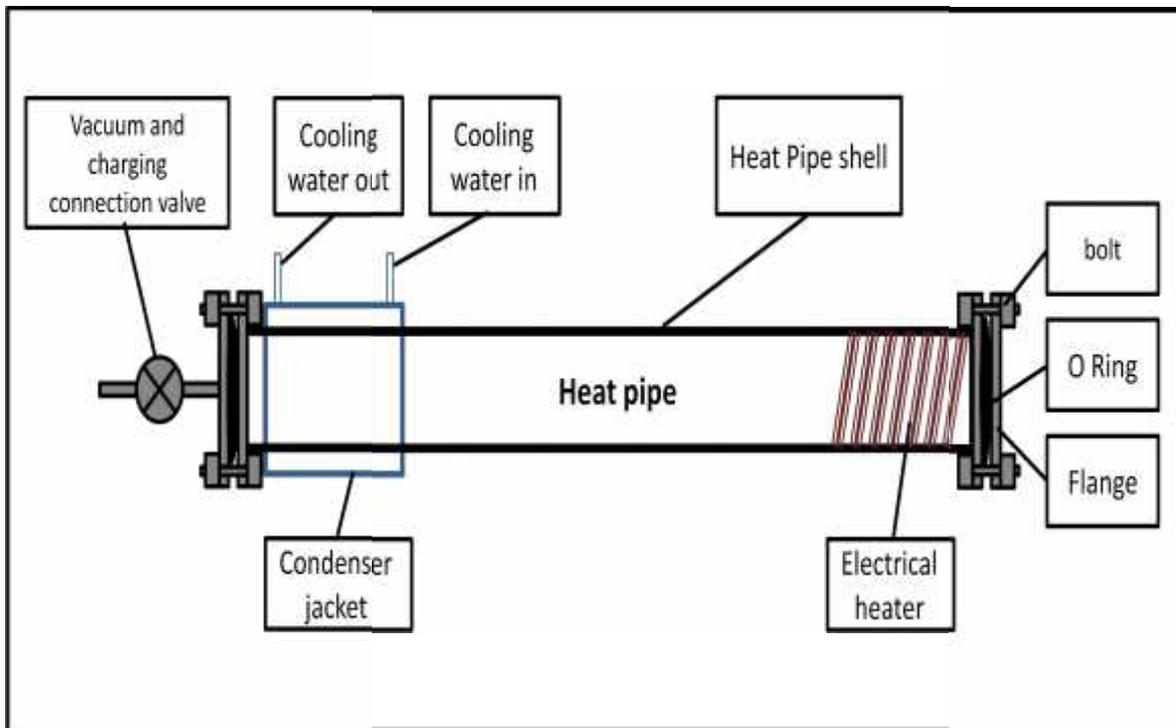
**Fig.2:** Heat pipe construction [Present work]
