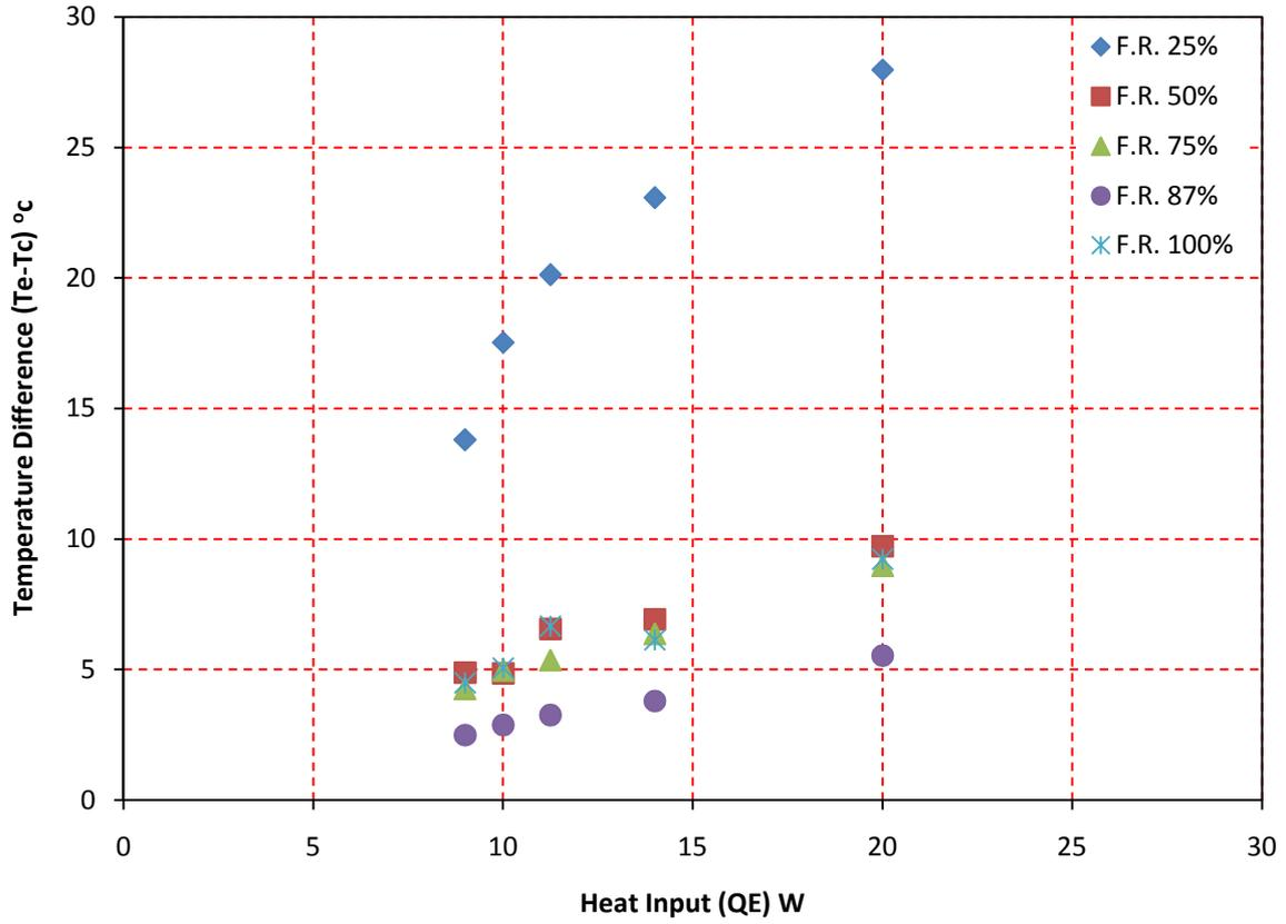
**Fig.7:** Temperature vs. heat input with variation of fill ratio for heat input
