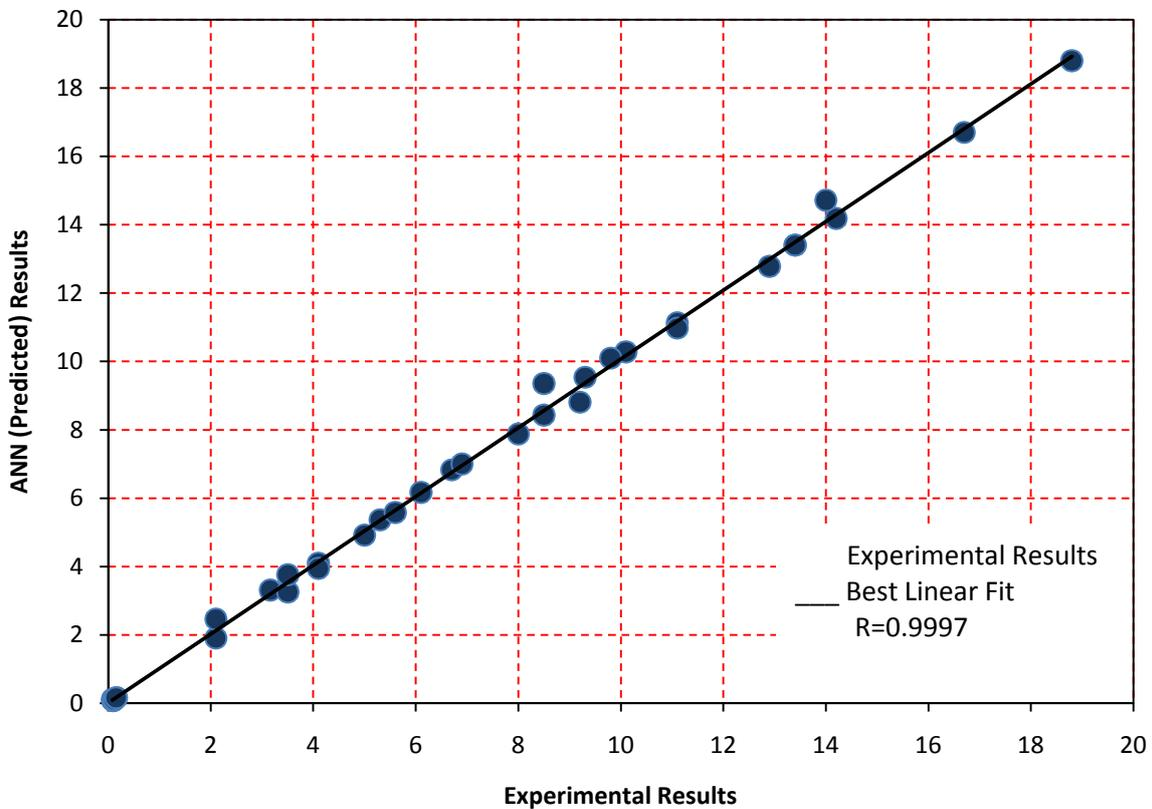
**Fig.10:** Comparison between ANN results and experimental results of heat transfer rate ( $Q_e$ ) using Resilient backpropagation algorithm
