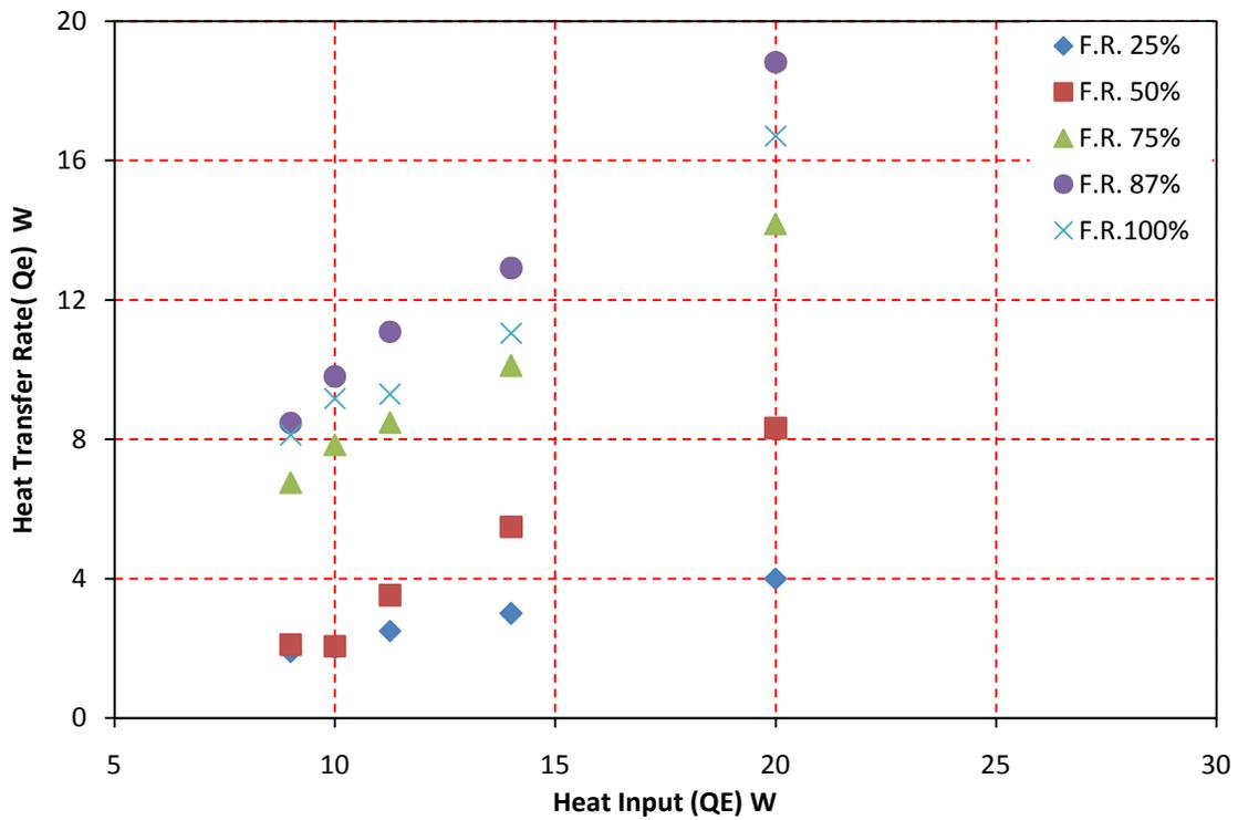
**Fig.8:** Heat transfer rate with heat input for different working fluid Fill ratio.
