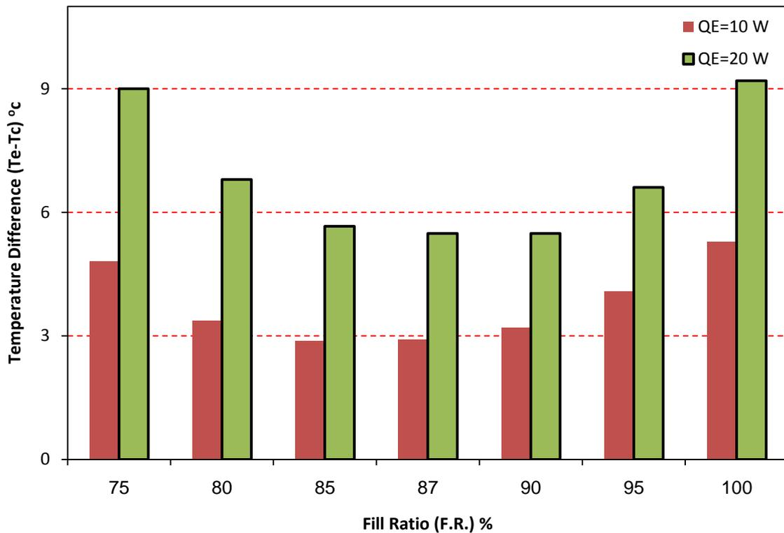
**Fig.12:** ANN predicated results of temperature difference between evaporator and condenser ( $T_e-T_c$ ) with varying fill ratio of working fluid at variation of heat input
