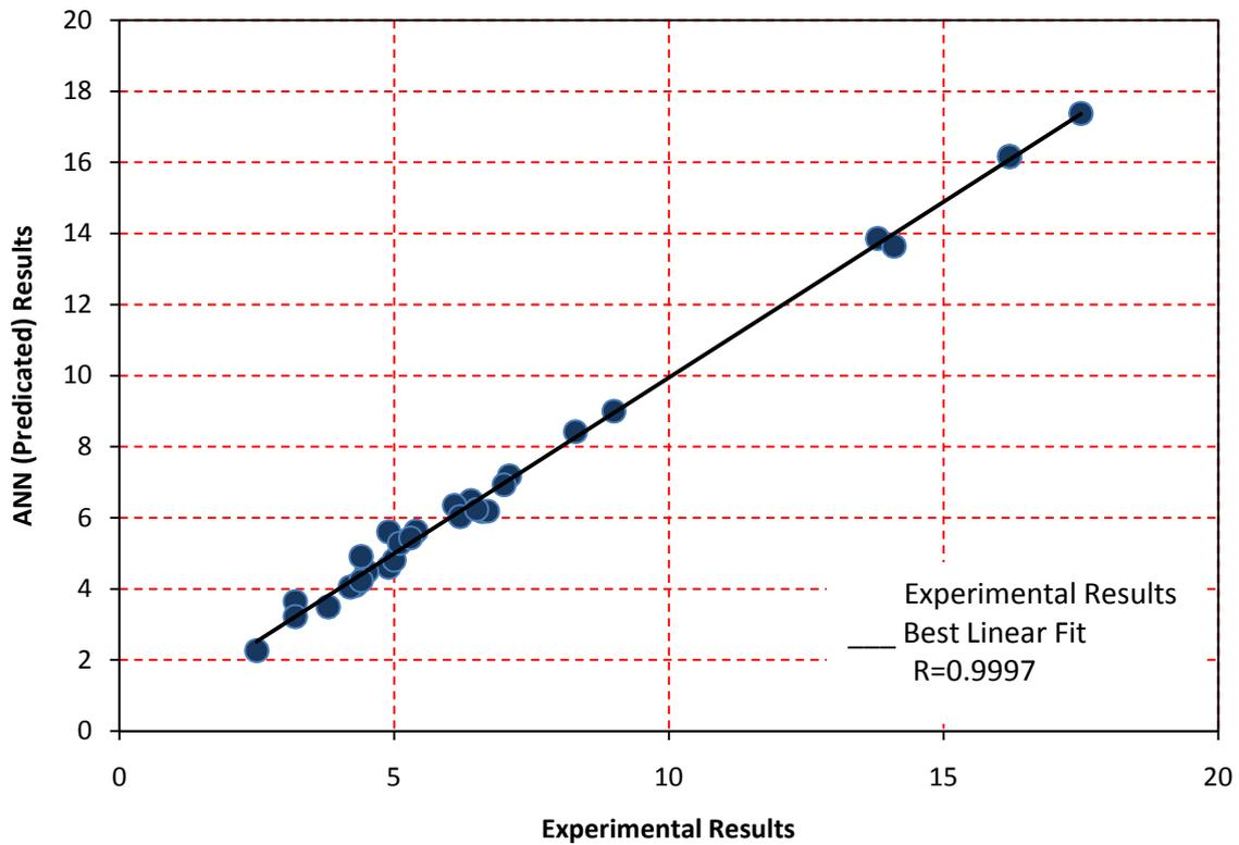
**Fig.11:** Comparison between ANN results and experimental results of temperature difference ( $T_e-T_c$ ) using Resilliantbackpropagation algorithm
