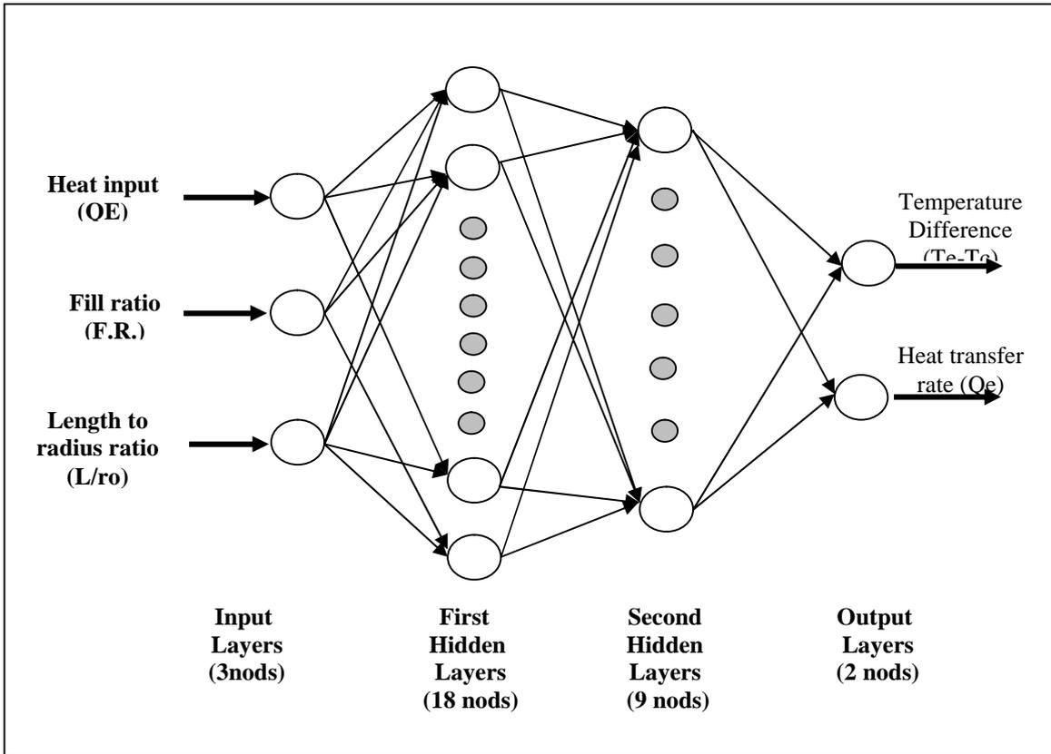
**Fig.9:** The architecture of neural network
