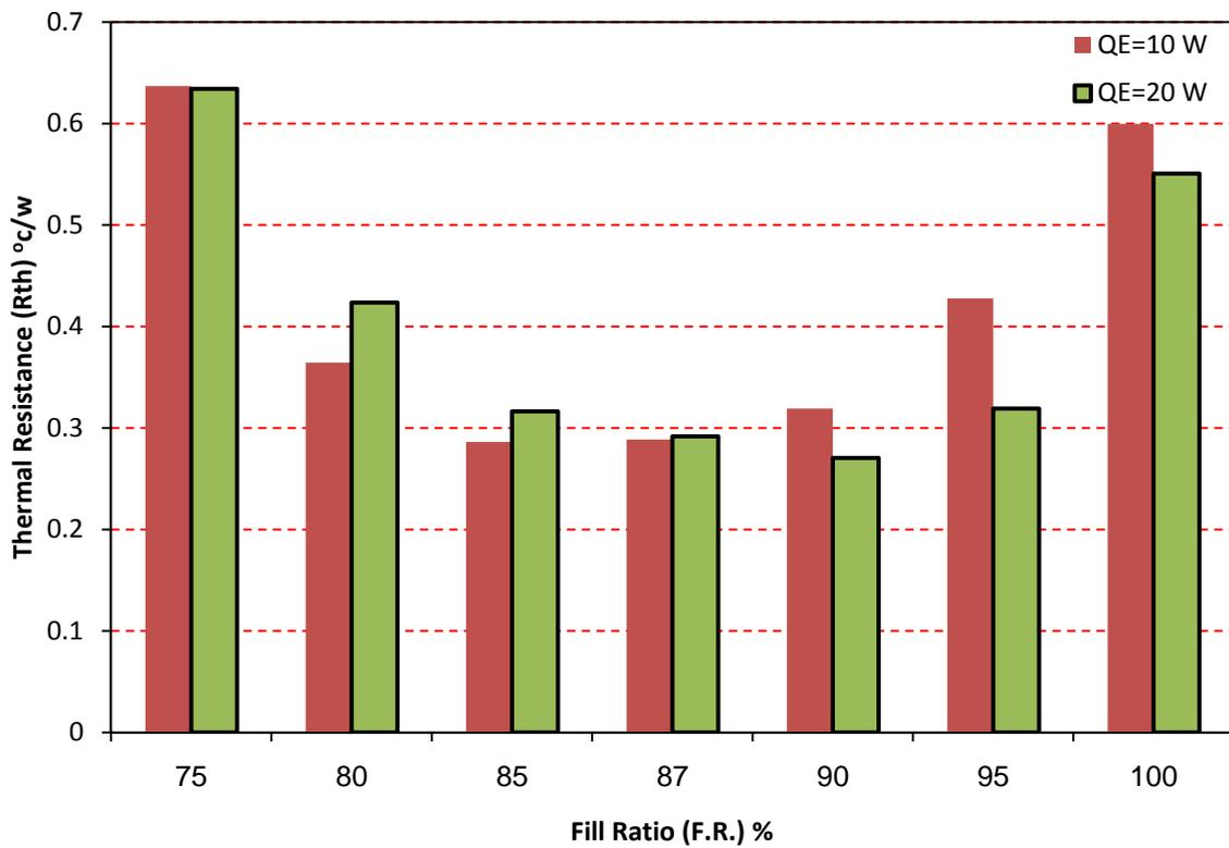
**Fig.14:** ANN predicated results of thermal resistance with varying fill ratio of working fluid at variation heat input
