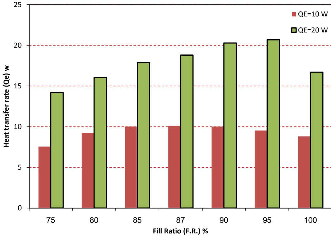
**Fig.13:** ANN predicated results of heat transfer rate with varying fill ratio of working fluid at variation heat input
