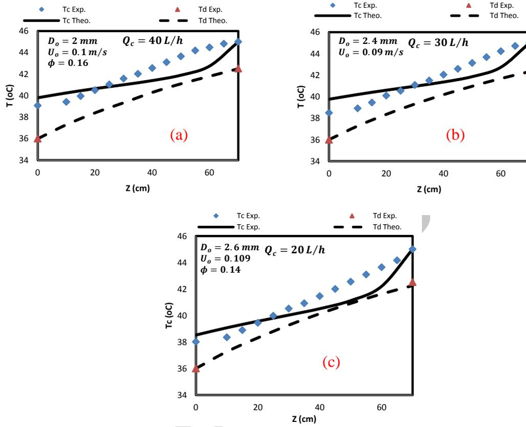
Figure 5: The temperature distribution of both the continuous and dispersed phases along the direct contact heat exchanger height for  $Q_d = 10 \text{ L/h}$  and  $D_{nz} = 1.25 \text{ mm}$  for a)  $Q_c = 40 \text{ L/h}$  b)  $Q_c = 30 \text{ L/h}$  and c)  $Q_c = 20 \text{ L/h}$
