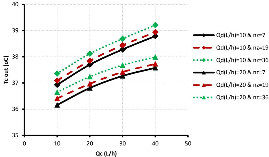
Figure 6: The effect of the sparger configuration on the continuous phase outlet temperature for two different dispersed phase flow rates and three different nozzles number with constant nozzle diameter ( $D_z = 0.001\text{m}$ )
