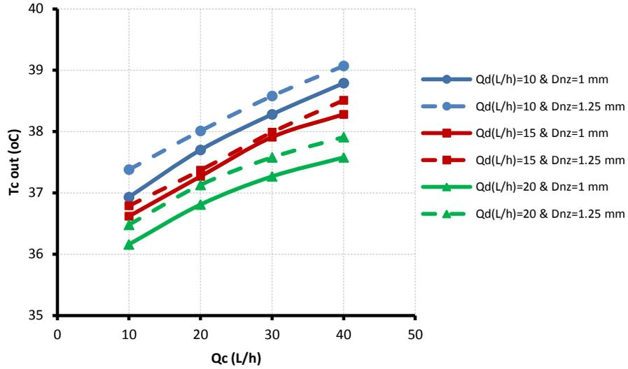
Figure 7: The effect of diameter of injection nozzle in the sparger on the continuous phase outlet temperature for two different dispersed phase flow rates. ( $n_z=7$ )
