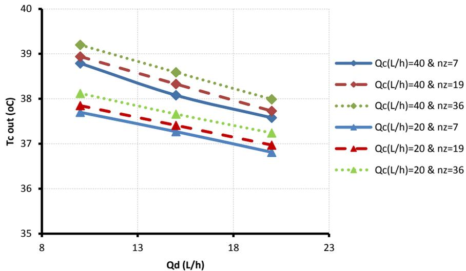
Figure 8: The variation of the outlet temperature of the continuous phase with dispersed phase flow rate for different continuous phase flow rate and sparger configuration.
