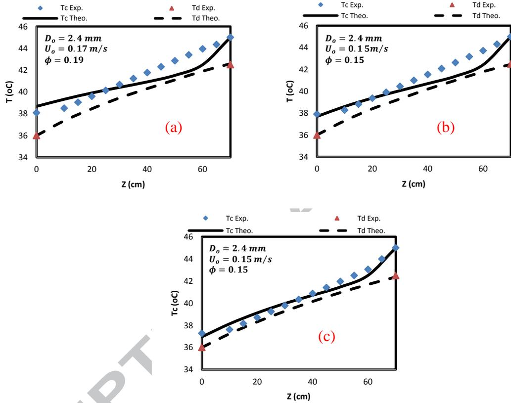
Figure 4: The temperature distribution of both the continuous and dispersed phases along the direct contact heat exchanger height for  $Q_d = 15 \text{ L/h}$  and  $D_{nz} = 1 \text{ mm}$  for a)  $Q_c = 40 \text{ L/h}$  b)  $Q_c = 30 \text{ L/h}$  and c)  $Q_c = 20 \text{ L/h}$
