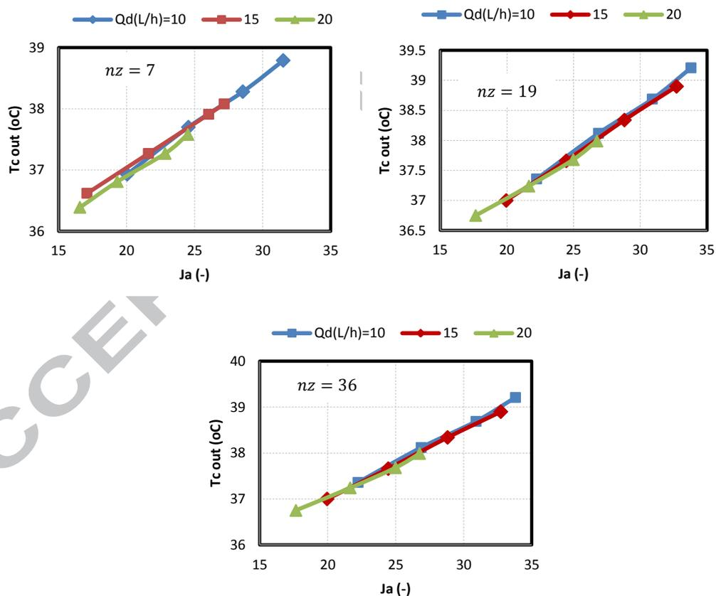
Figure 9: The effect of  $Ja$  on the outlet temperature of the continuous phase
