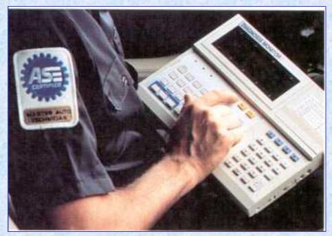
Using a diagnostic analyzer to find the source of engine performance problems
