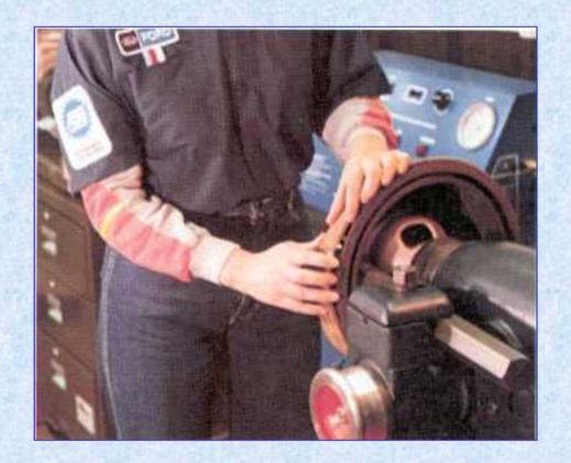
This technician is machining a brake drum
