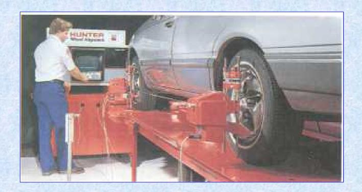
Specialized stall used when working on steering and suspension systems
