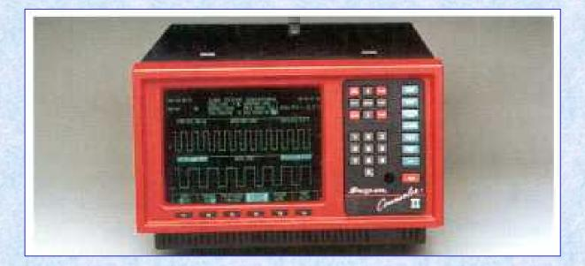
Dual trace scopes can read and show two separate waveforms simultaneously
