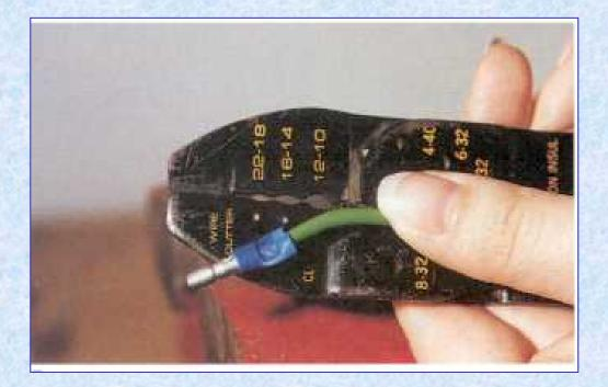
The crimping jaw was used to form this connector around the wire
