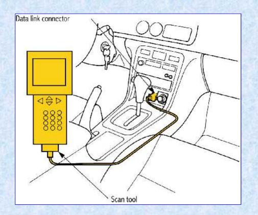
Power, ground, and communication lines are all provided in this data link connector
