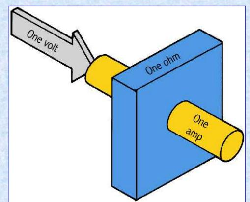
One volt can push one amp of current through one ohm of resistance
