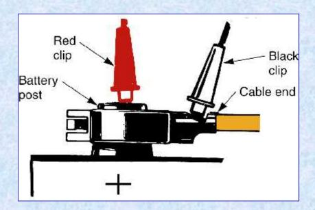
Checking the terminal for corrosion and high resistance
