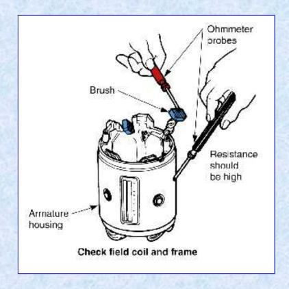
If resistance is low, replace the field winding
