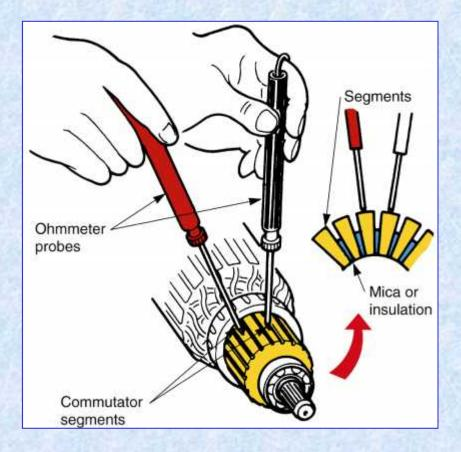
If an open exists between any commutator segment, replace the armature
