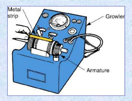
If the metal strip vibrates, replace the armature
