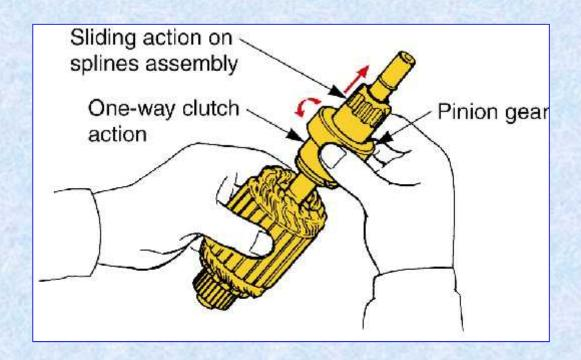
Check clutch action, as well as gear and bushing condition
