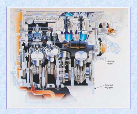
Remove the intake manifold to access the starting motor
