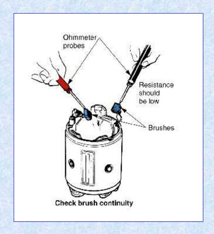
If resistance is high, replace the field winding
