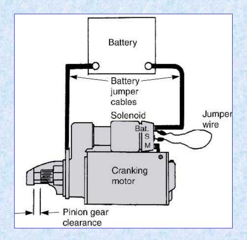
Connect a battery and check operation
