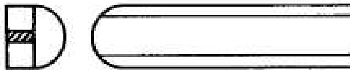
Spherical-surfaced LED and spherical-ended fiber
