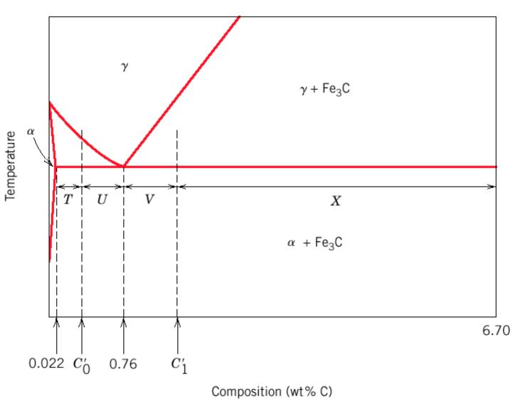
Fraction of  $\alpha$  phase is determined by application of the lever rule across the entire ( $\alpha + Fe_3C$ ) phase field:
