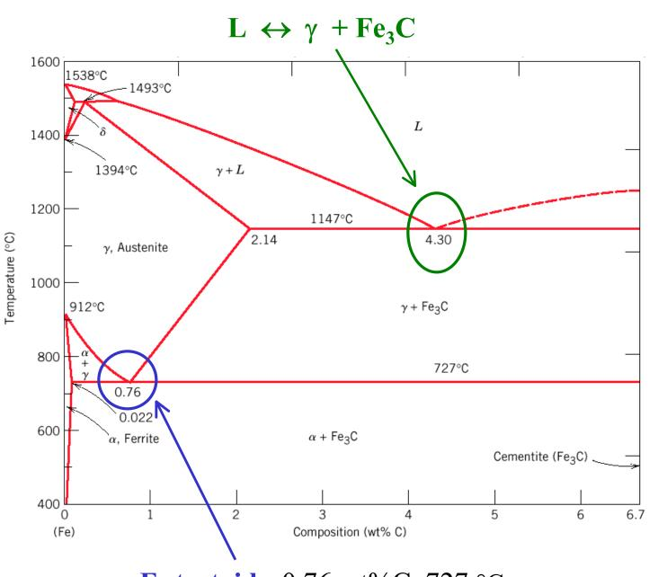
Eutectoid: 0.76 wt%C, 727 °C  $\gamma(0.76 \text{ wt\% C}) \leftrightarrow \alpha (0.022 \text{ wt\% C}) + \text{Fe}_3\text{C}$
