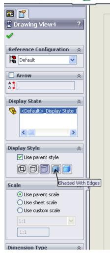
Click on the ISOMETRIC view, then choose SHADED WITH EDGES under DISPLAY STYLE on the left. In drawings, we always shade in the ISOMETRIC view
