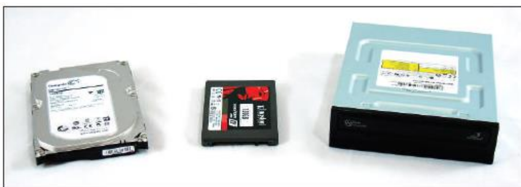
Figure (7) Two types of hard drives (larger magnetic drive and smaller solid-state drive) and a DVD drive
