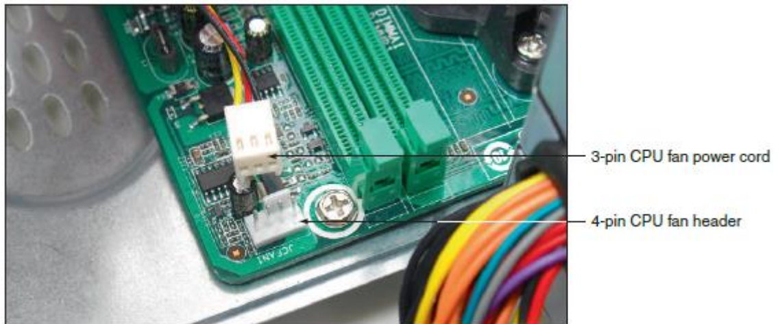
Figure (3) A cooler fan gets its power from a 4-pin PWM header on the motherboard
