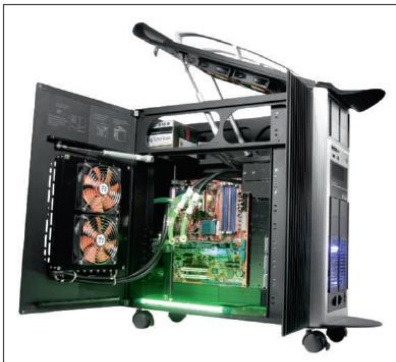
Figure (8) A liquid cooling system pumps liquid outside and away from components where fans can then cool the liquid
