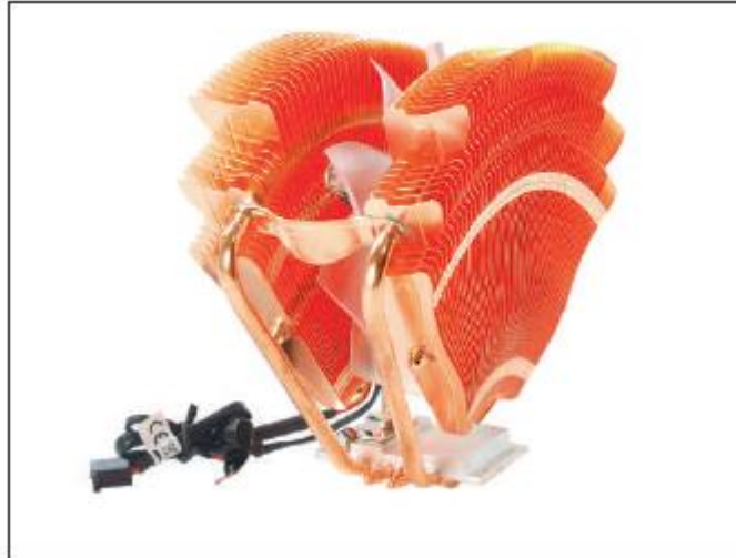
Figure (2) The Thermaltake V1 copper cooler fits Intel LGA1366 and LGA775 and AMD AM2 and AM2+ sockets
