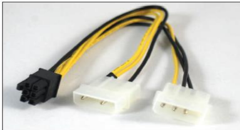
Figure (10) This adapter converts two Molex cables to a single 12 V 6-pin PCIe connector
