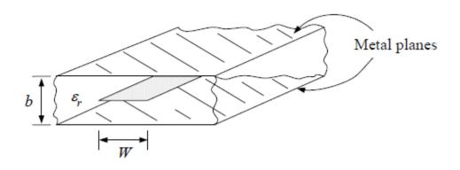
A stripline is a planar type transmission line which is well suited for microwave integrated circuitry and photolithographic fabrication.
