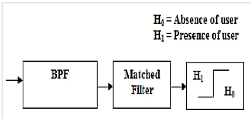
**Fig.2.15:** Matched filter Block diagram [9].
