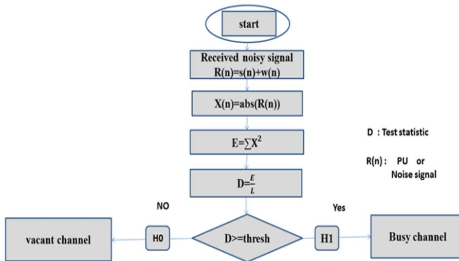
**Fig.2.14:** Simple Flow chart of the Energy Detection[3].
