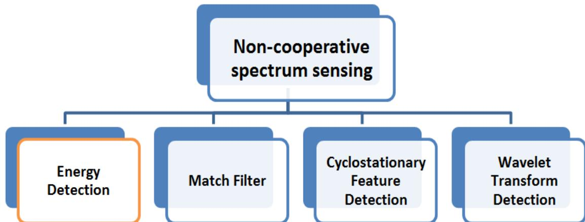
**Fig. 2.11:** Classification of non-cooperative spectrum sensing[7].
