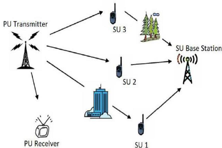
**Fig.2.17:** Centralized cooperative sensing[4].
