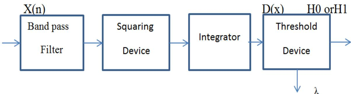
**Fig. 2.12:** Simple block diagram for Energy Detection method[2].
