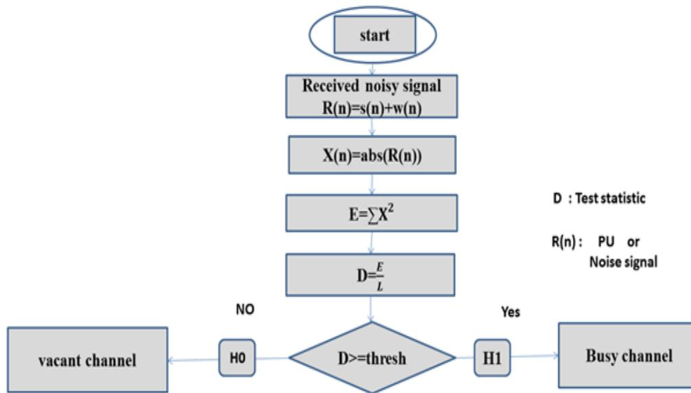
**Fig. 3.1:** Simple Flowchart of Energy Detection.
