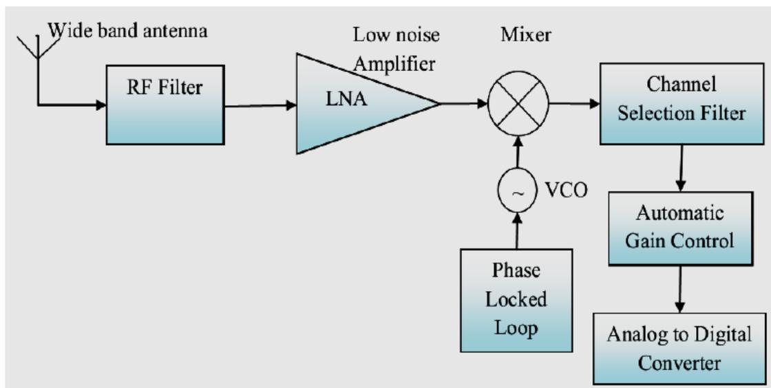
**Fig.2.5b:** Radio front-end [22]
