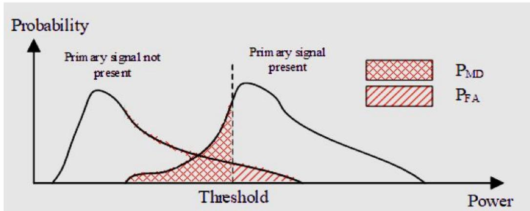
**Fig. 2.13:** Threshold setting in Energy Detection[7].
