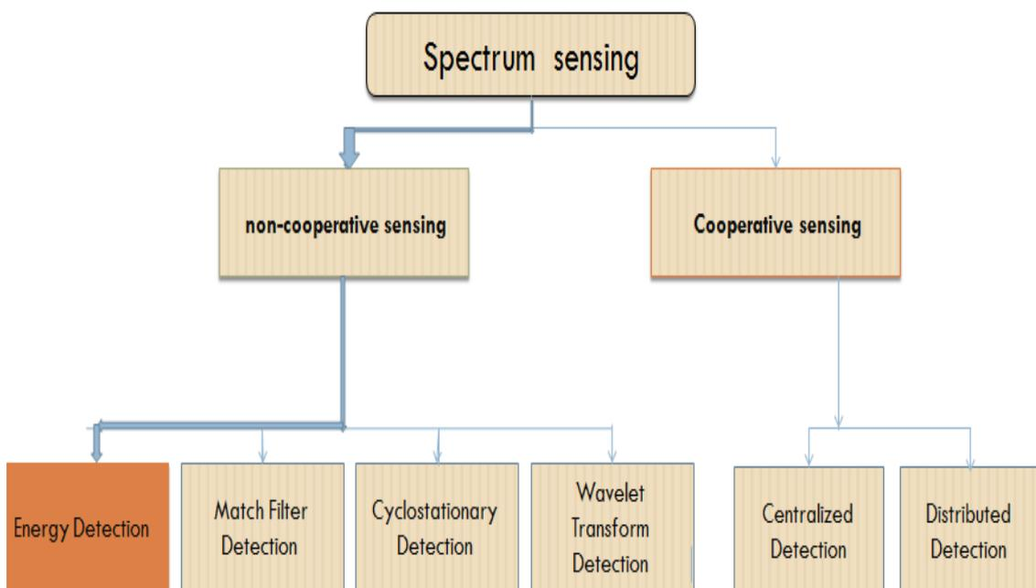
**Fig. 2.10:** Classifications of spectrum sensing [7].
