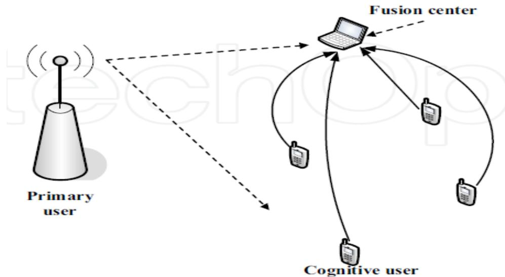
**Fig.2.18:** Scheme of partially cooperative network[11].
