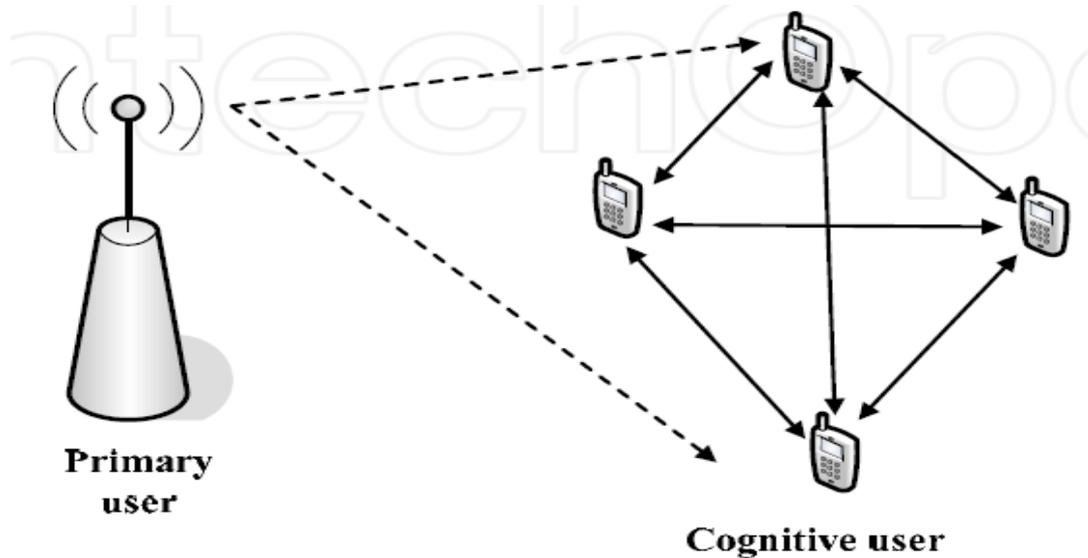
**Figure 2.20:** Scheme of distributed sensing[11].
