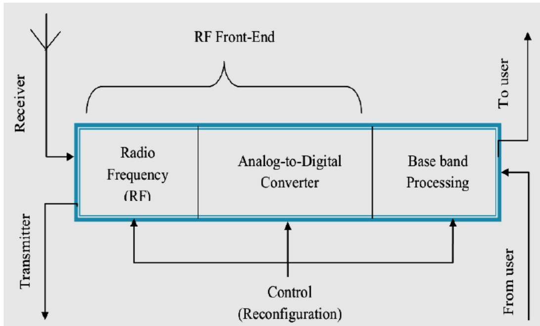
**Fig. 2.5a:** Cognitive Radio Transceiver[22].
