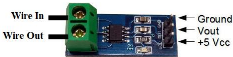
Fig. 3.5 ACS712-20A current sensor [45]
