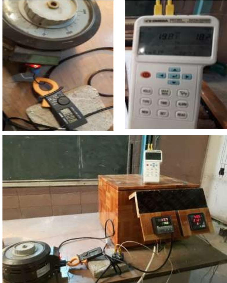
Figure 4.8 Connecting instruments to measuring the soil thermal conductivity
