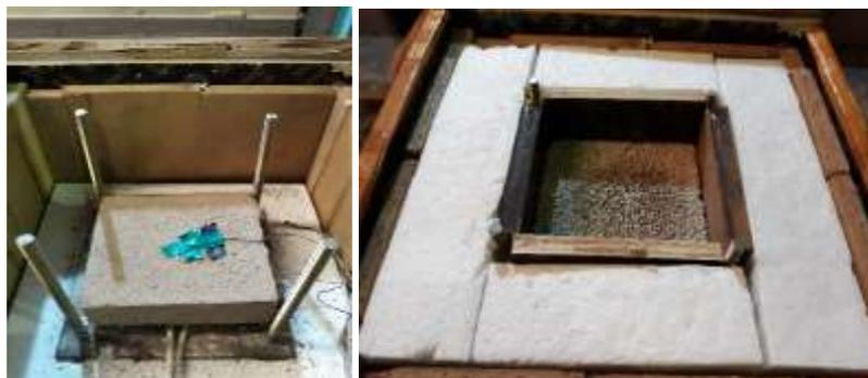
Figure 4.7 Placing thermostable and insulations
