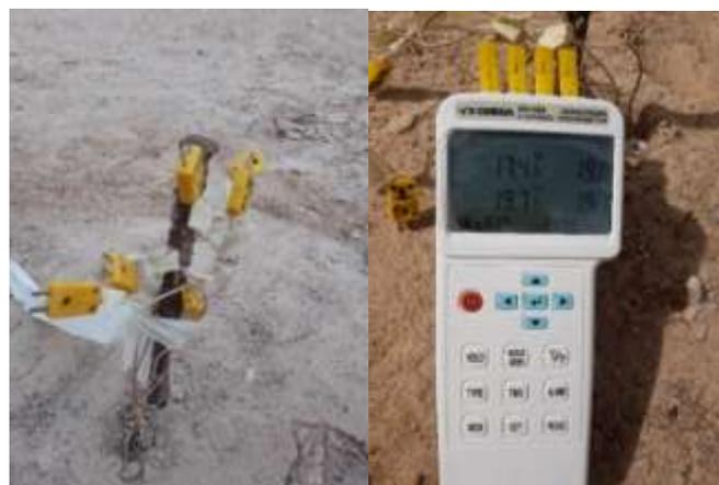
Figure 4.22: Data logger for Soil temperature gradient.
