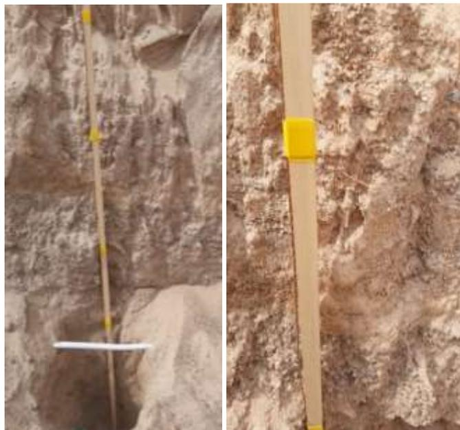
Figure 4.10 Setting the thermocouples to measuring the soil temperature gradient.
