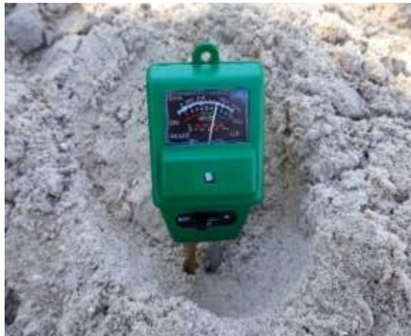
Figure 4.5: measuring the moisture content in the burying site.
