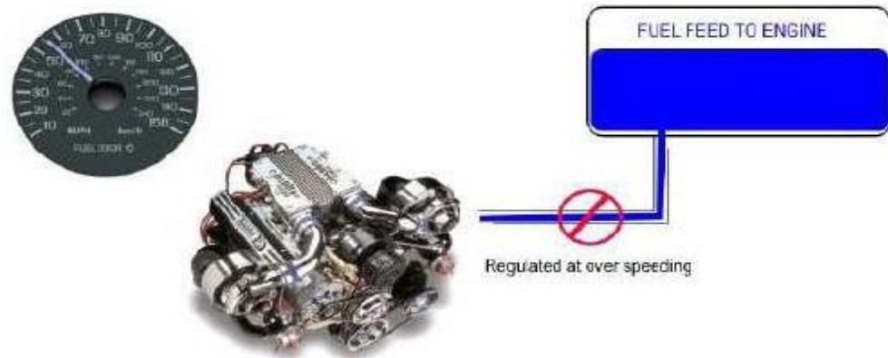
Fig.3.4: Description of the function of the road speed Limiter [44]
