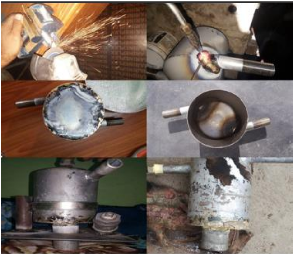
Figure 3.15: Steps of Manufacturing a Tangential Swirl Burner at Nozzle Diameter 5cm
