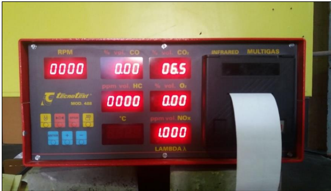
Figure 3.23: Gas Analysis Unit T156D
