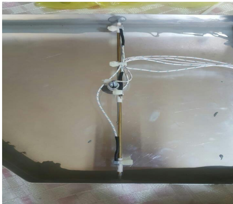
Figure 3. 15 Installing method of thermocouples inside water and paraffin wax tanks
