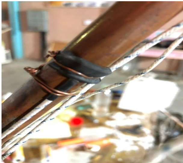
Thermocouple on the heat pipe surface
