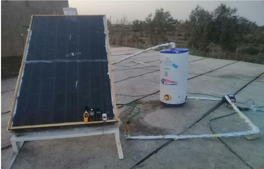
Fig. 4.1: Photo for DPSC system with measurment devices.
