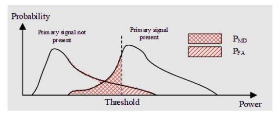
Fig. 2.13: Threshold setting in Energy Detection[7].
