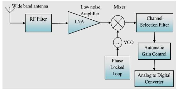
Fig.2.5b: Radio front-end [22]
