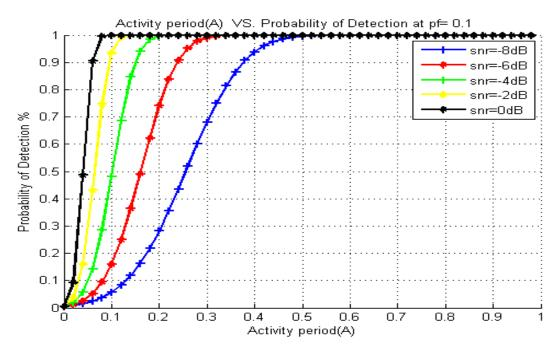
**Fig. 4.2:** Probability of Detection by varying (A) at different values of SNR PF = 0.1, L= 2000.
