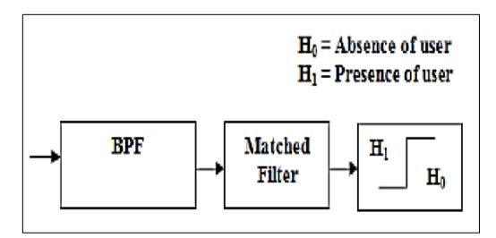
Fig.2.15: Matched filter Block diagram [9].
