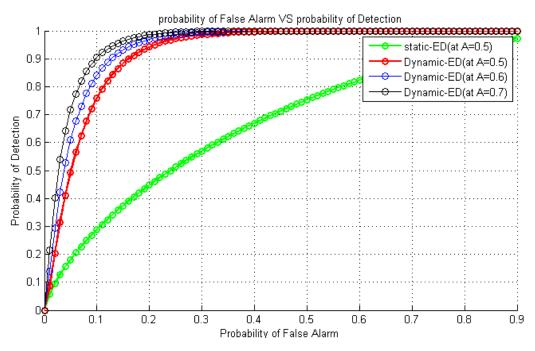
**Fig. 4.7:** Effect of dynamic threshold coefficient (d) and varying (*A*) values on ROC detection at L=1000 for CR systems.
