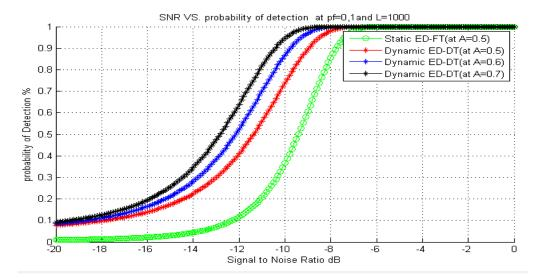
Fig. 4.10 Relation between SNR and probability of detection with different A L=1000 and PF =0.1
