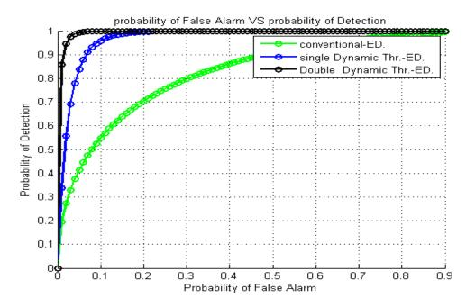
Fig. 4.6: ROC of fixed and dynamic threshold CR detection for d = 1.03 and L= 1000.
