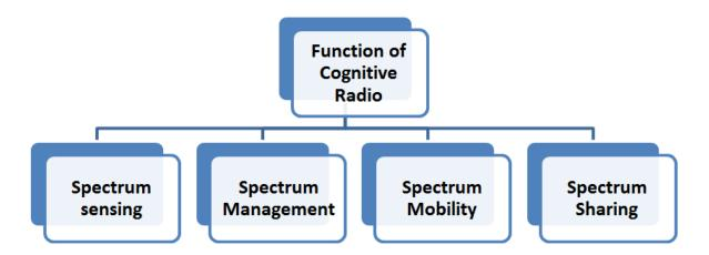
Fig 2.7: Simple scheme for the functions of CR [7].
