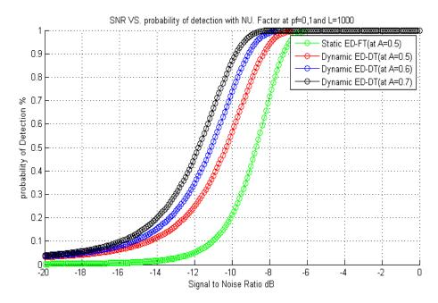
Fig. 4.14 Effect of Noise Uncertainty factor (NU) and relation between SNR and PD with different A at message L=1000 and PF =0.1.
