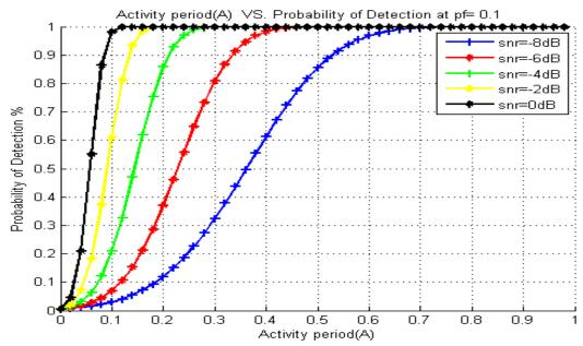
**Fig. 4.1:** Probability of Detection by varying (A) at different values of SNR PF=0.1, L=1000.
