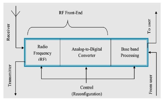
Fig. 2.5a: Cognitive Radio Transceiver[22].
