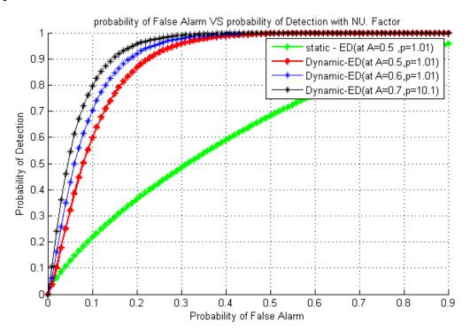
**Fig. 4.13:** Effect of Noise Uncertainty Factor (NU) with dynamic threshold and varying (*A*) values on ROC detection at L=1000 for CR system.
