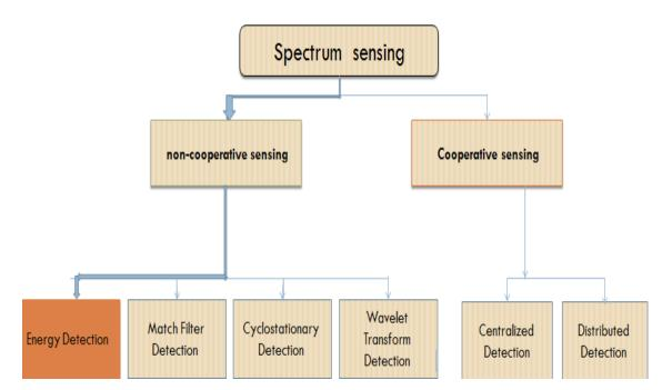
Fig. 2.10: Classifications of spectrum sensing [7].
