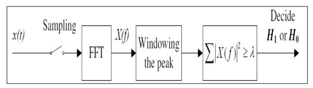
Fig. 2.16: Wavelet based Sensing Block diagram.
