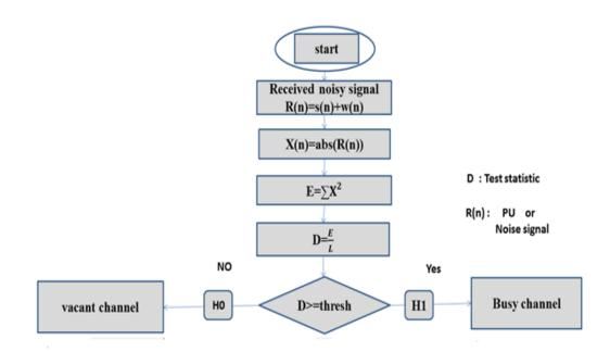
Fig. 3.1: Simple Flowchart of Energy Detection.
