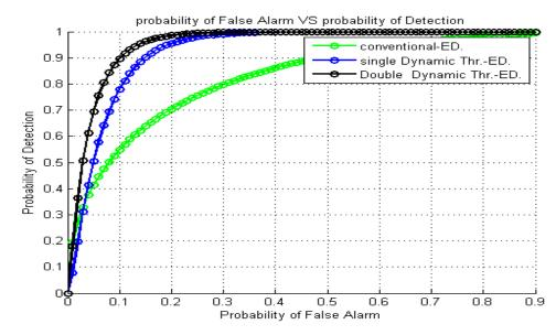
Fig. 4.5: ROC of fixed and dynamic threshold CR detection for d=1.01 and L=1000.
