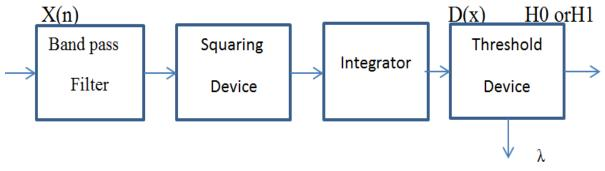
**Fig. 2.12:** Simple block diagram for Energy Detection method[2].
