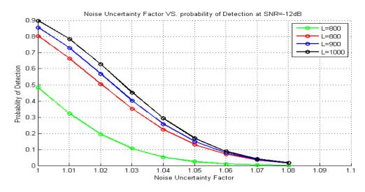
**Fig. 4.11:** Effect of Noise Uncertainty Factor on the Probability of Detection with varying Number of Samples.
