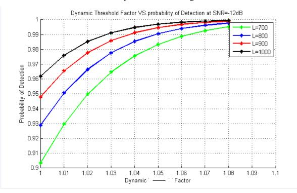
Fig. 4.3: Effect of Dynamic Factor on the PD with varying number of samples.
