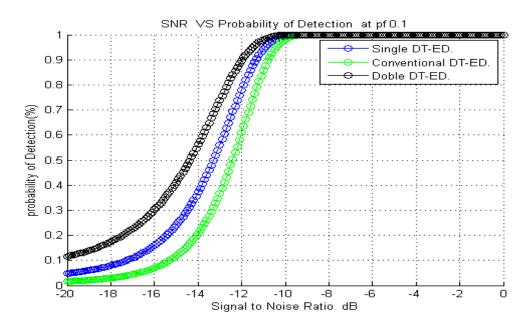
Fig. 4.9: Relation between SNR and PD (L=1000 at PF =0.1
