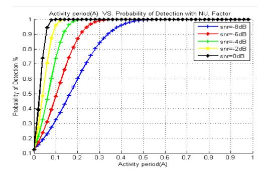
**Fig.4.12.** Effect of Noise Uncertainty coefficient (p) on the Probability of Detection with varying SNR values and L=1000.
