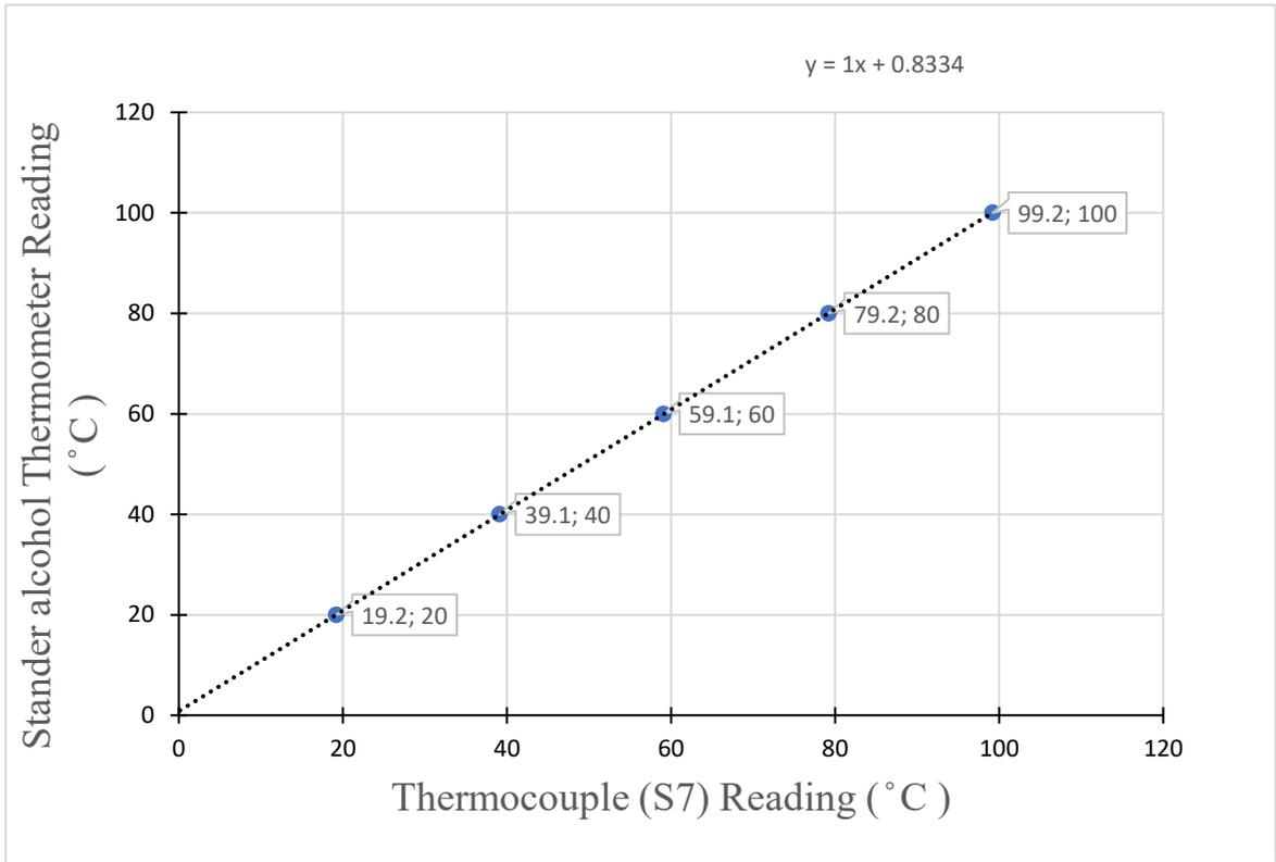
Figure A .7: Thermocouple (S7) calibration, ISS 2, basin water
