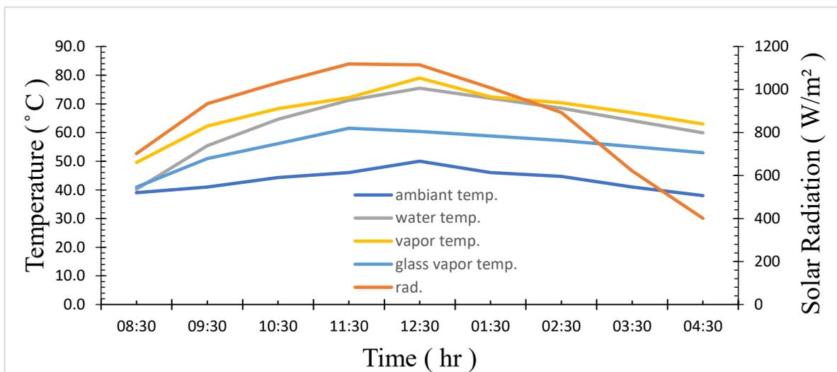
Figure 4.51: variation of temperature and solar radiation with measurement time for solar still with N shape water channel
