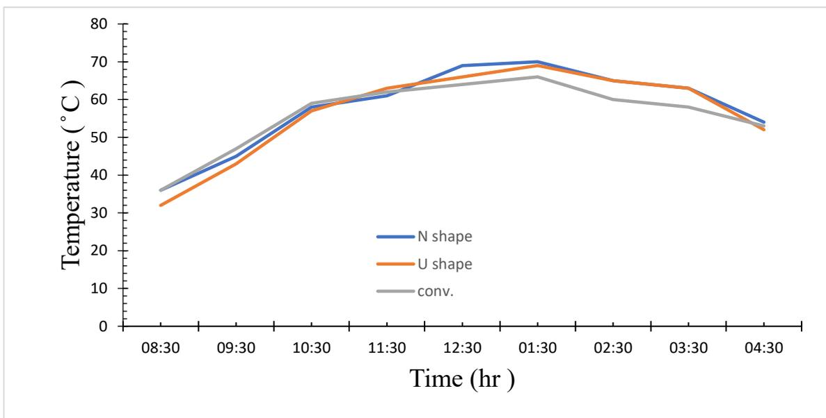
Figure 4.46: variation of basin water temperature with the time of the experiment
