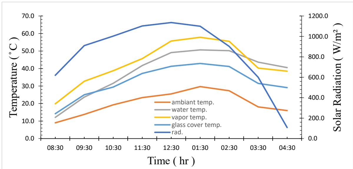
Figure 4.1: variation of temperature and solar radiation with measurement time for conventional solar still
