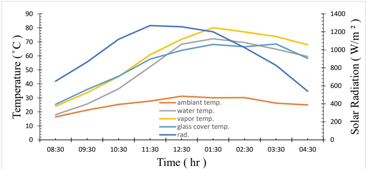
Figure 4.23: variation of temperature and solar radiation with measurement time for solar still with 25 \*25 grid size wick still
