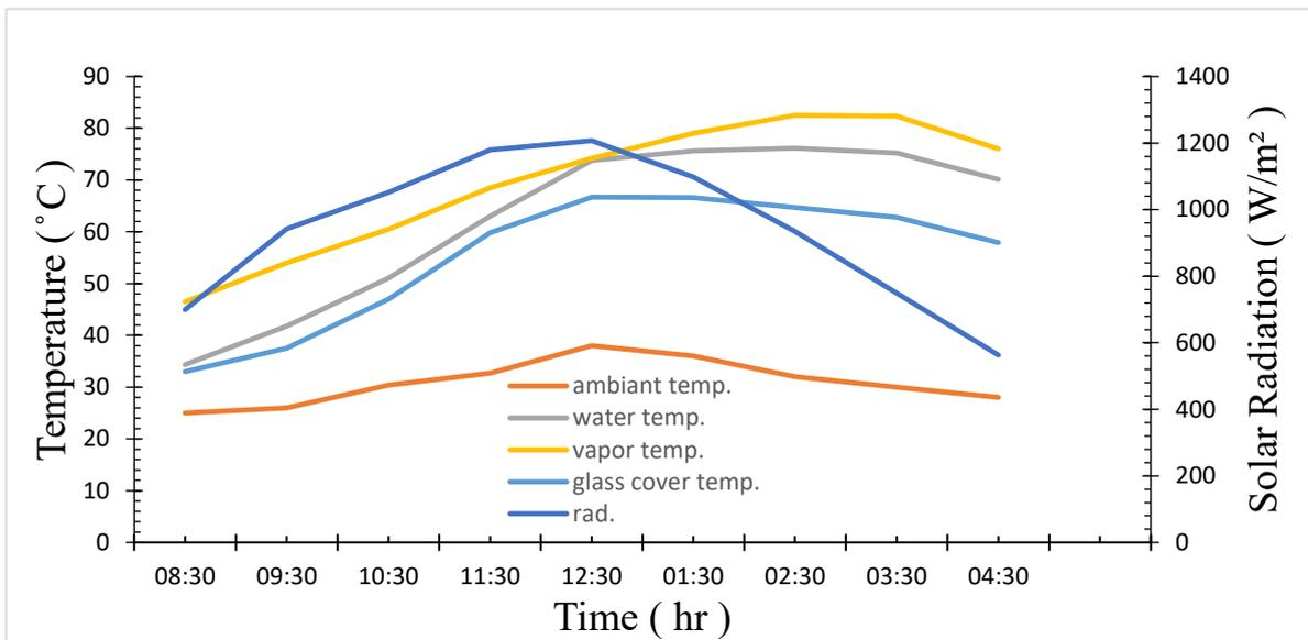
Figure 4.16: variation of temperature and solar radiation with measurement time for solar still with 15 mm diameter copper pipe
