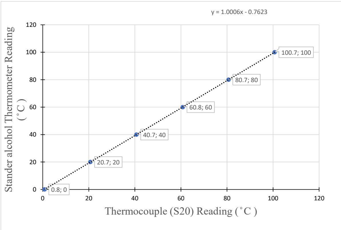
Figure A .20: Thermocouple (S20) calibration
