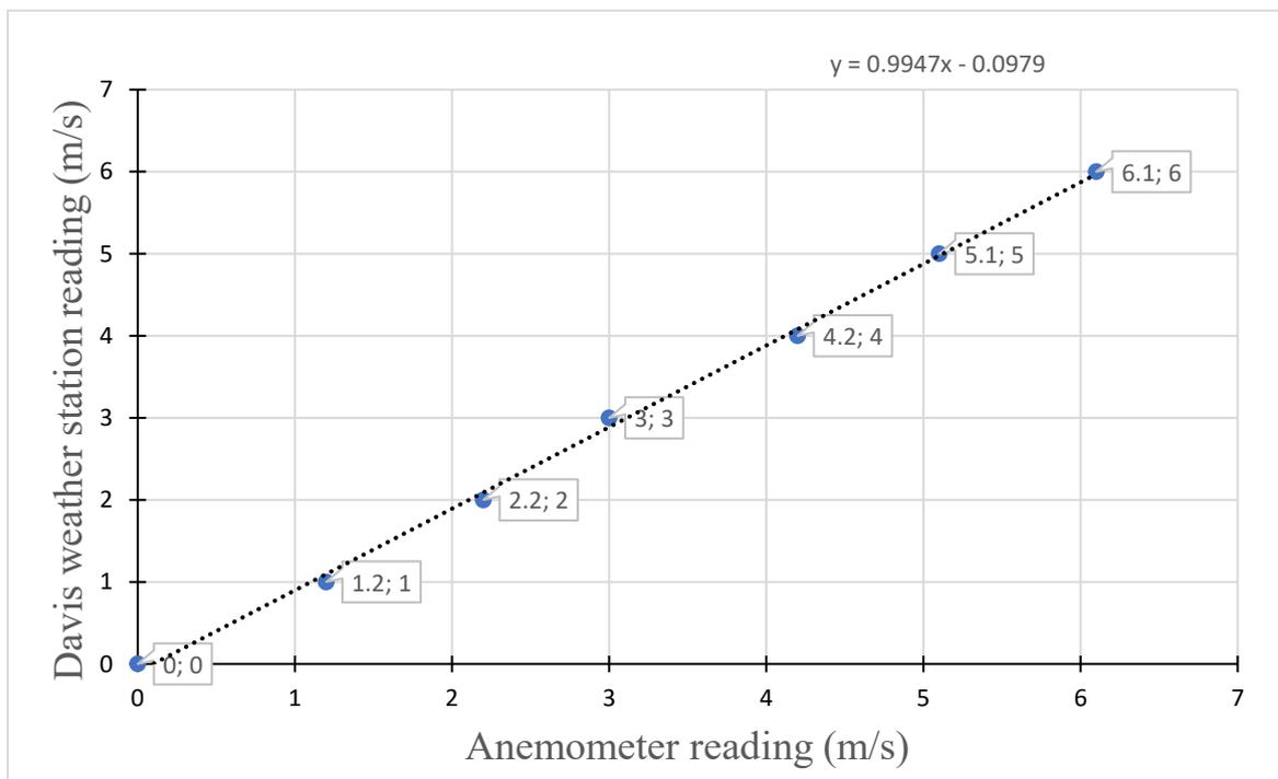
D.1 Anemometer calibration
