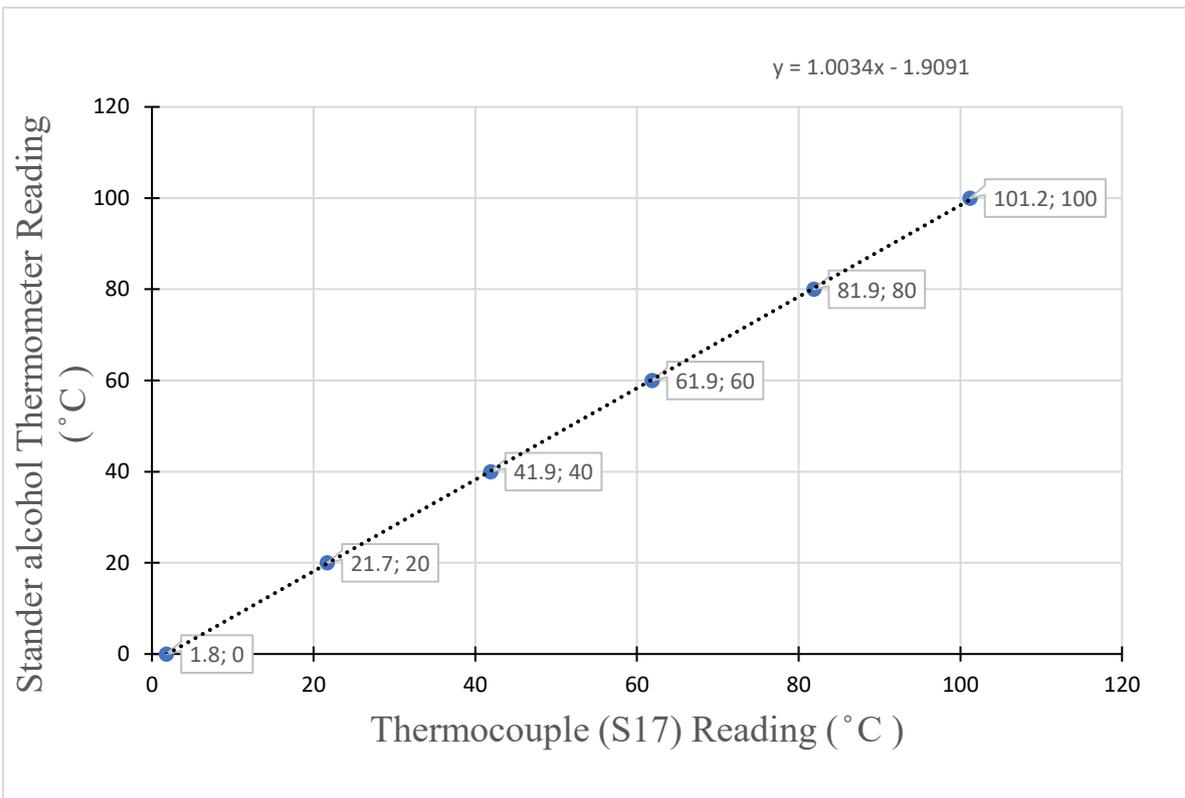
Figure A .17: Thermocouple (S17) calibration, CSS, glass cover
