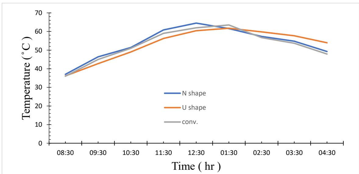
Figure 4.39: variation of basin water temperature with the time of the experiment
