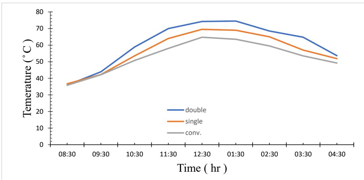
Figure 4.34 variation glass cover temperature with the time of the experiment
