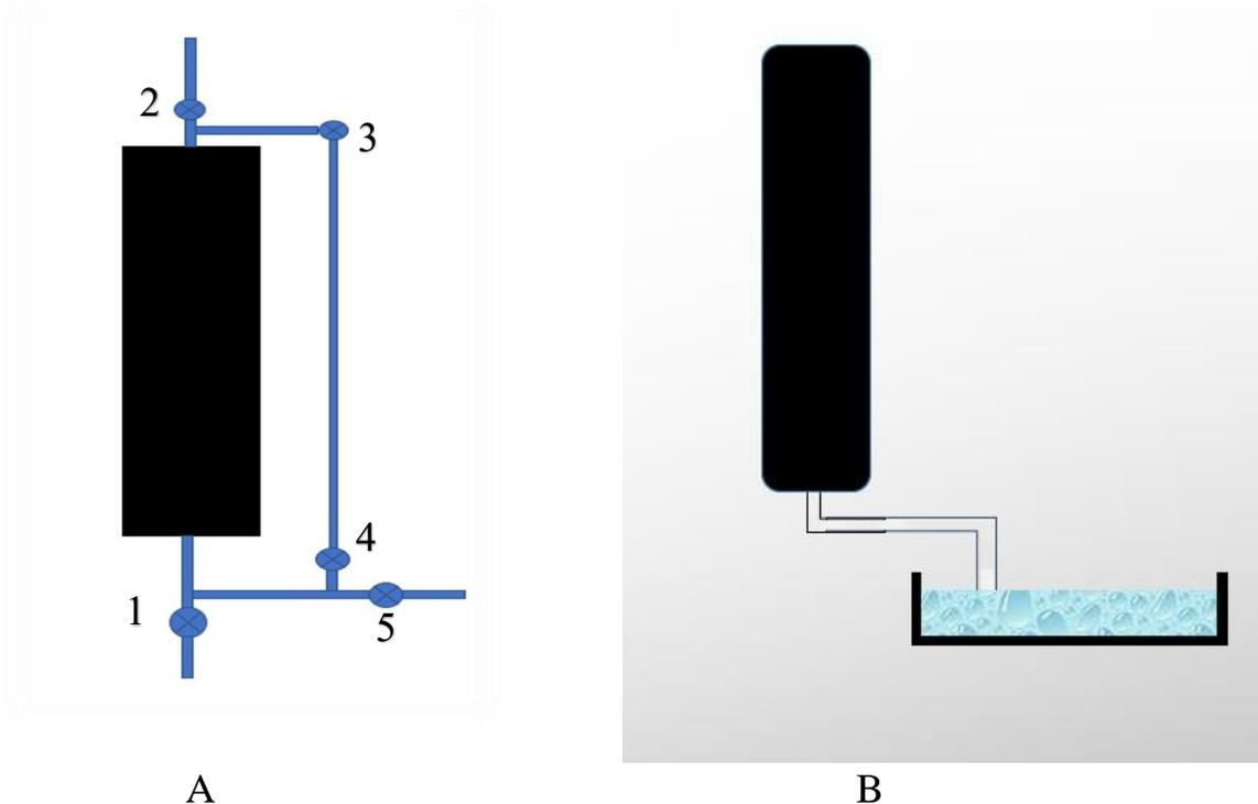
Figure 3.6 Schematic view of A: tank and control valves and B: tank feeding mechanism
