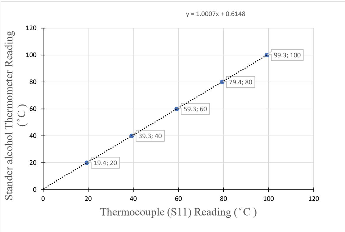
Figure A .11: Thermocouple (S11) calibration, ISS 2, glass cover
