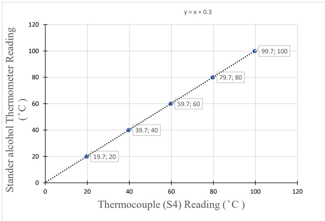
Figure A .4: Thermocouple (S4) calibration, ISS 1, vapor
