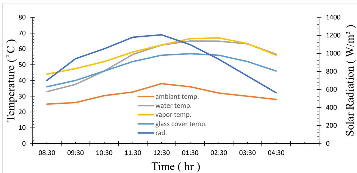
Figure 4.15: variation of temperature and solar radiation with measurement time for conventional solar still
