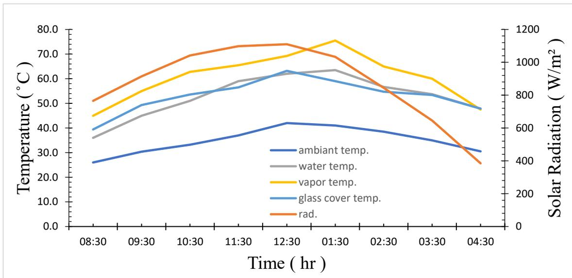
Figure 4.38: variation of temperature and solar radiation with measurement time for solar still with U shape water channel at 1 L/min.
