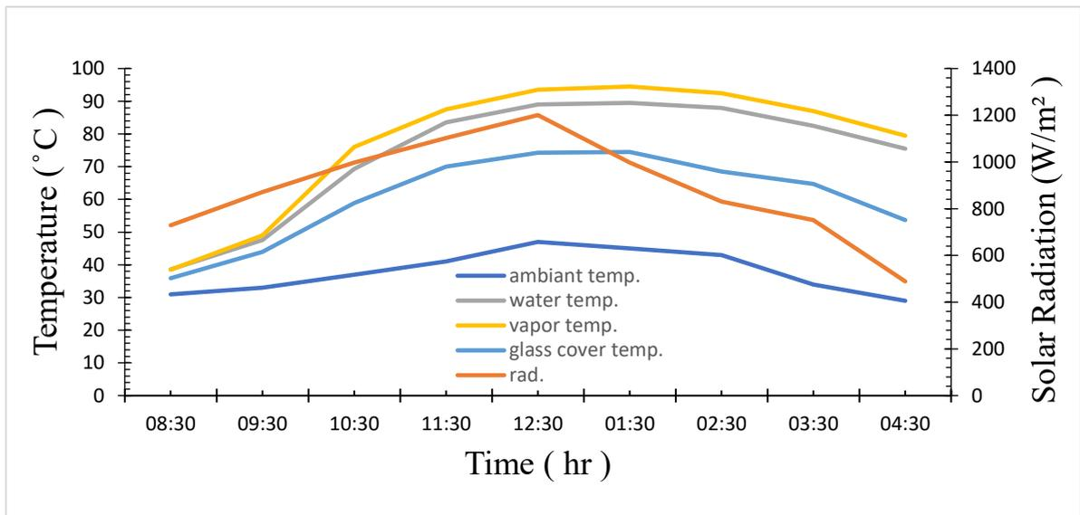
Figure 4.30: variation of temperature and solar radiation with measurement time for solar still with double wicks (25 \* 25 and 50 \* 50 grids size)
