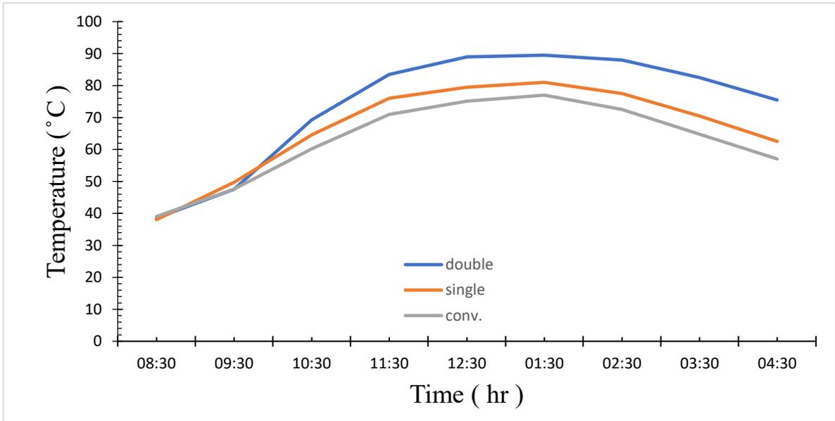
Figure 4.32 variation of basin water temperature with the time of the experiment
