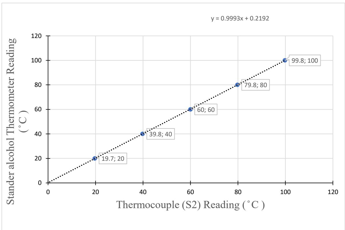
Figure A .2: Thermocouple (S2) calibration, ISS 1, water basin
