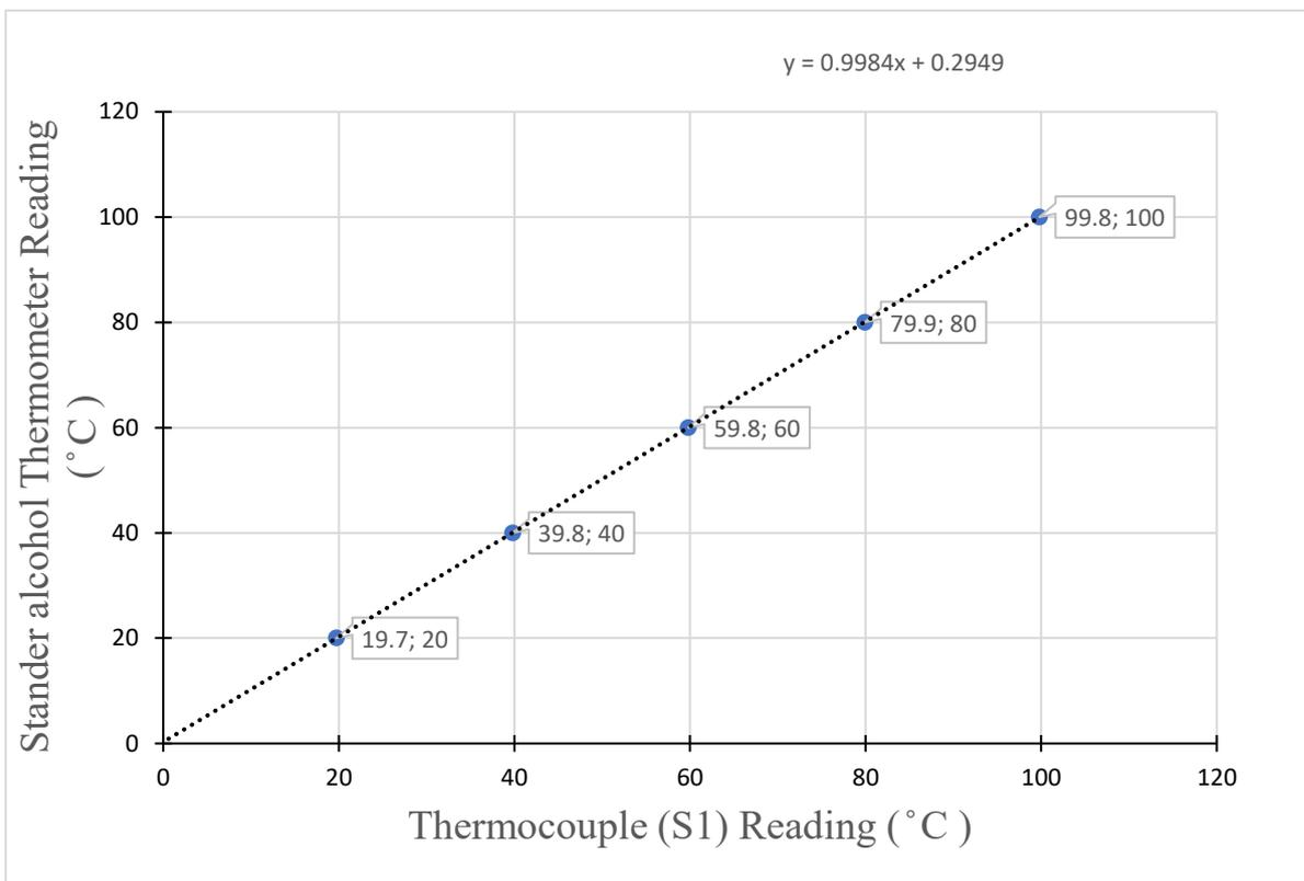
Figure A .1: Thermocouple (S1) calibration, ISS 1, water basin
