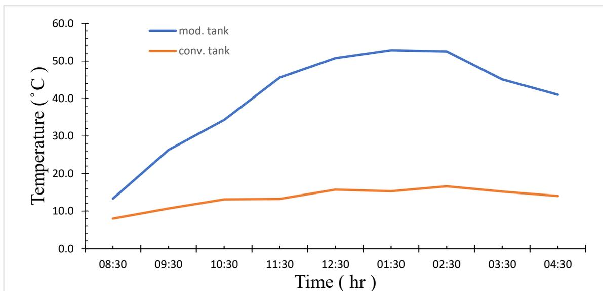
Figure 4.3: variation of input water temperature with the time of the experiment
