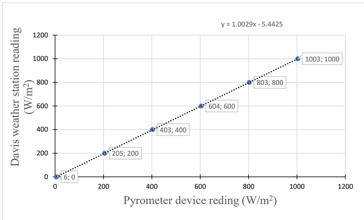
C.1 Pyranometer calibration
