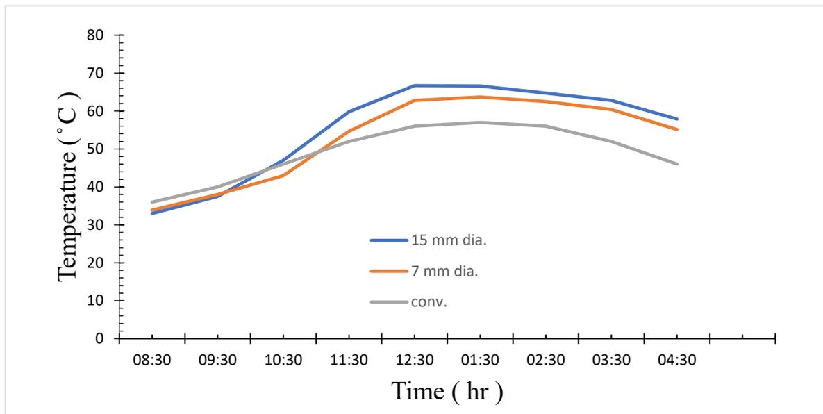
Figure 4.20: variation of basin water temperature with the time of the experiment
