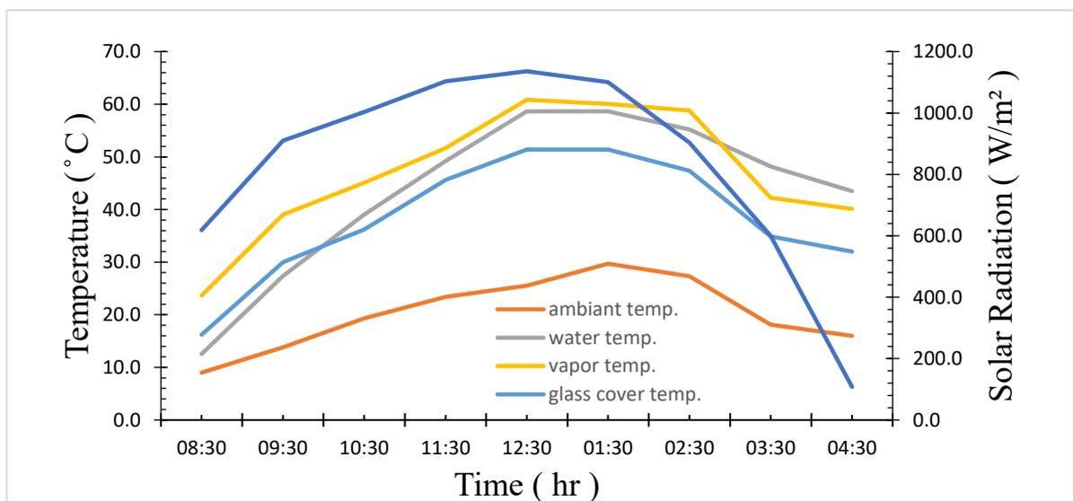
Figure 4.2: variation of temperature and solar radiation with measurement time for modified solar still
