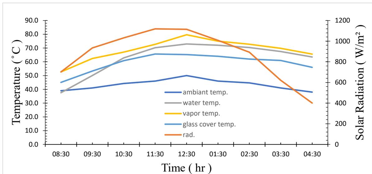
Figure 4.52: variation of temperature and solar radiation with measurement time for solar still with U shape water channel
