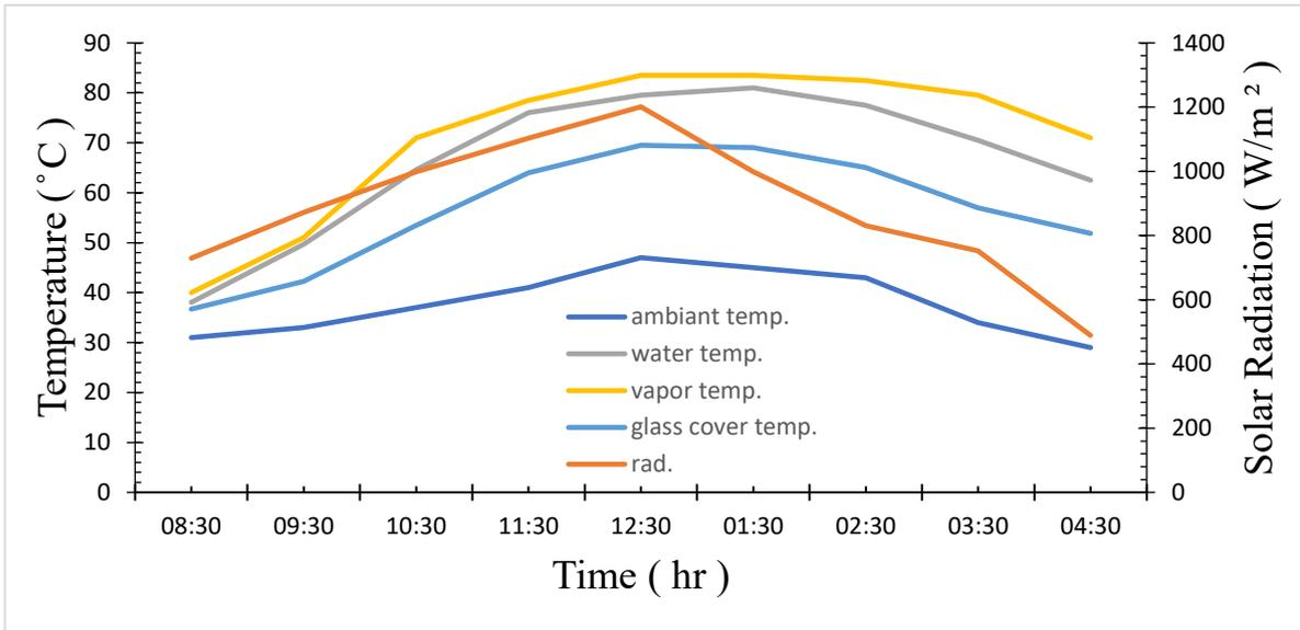
Figure 4.31: variation of temperature and solar radiation with measurement time for solar still with single wick (25 \*25 grid size)
