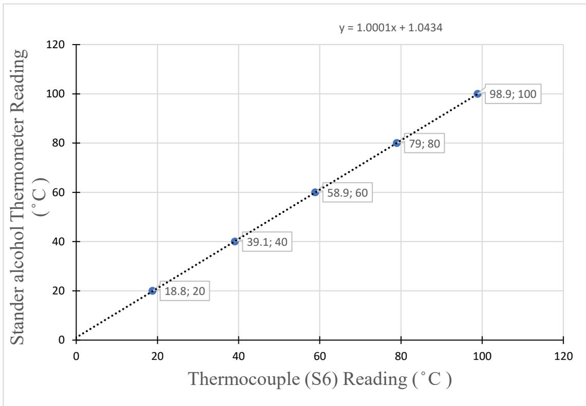
Figure A .6: Thermocouple (S6) calibration, ISS 1, glass cover
