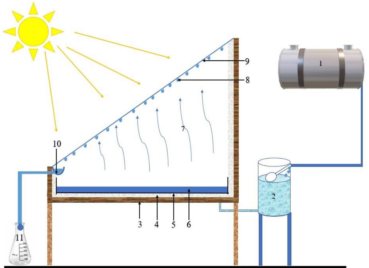
Figure 1.2 single slope solar still
