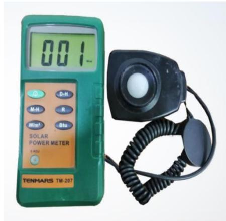
Figure 3.3 Solar radiation measuring device
