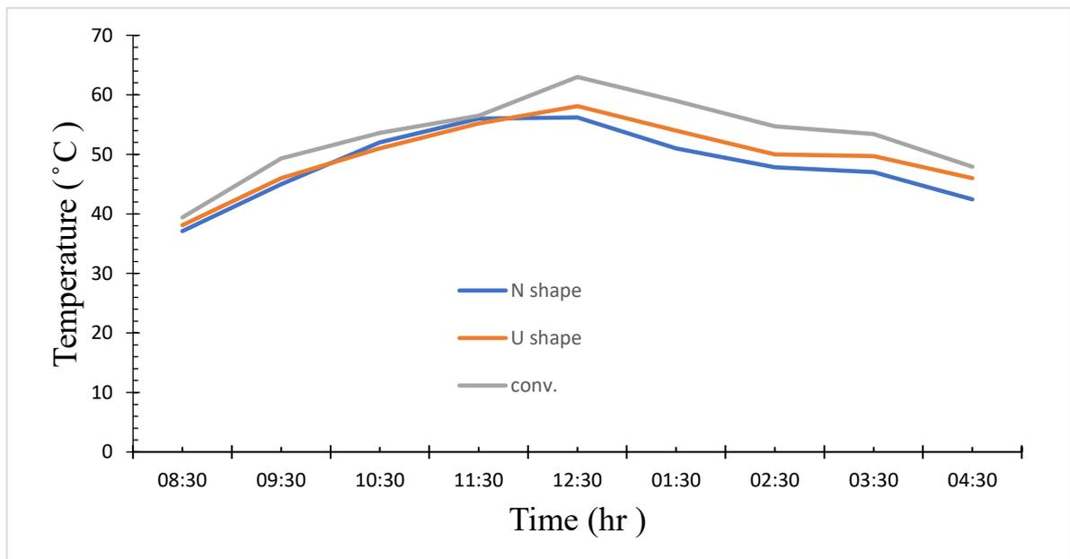
Figure 4.48: variation of glass cover temperature with the time of the experiment
