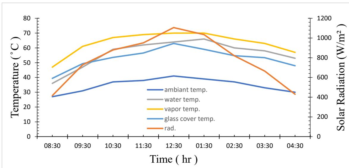
Figure 4.43: variation of temperature and solar radiation with measurement time for conventional solar still
