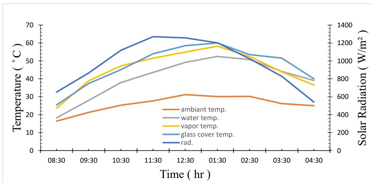
Figure 4.22: variation of temperature and solar radiation with measurement time for conventional solar still
