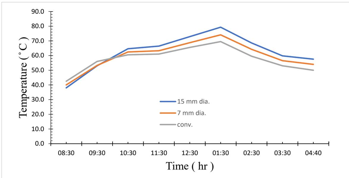
Figure 4.12: variation of vapor temperature with the time of the experiment
