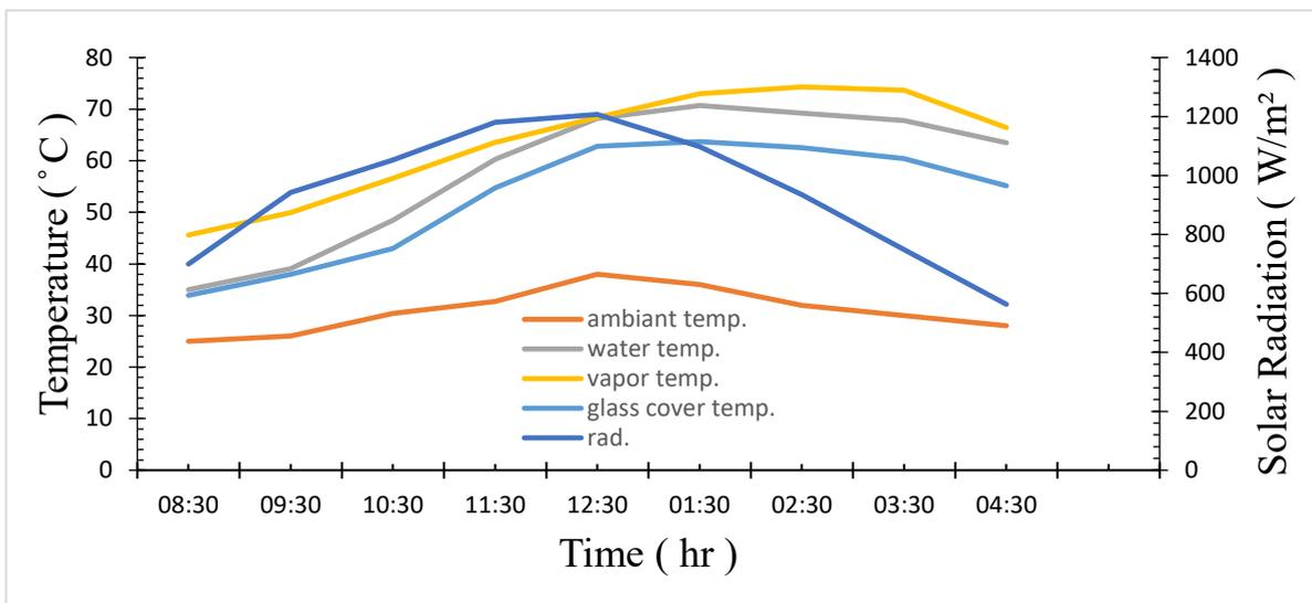
Figure 4.17: variation of temperature and solar radiation with measurement time for solar still with 7 mm diameter copper pipe
