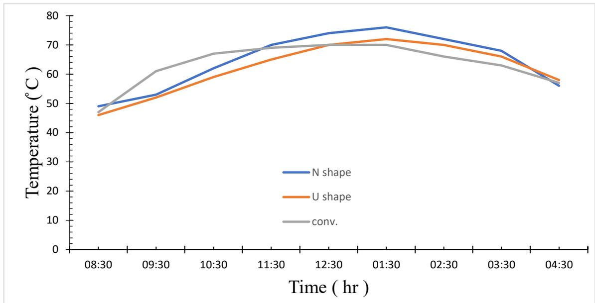
Figure 4.47: variation of vapor temperature with the time of the experiment
