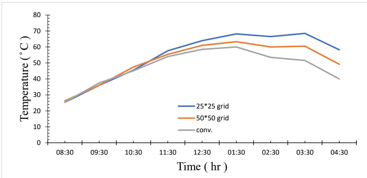
Figure 4.27 variation of glass cover temperature with the time of the experiment
