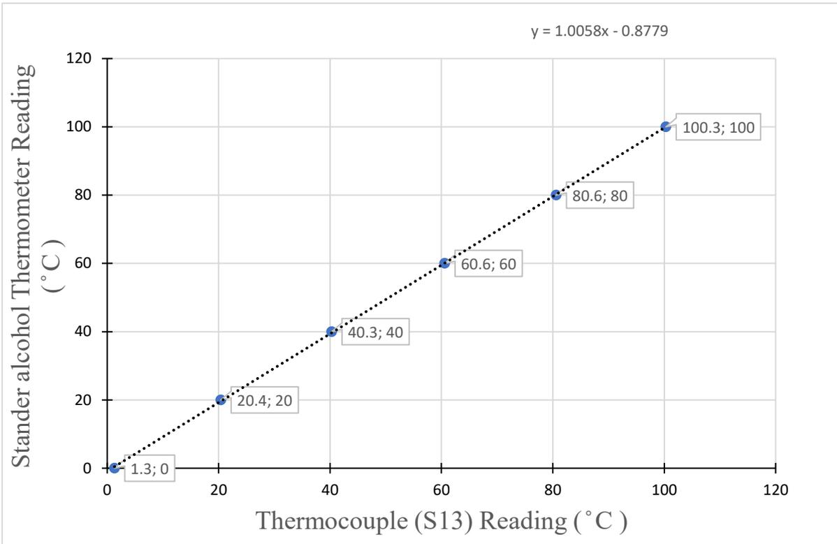
Figure A .13: Thermocouple (S13) calibration, CSS, basin water
