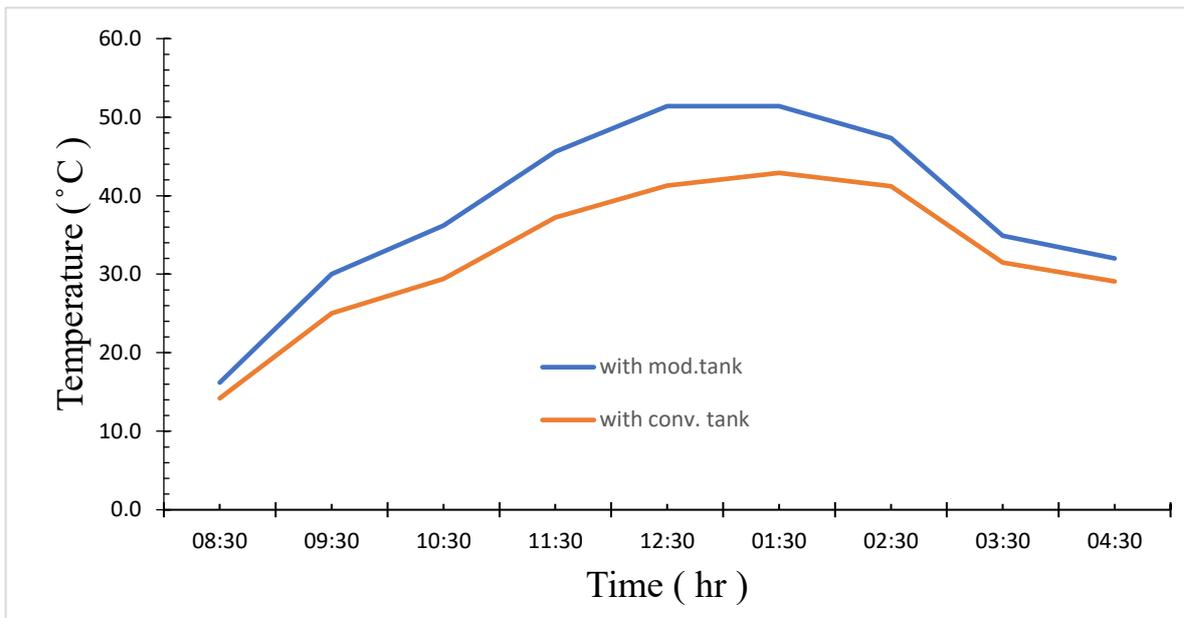
Figure 4.6 variation of glass cover temperature with the time of the experiment
