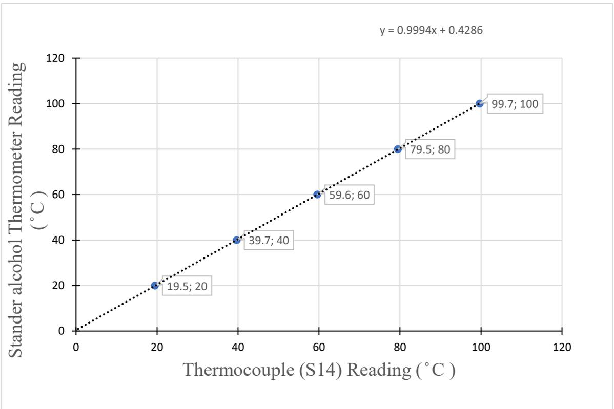
Figure A .14: Thermocouple (S14) calibration, CSS, basin water
