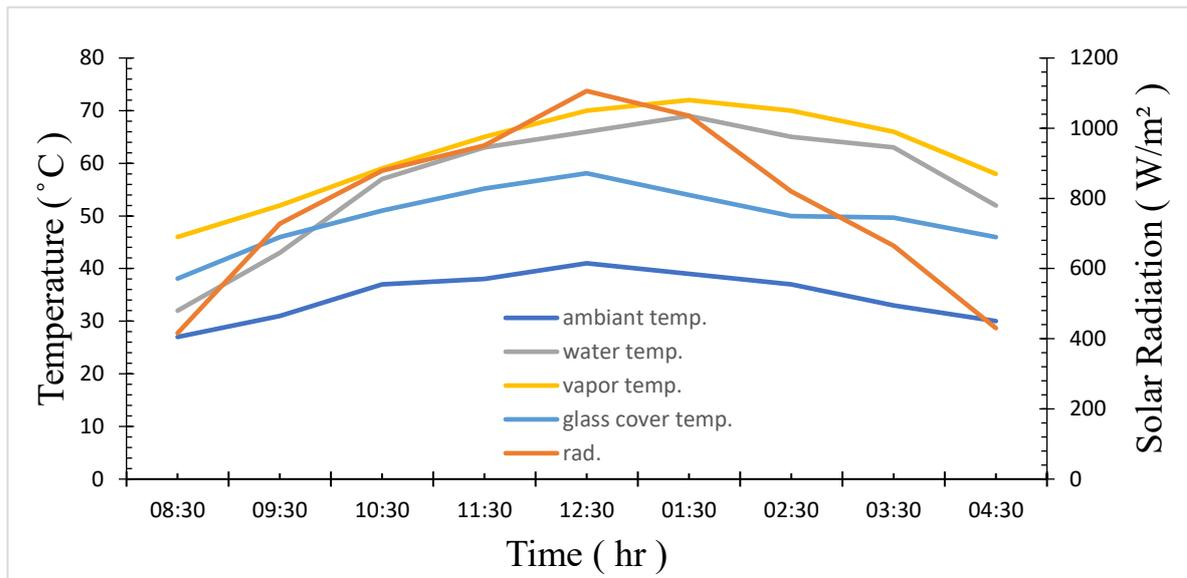
Figure 4.45: variation of temperature and solar radiation with measurement time for solar still with U shape water channel at 1.5 L/min.
