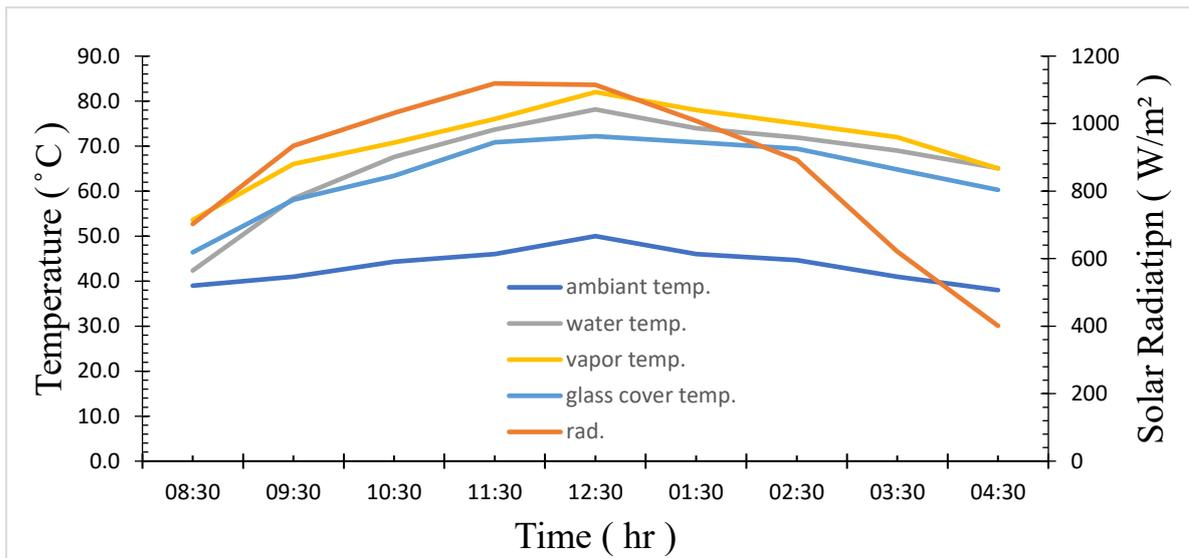
Figure 4.50: variation of temperature and solar radiation with measurement time for conventional solar still
