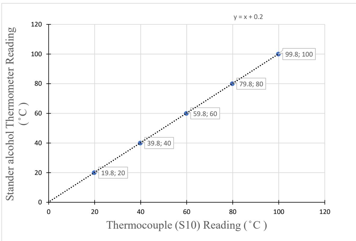
Figure A .10: Thermocouple (S10) calibration, ISS 2, vapor
