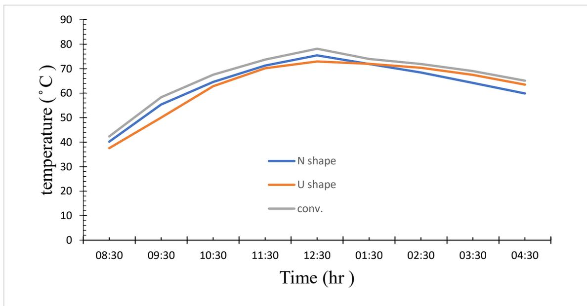
Figure 4.53: variation of basin water temperature with time of experiment
