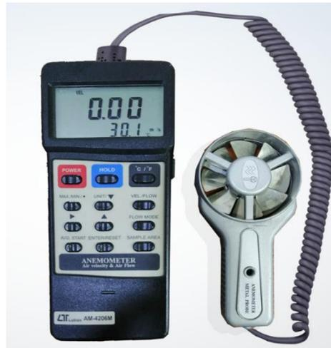
Figure 3.4 Wind speed measuring device (anemometer)
