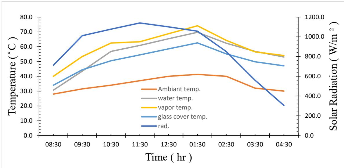
Figure 4.10: variation of temperature and solar radiation with time for solar still with 7 mm diameter copper pipe
