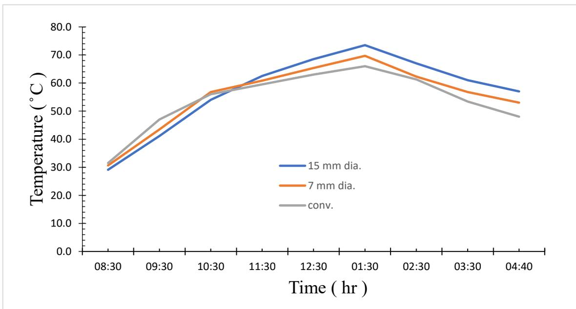
Figure 4.11: variation of basin water temperature with the time of the experiments
