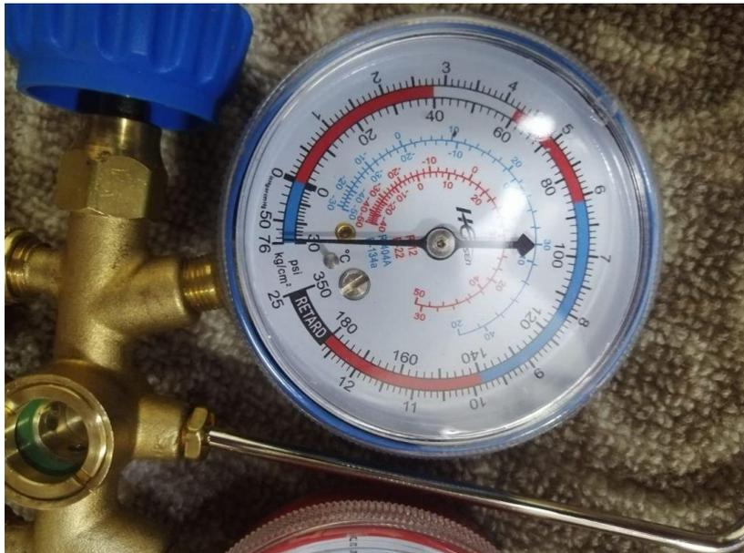
Figure B.2: low pressure gauge
