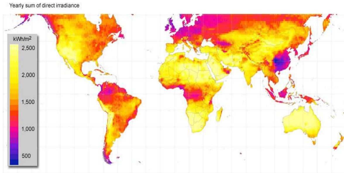
Figure 1.1 (A): World direct normal solar irradiation [4]
