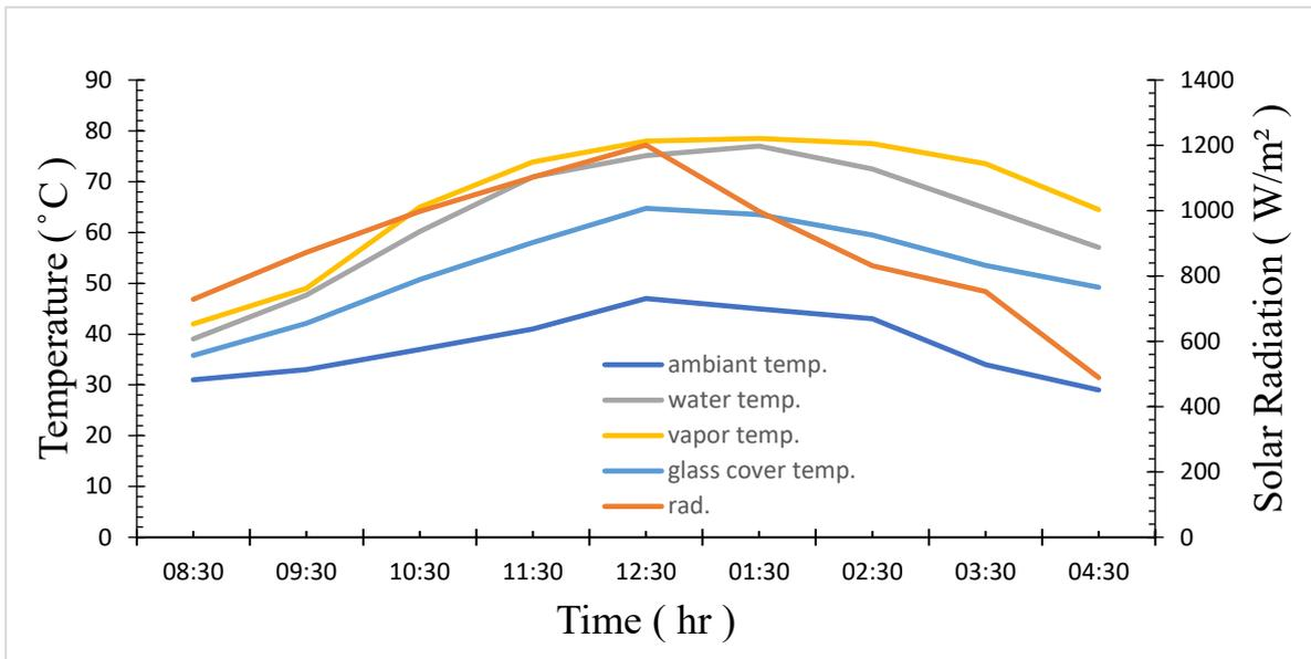
Figure 4.29: variation of temperature and solar radiation with measurement time for conventional solar still
