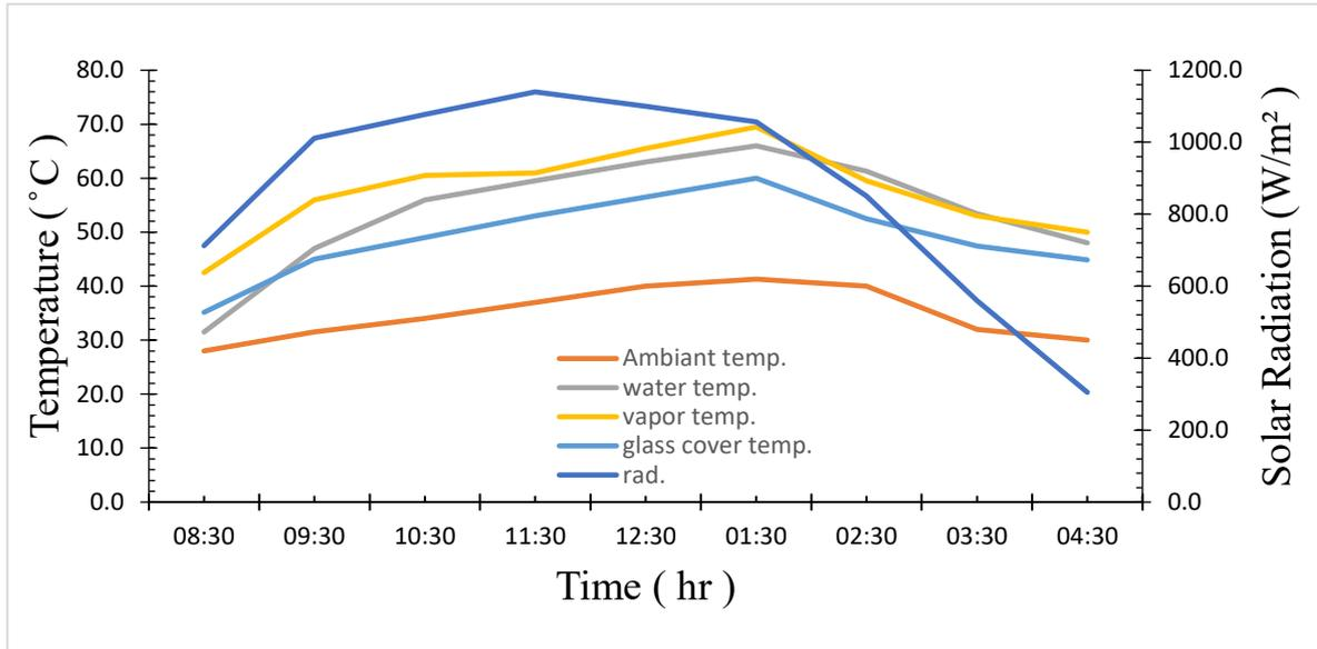
Figure 4.8: variation of temperature and solar radiation with time for conventional solar still
