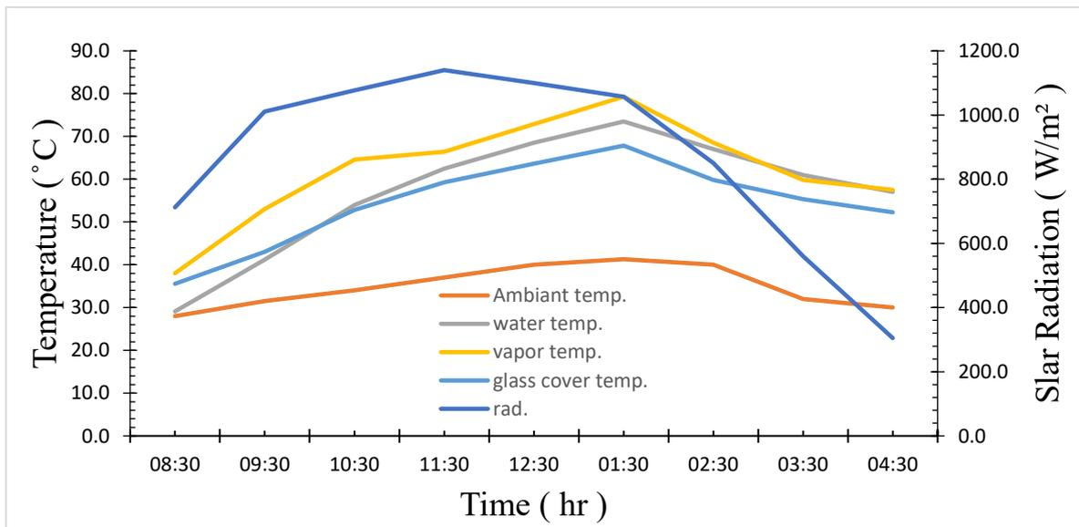
Figure 4.9: variation of temperature and solar radiation with time for solar still with 15 mm diameter copper pipe
