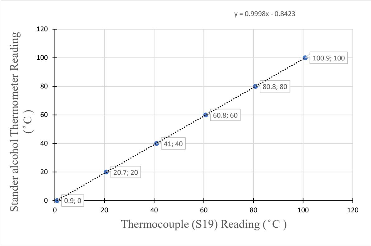
Figure A .19: Thermocouple (S19) calibration, ambient
