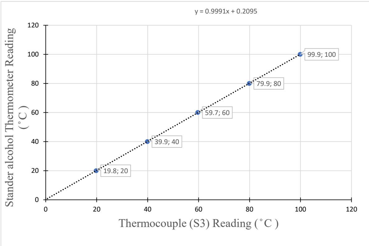
Figure A .3: Thermocouple (S3) calibration, ISS 1, vapor
