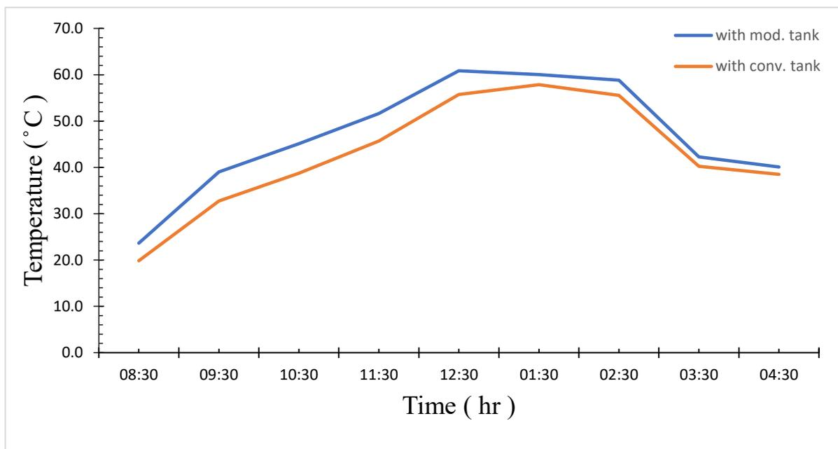
Figure 4.5: variation of vapor temperature with time of the experiment
