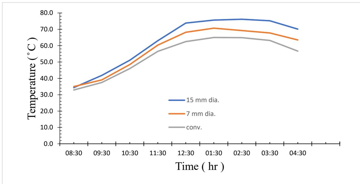
Figure 4.18: variation of basin water temperature with the time of the experiment
