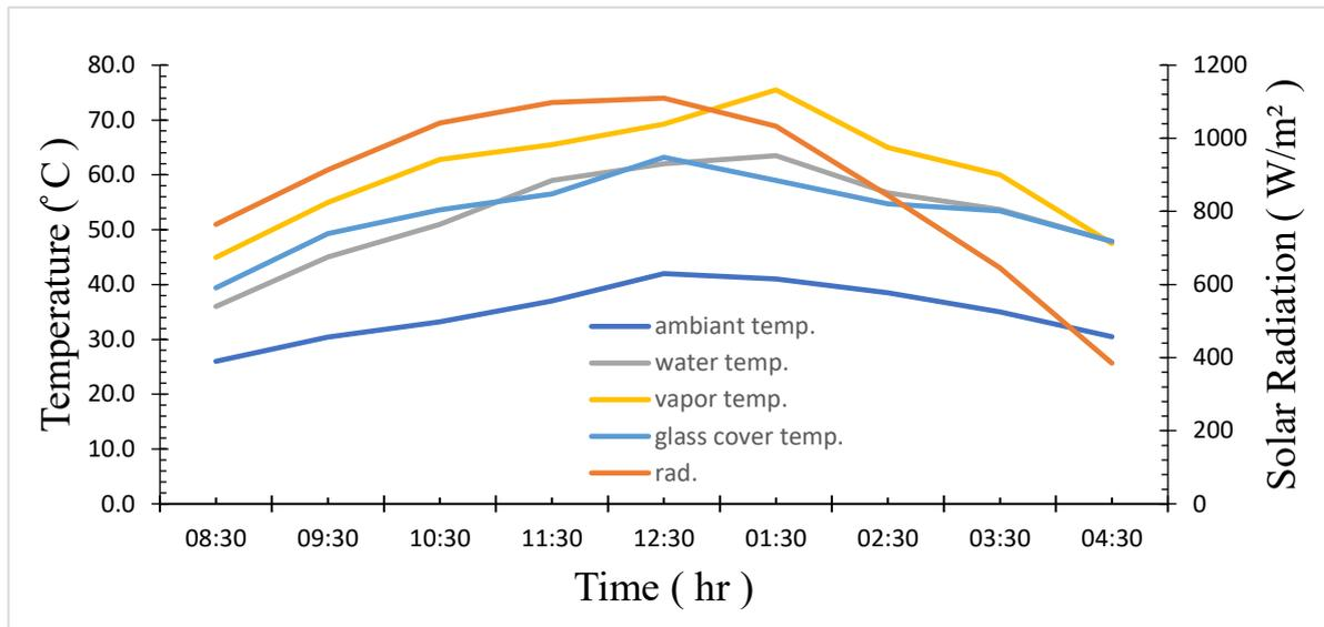
Figure 4.36: variation of temperature and solar radiation with measurement time for conventional solar still
