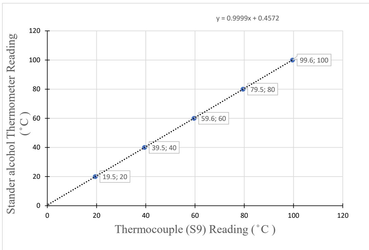
Figure A .9: Thermocouple (S9) calibration, ISS 2, vapor
