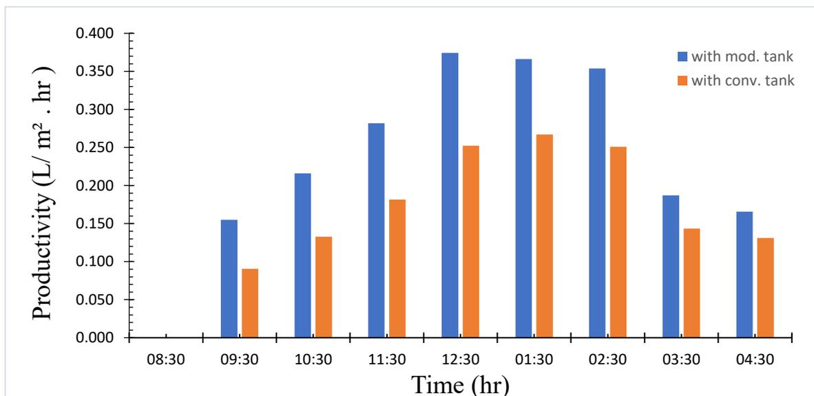
Figure 4.7 productivity variation with time for conventional and modified solar stills
