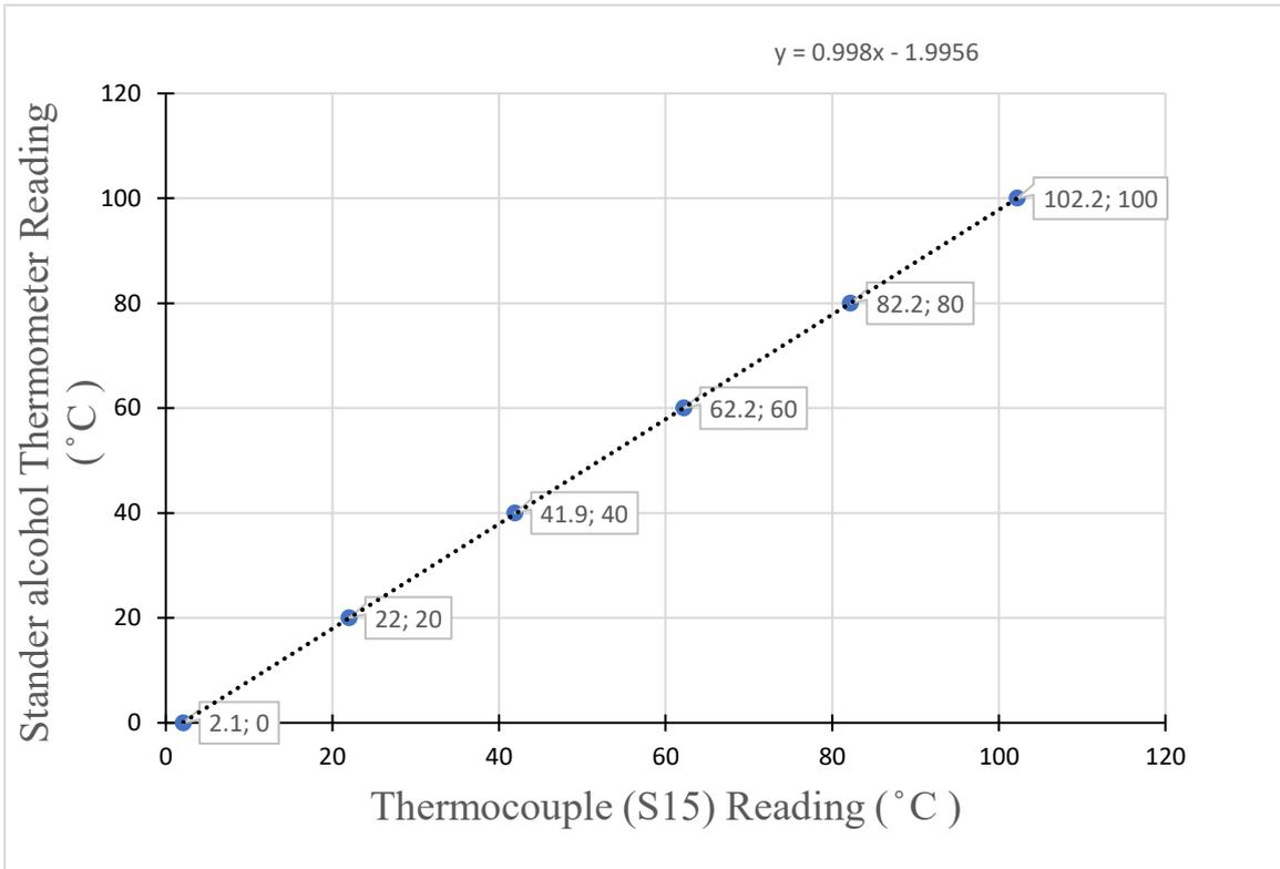
Figure A .15: Thermocouple (S15) calibration, CSS, vapor
