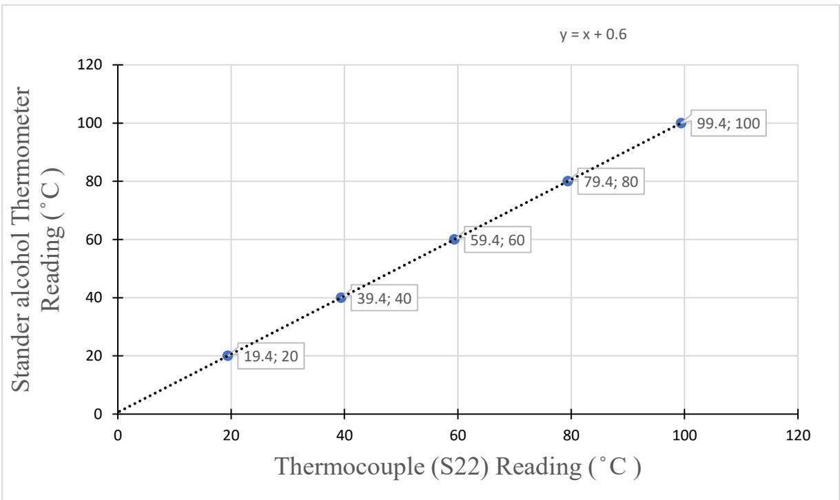
Figure A .22: Thermocouple (S22) calibration
