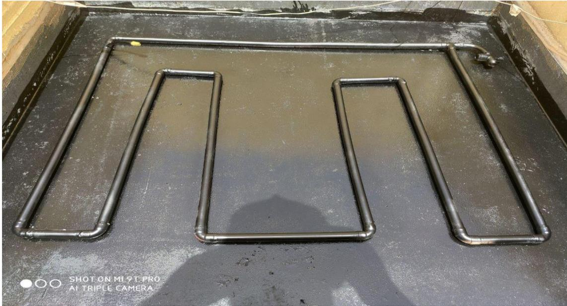
Figure 3.7 Evacuated copper tube
