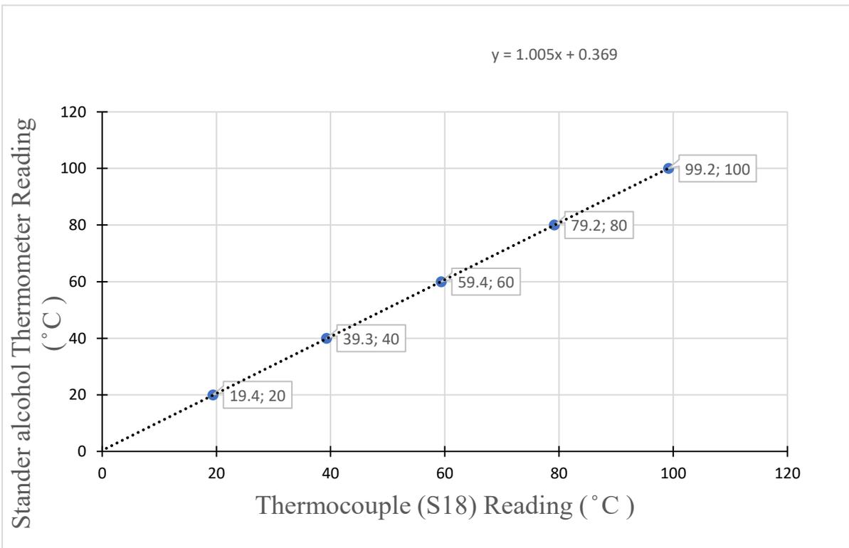
Figure A .18: Thermocouple (S18) calibration, CSS, glass cover
