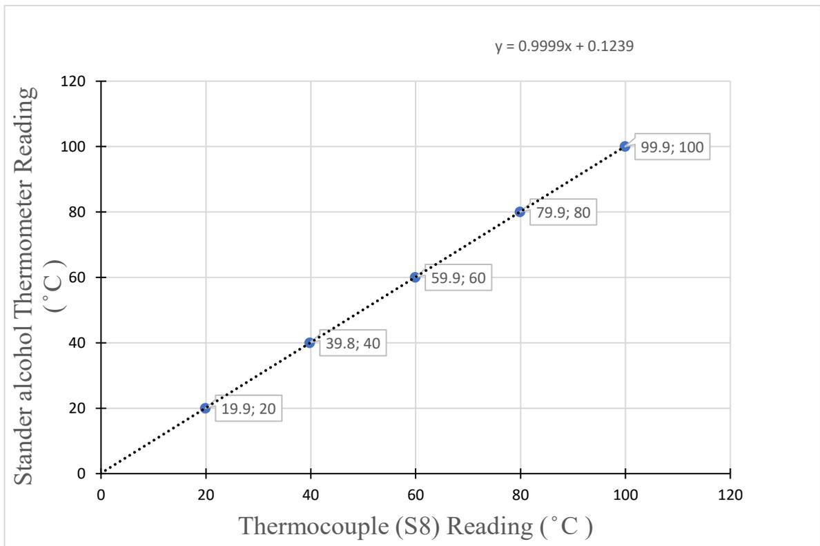
Figure A .8: Thermocouple (S8) calibration, ISS 2, basin water
