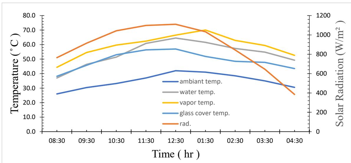
Figure 4.37: variation of temperature and solar radiation with measurement time for solar still with N shape water channel at 1 L/min.
