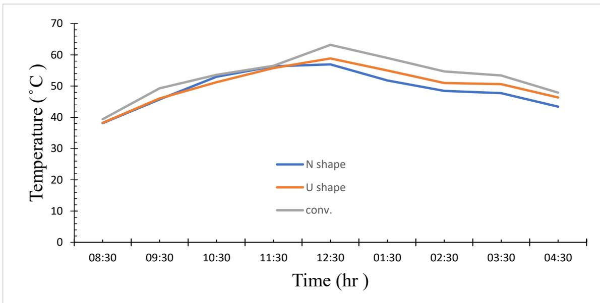
Figure 4.41: variation of glass cover temperature with the time of the experiment
