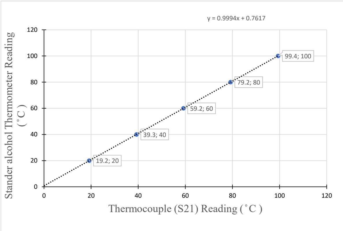
Figure A .21: Thermocouple (S21) calibration
