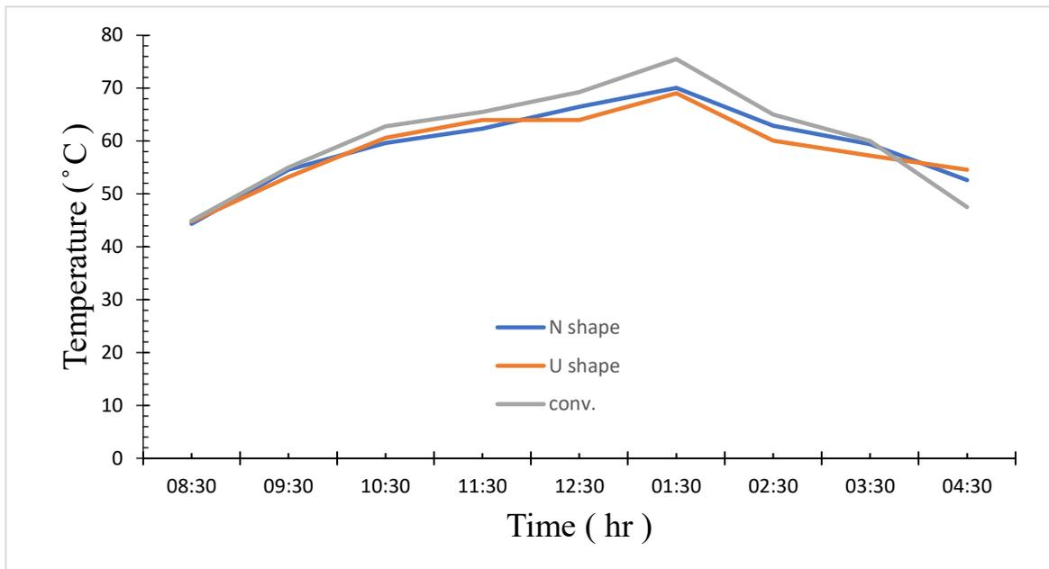
Figure 4.40: variation of vapor temperature with the time of the experiment
