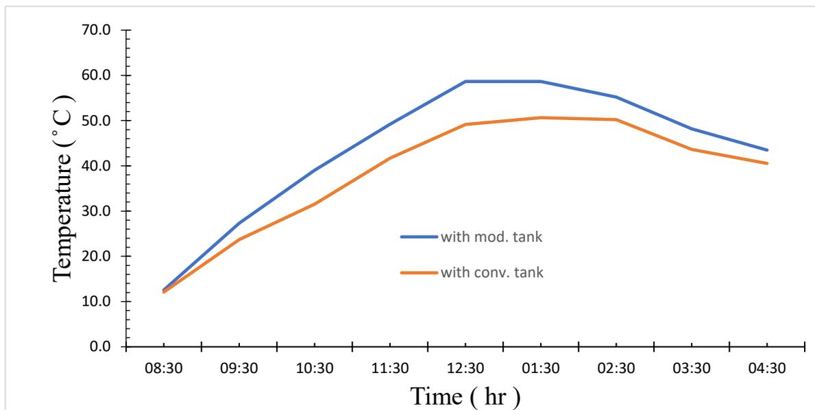
Figure 4.4: variation of basin water temperature with the time of the experiment
