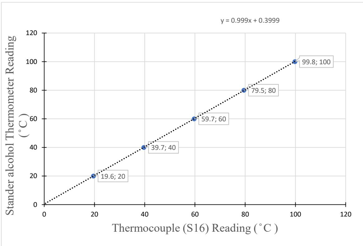
Figure A .16: Thermocouple (S16) calibration, CSS, vapor
