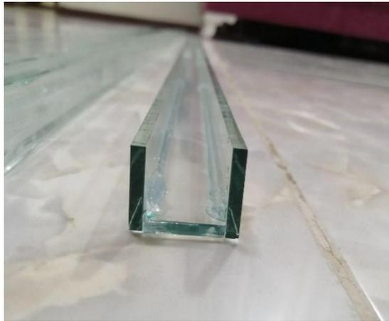
Figure 3.11 Glass cooling water channel
