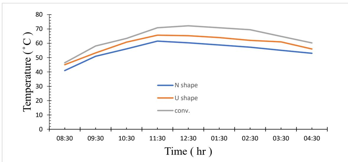
Figure 4.55: variation of glass cover temperature with the time of the experiment
