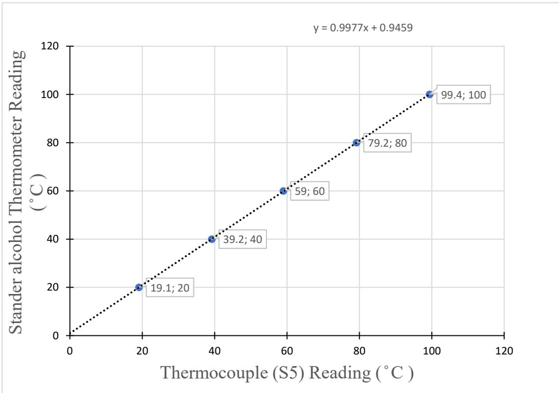
Figure A .5: Thermocouple (S5) calibration, ISS 1, glass cover
