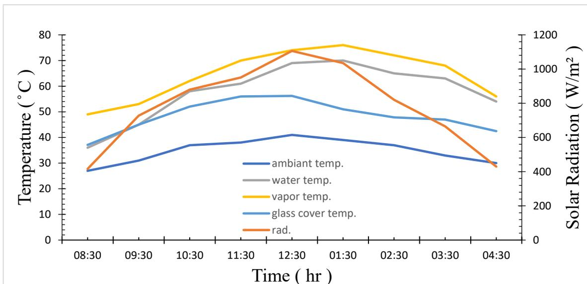
Figure 4.44: variation of temperature and solar radiation with measurement time for solar still with N shape water channel at 1.5 L/min.
