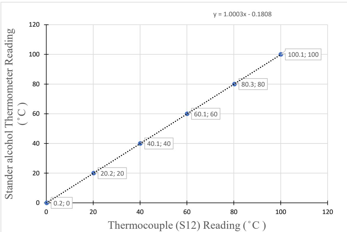
Figure A .12: Thermocouple (S12) calibration, ISS 2, glass cover
