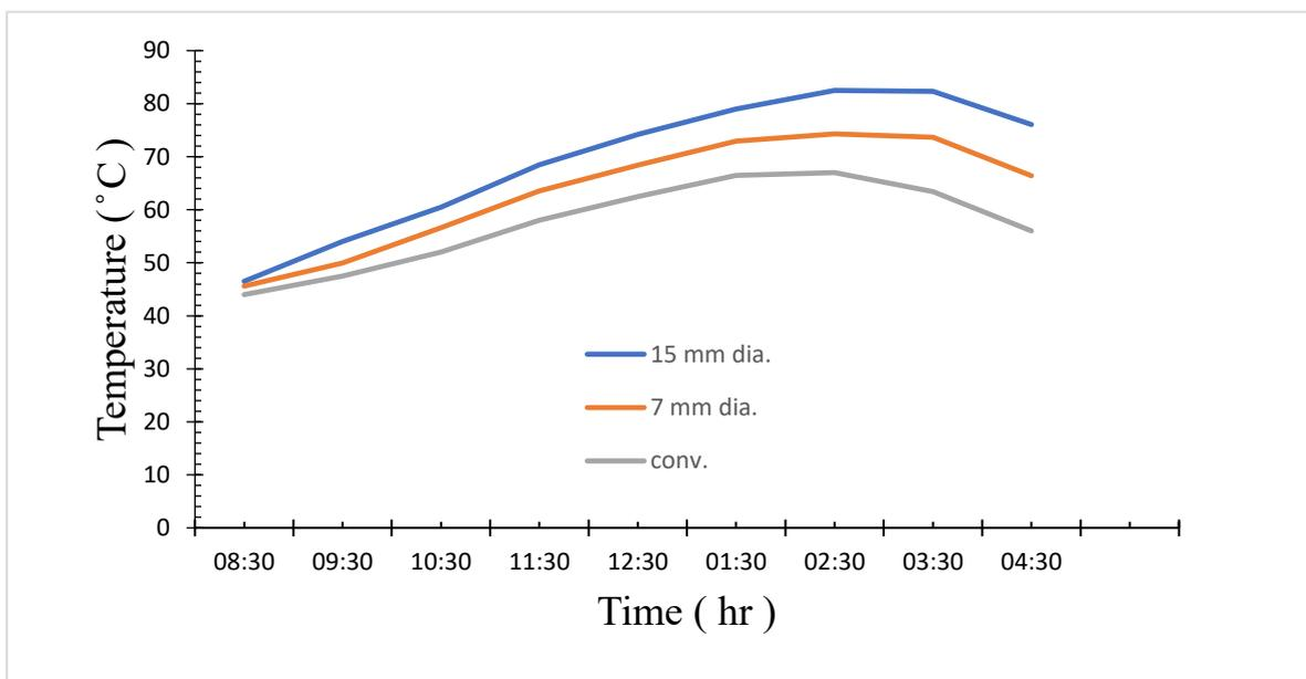
Figure 4.19: variation of basin water temperature with the time of the experiment
