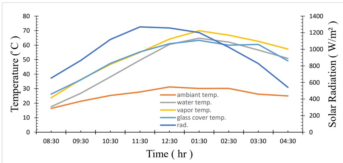
Figure 4.24: variation of temperature and solar radiation with measurement time for still with 50 \* 50 grid size wick
