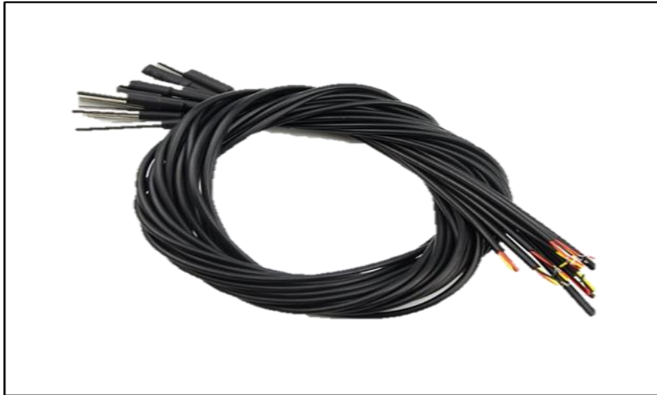
Fig. 4.7: Eight temperature sensors.
