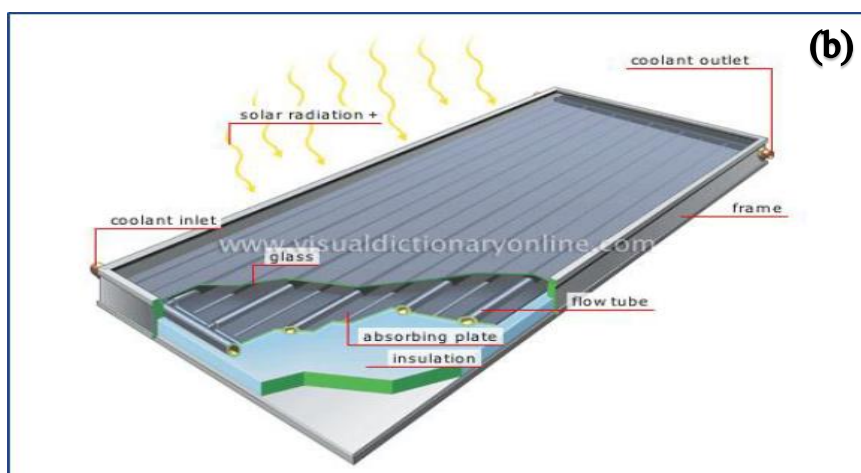
Fig. 1.3: Flat plate solar collector (FPC) [web site].
