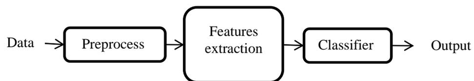
Figure 2.4. The block diagram of the system that used for automatic seizure detection.
