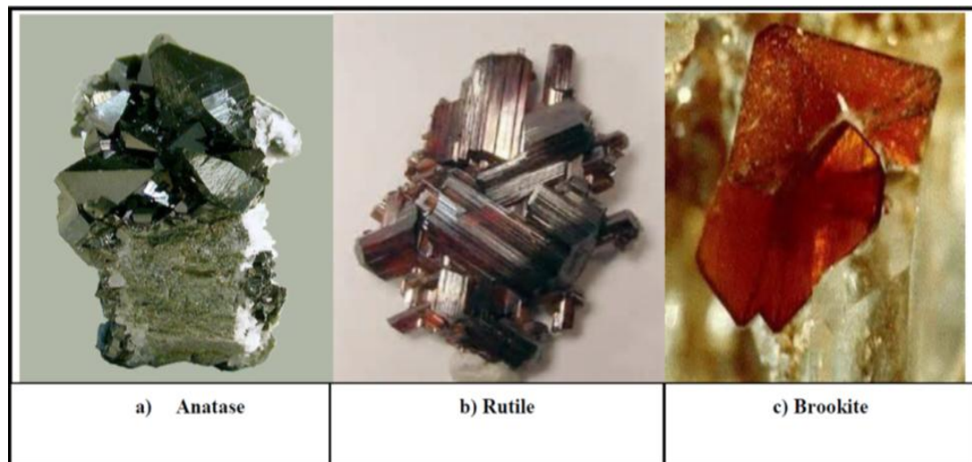
Figure 4.2 Crystalline Forms of Titanium Dioxide, Anatase, Rutile, and Brookite[49]
