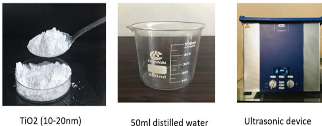
Figure 4.5 TiO 2 prepared procedure.
