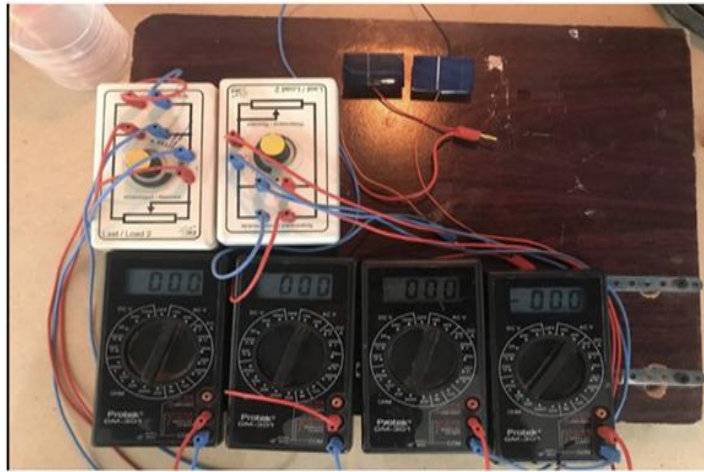
Solar cell's test panel
