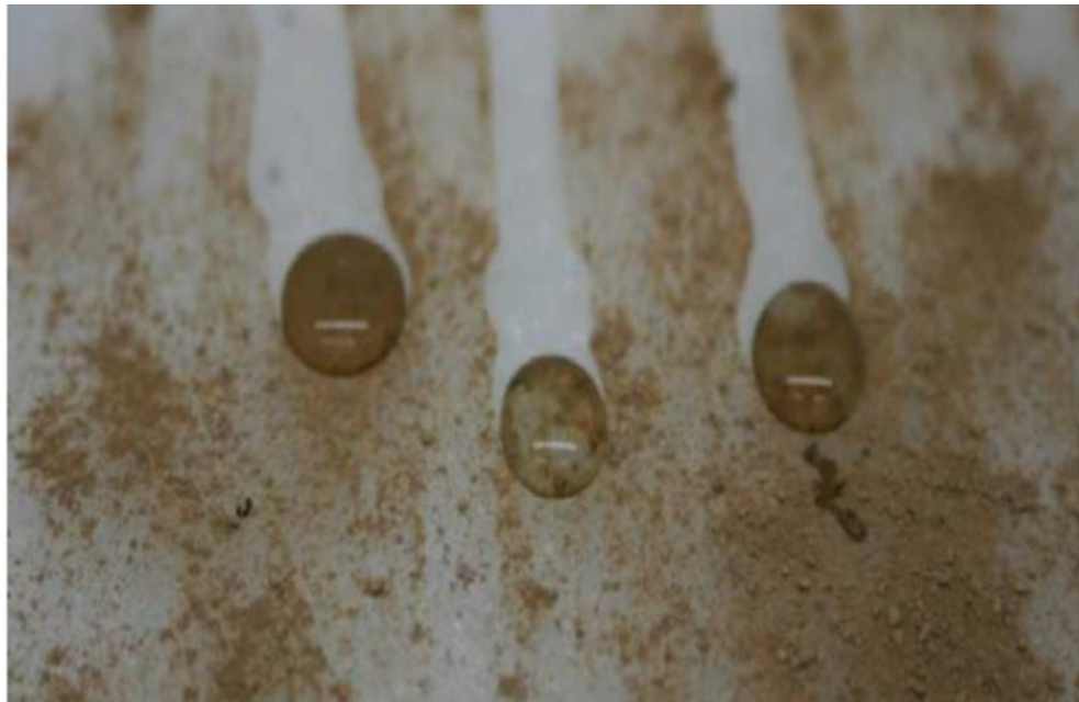
Figure 2.4 water droplets rolling down carrying the dust particles on the superhydrophobic surface[43].
