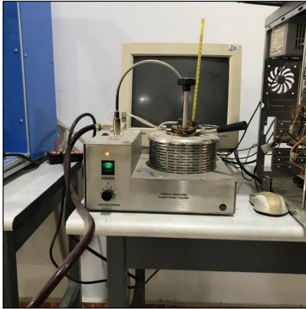
Figure 3-5 flash point test by Pensky martens flash point tester.
