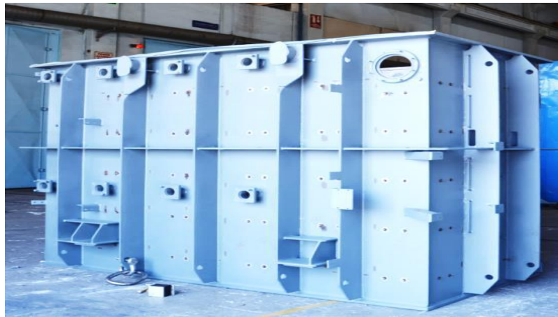
Fig. 1.9: The Transformer housing [14].
