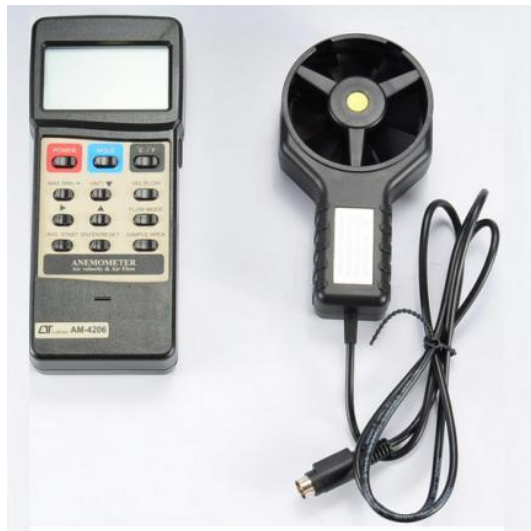
Figure 4.5 Anemometer to measure airflow velocity
