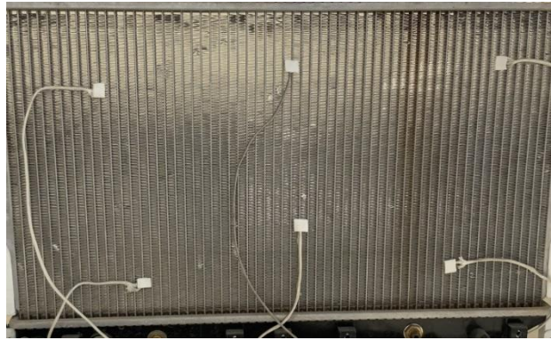
Figure 4.11 Distribution of thermocouples on the radiator
