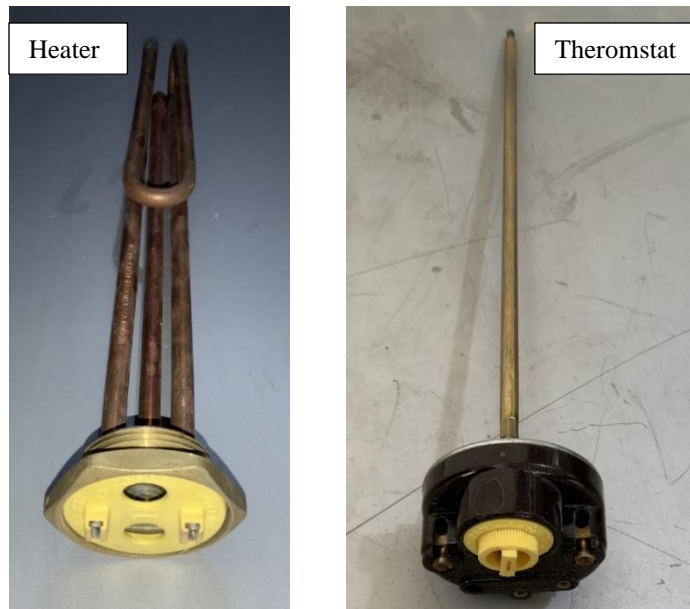
Figure 4.9 water heater and thermostat
