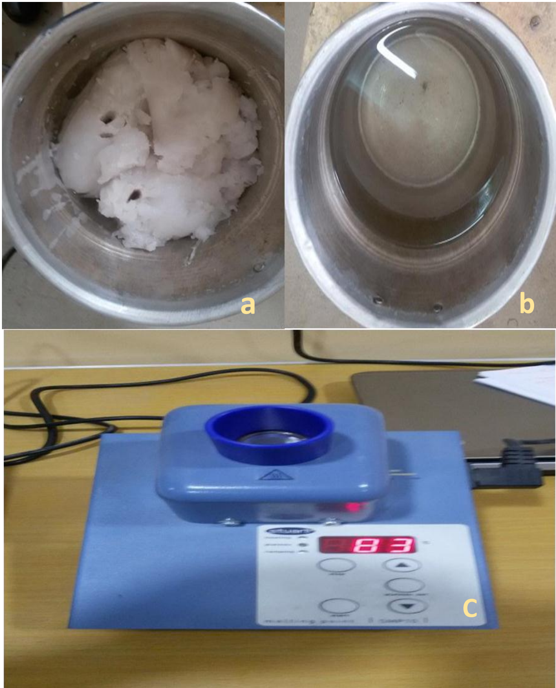
Figure (4-14): Paraffin Wax (PCM) Before (a), After Melting (b), and the Device for Estimating the Melting Point of Paraffin Wax (c)
