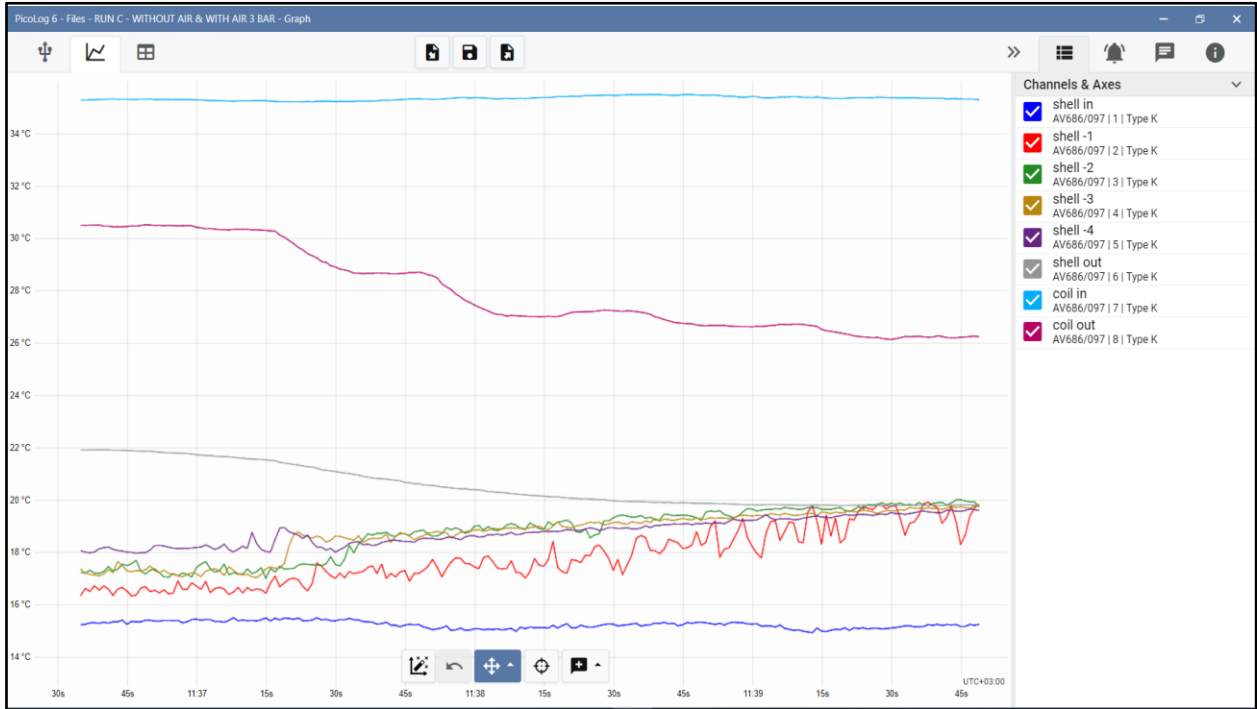
Figure 3.14 represent the screen capture of the measured temperatures along with the heat exchanger.
