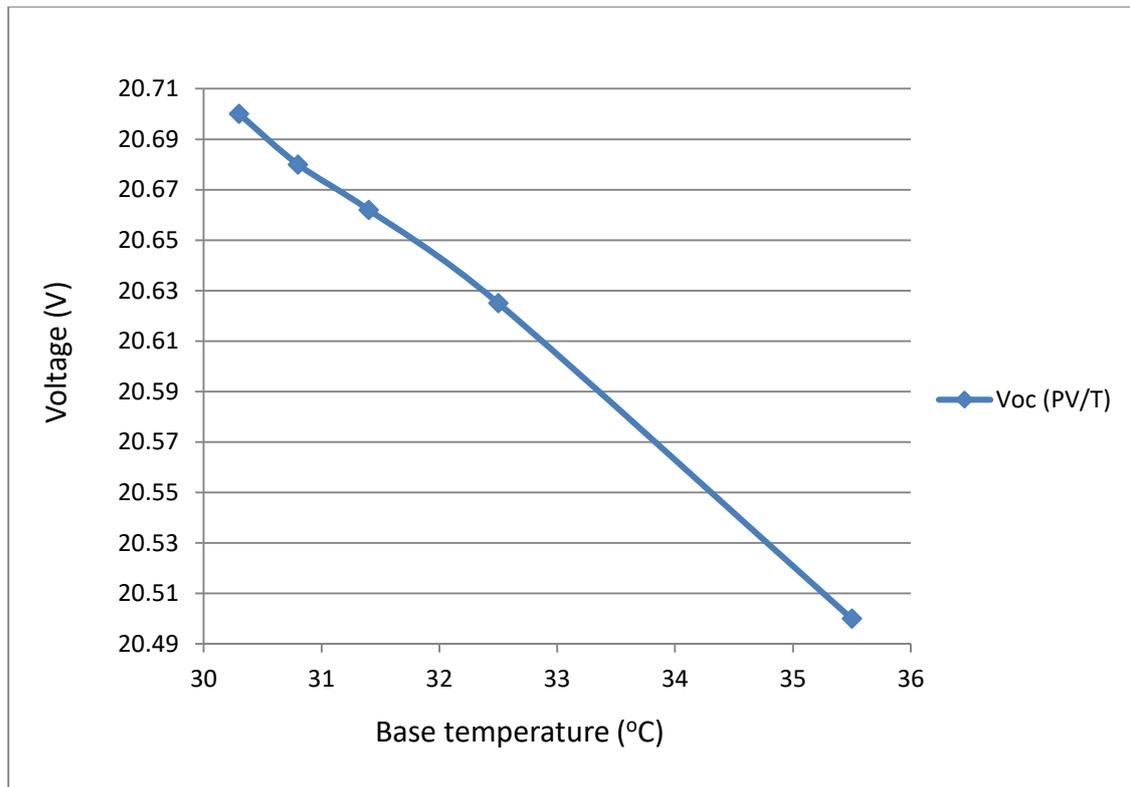
Figure 5-21 Effect of  $T_b$  over  $V_{oc}$  for PV/T system under solar radiation of  $1000 \text{ w/m}^2$  and volume flow rate of (1 to 5) LPM.
