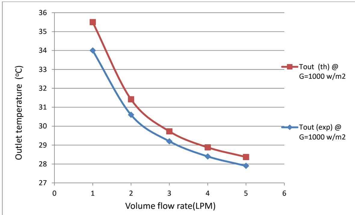
Figure 5-27 Outlet temperature  $T_o$  over volume flow rate in comparison on numerical and experimental results for PV/T water system.
