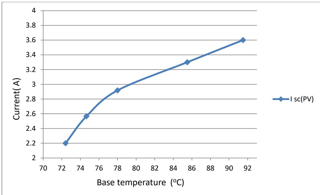
Figure 5-10 Short circuit current  $I_{sc}$  at the various of the base temperature  $T_b$  of PV module under solar radiation (600 - 1000)  $W/m^2$
