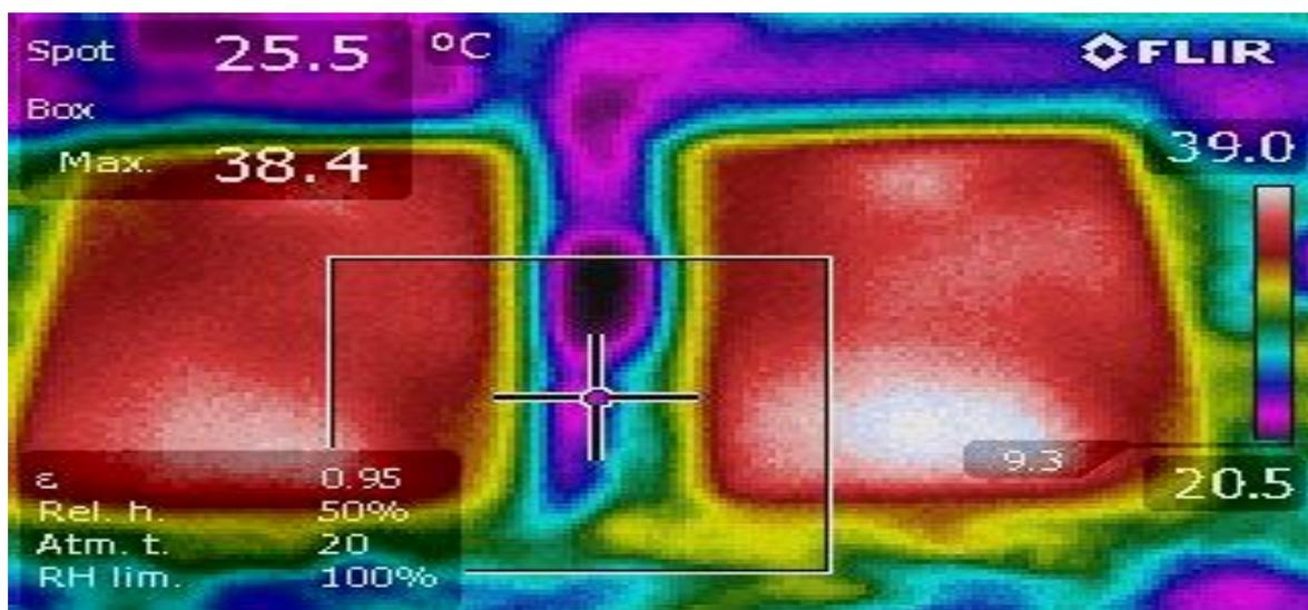
Figure 4-3 Real thermal image of Mono-crystalline PV panel [62].
