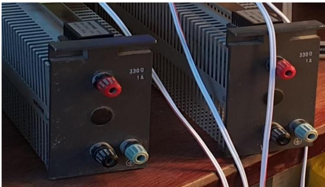
Figure 4-12 Variable resistance load.
