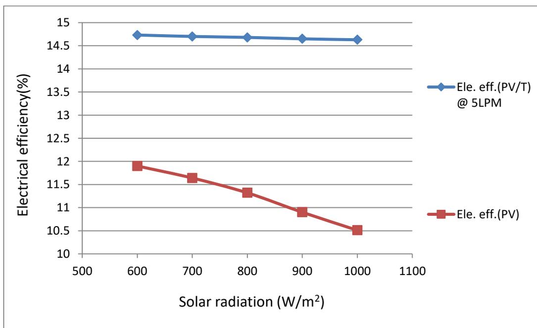
Figure 5-25 Electrical efficiency of PV/T water system and PV panel variation with different solar irradiances at volumetric flow rate of 5 LPM.
