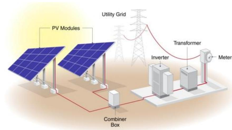
Figure1-1 Main solar energy system components (Ground-mounted array diagram) [4].
