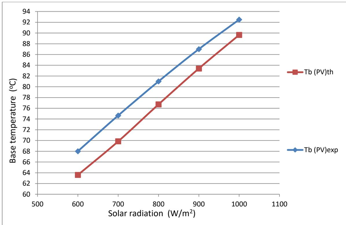
Figure 5-26 Base temperature  $T_b$  over solar radiation in comparison on numerical and experimental results for PV panel.
