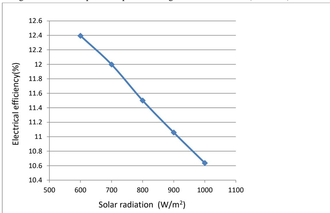
Figure 5.4 Electrical efficiency  $\eta_e$  against solar radiation (600-1000) W/m<sup>2</sup> for (PV) panel.
