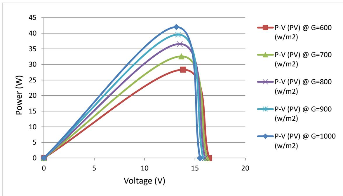
Figure 5-14 P-V curve for PV module for different solar radiation.
