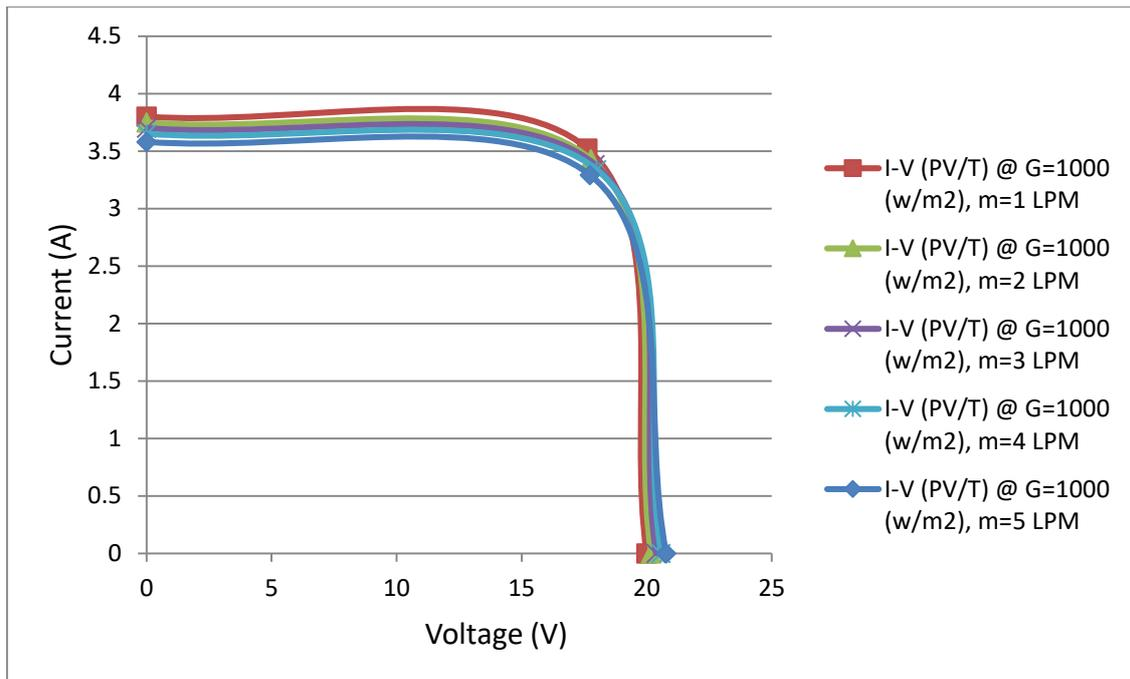
Figure 5-17 *I-V* curve of the PV/T module for various volume flow rate at  $1000 \text{ (w/ m}^2\text{)}$ .
