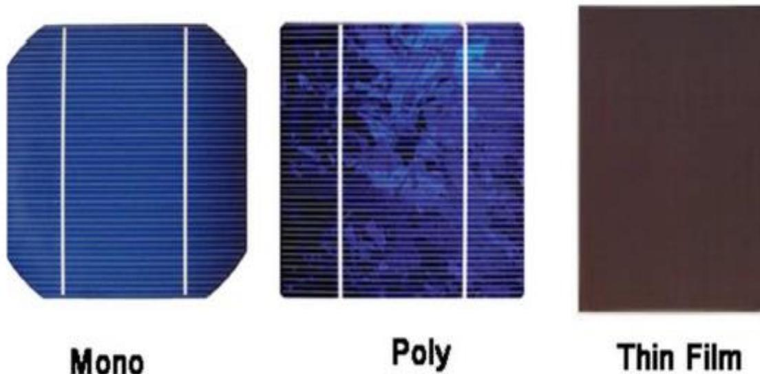
Figure 1-4 Types of PV Panels [16].
