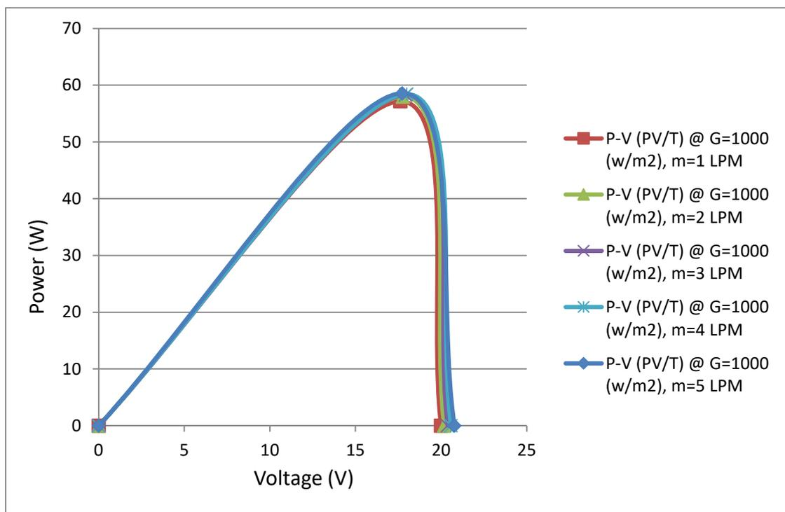
Figure 5-18 *P-V* curve of the PV/T module for various volume flow rate at  $1000 \text{ (w/ m}^2\text{)}$ .
