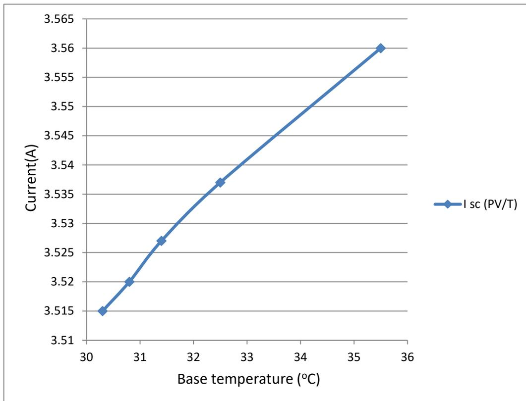
Figure 5-22 Effect of  $T_b$  over  $I_{oc}$  for PV/T system under solar radiation of  $1000 \text{ w/m}^2$  and volume flow rate of (1 to 5) LPM.
