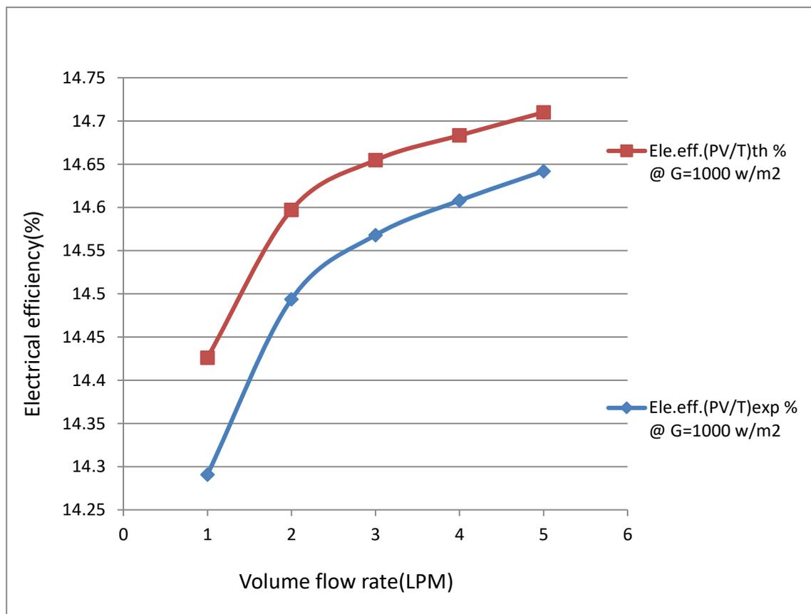
Figure 5-28 Electrical efficiency  $\eta_e$  over volume flow rate in comparison on numerical and experimental results for PV/T water system.
