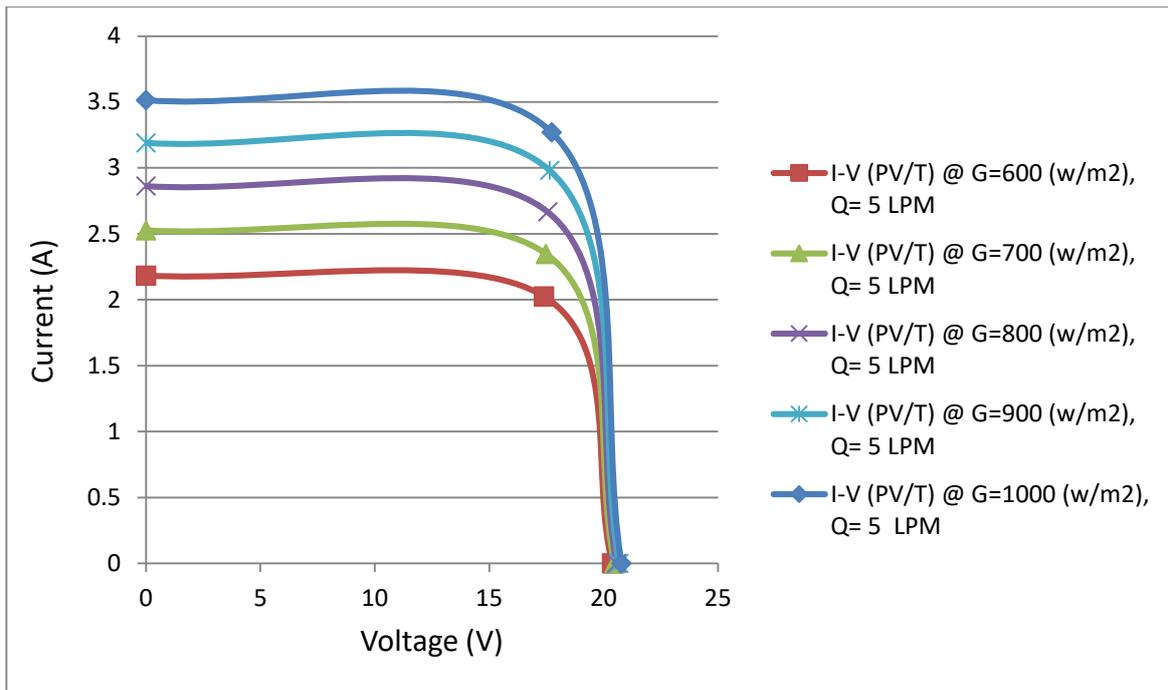
Figure 5-15 I-V curve for PV/T module for different solar radiation at  $m = 5$  LPM.
