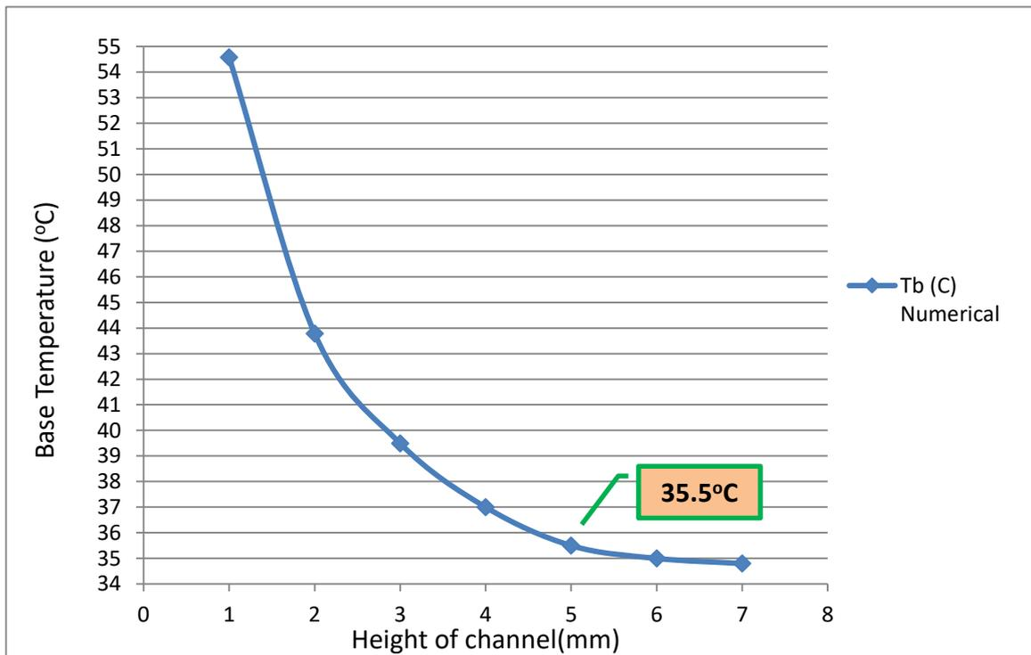
Figure 5-1 Relationship between water channel height and base temperature of PV/T system at  $1000 \text{ W/m}^2$  and 1LPM.
