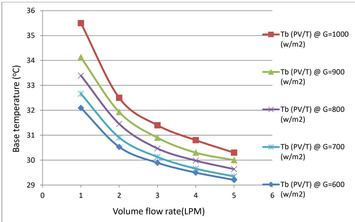
Figure 5-23 Changes of base temperature ( $T_b$ ) of water PV/T system over volume flow rates under various solar irradiance
