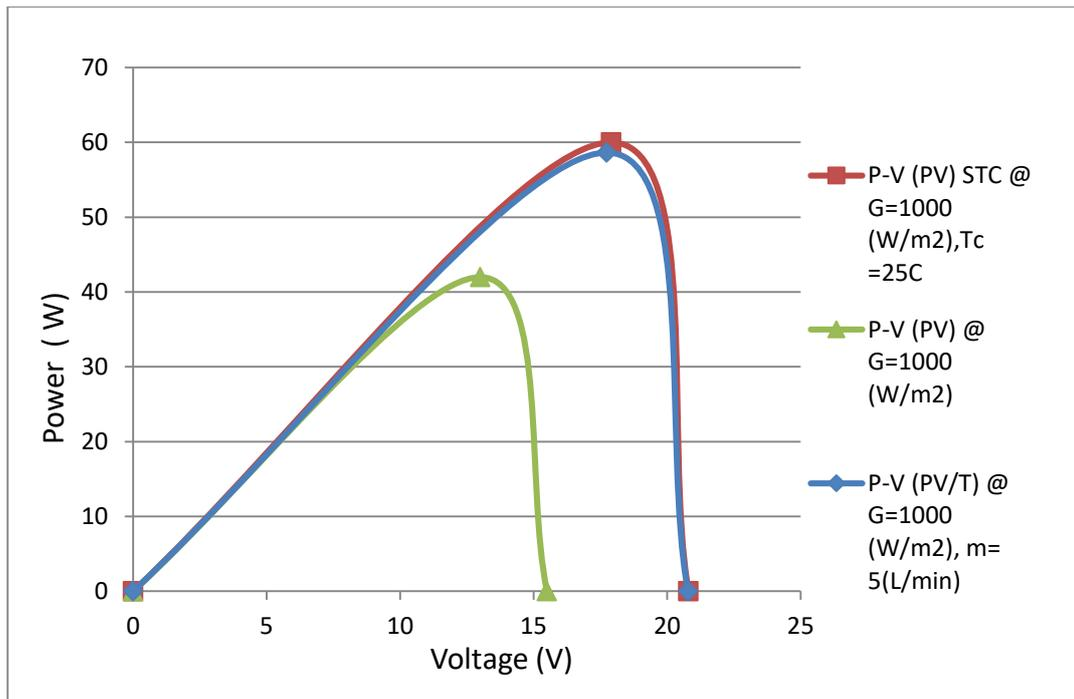
Figure 5-9 PV curve of the PV-STC module, PV module and PV/T water System
