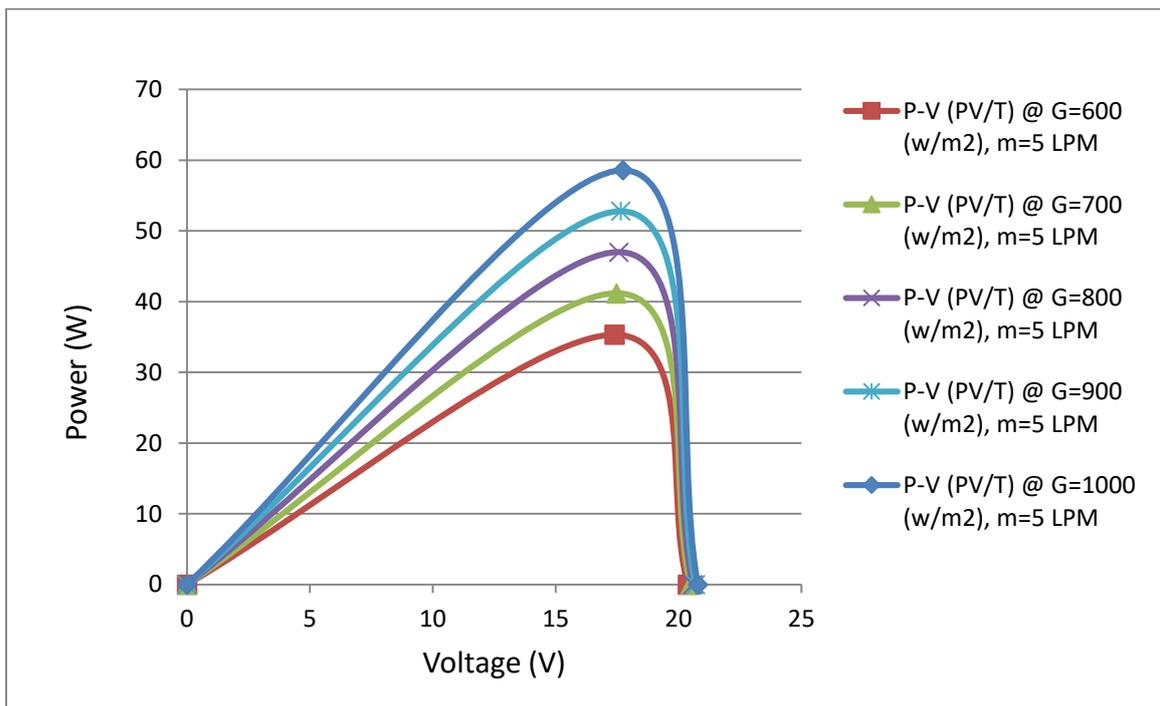
Figure 5-16 Characteristic of PV/T system for different solar radiation at flow rate 5 LPM.
