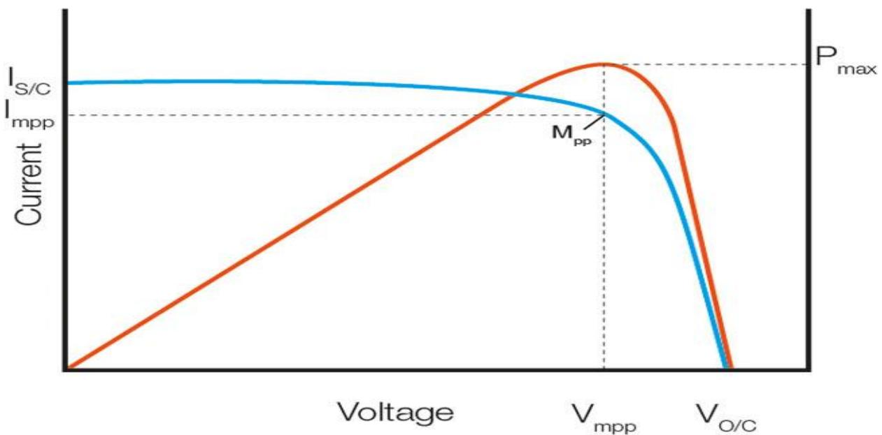
Figure3-5Current-voltage curve of the PV cell [56]
