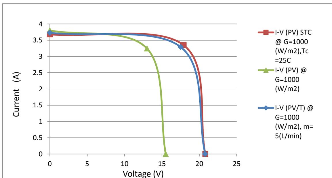
Figure5-8 I-V curve of the PV-STC module, PV module and PV/T water System
