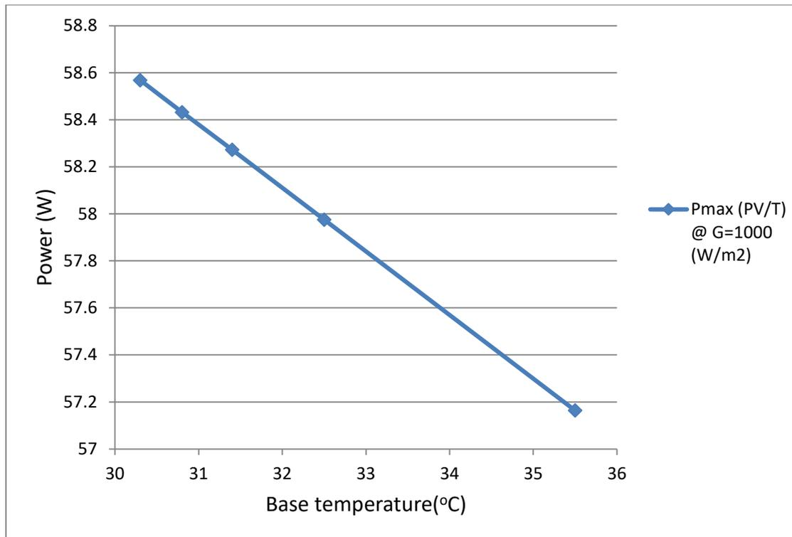
Figure 5-20 Changes of  $P_{max}$  over  $T_b$  of PV/T water system under solar radiation of  $1000 \text{ w/m}^2$  and volume flow rate of (1 to 5) LPM.
