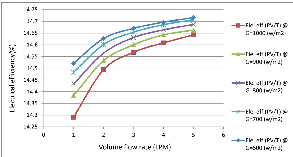
Figure 5-24 Changes of electrical efficiency ( $\eta_{el}$ ) of PV/T system over volume flow rates under various solar irradiance.
