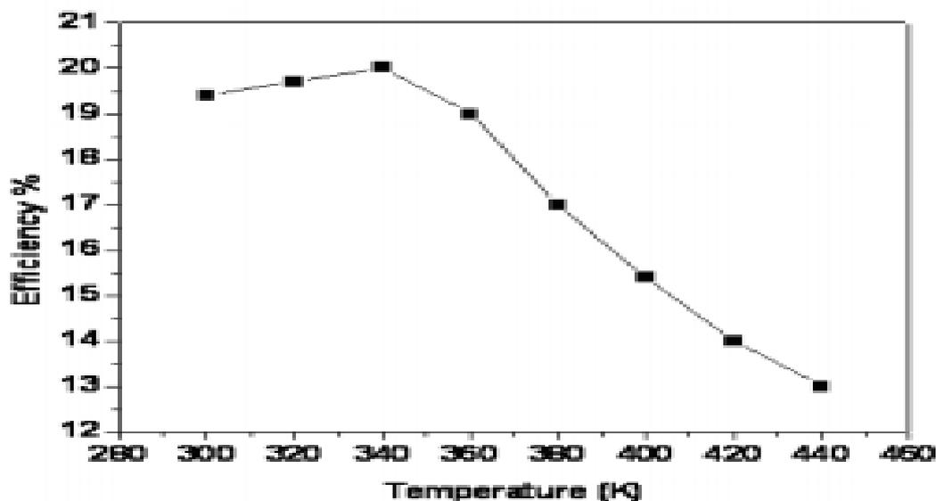
Figure 1-3 A graph of temperature effect on the electrical efficiency of the cell [14].
