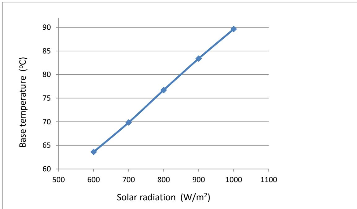
Figure 5.3 Base PV panel temperature  $T_b$  against solar radiation (600-1000) W/m<sup>2</sup>.
