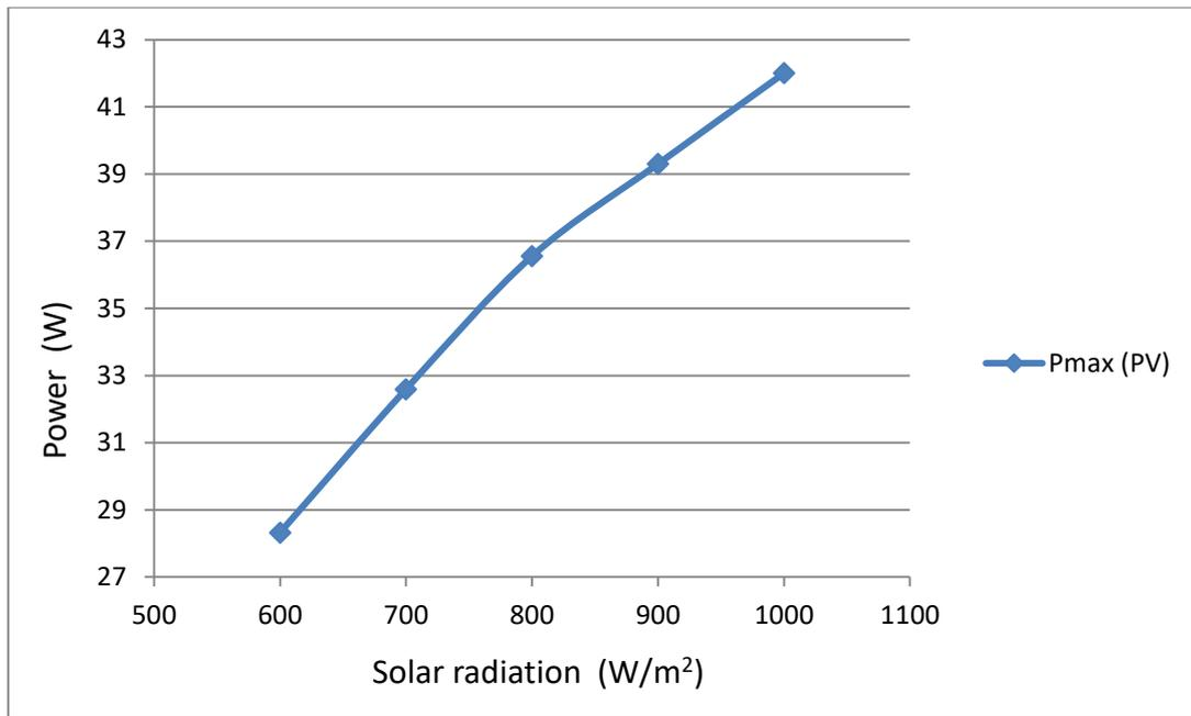
Figure 5-12 Electrical power  $P$  at the various of the solar radiation  $G$  of PV module.
