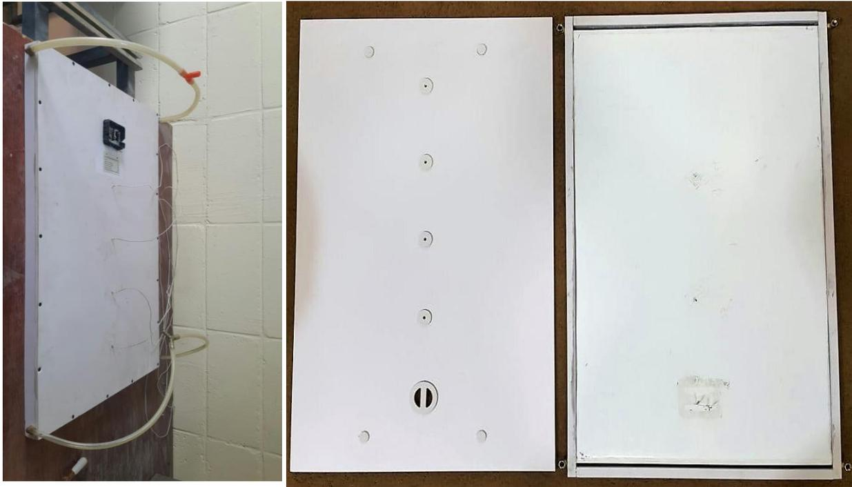
Figure 4-4 Fluid collector channel with PV module (PV/T system).
