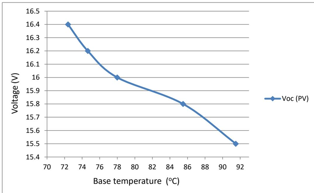
Figure 5-11 Open circuit voltage  $V_{oc}$  at the various of the base temperature  $T_b$  of PV module under solar radiation (600 - 1000)  $W/m^2$
