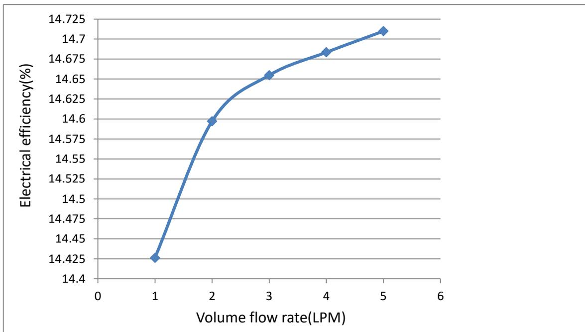
Figure 5.7 Electrical efficiency  $\eta_e$  against water flow rate (1 to 5) LPM at 1000 ( $\text{W}/\text{m}^2$ ).
