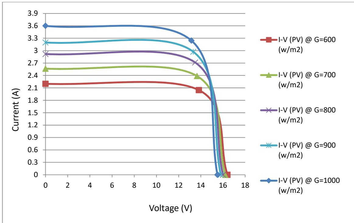
Figure 5-13 I-V curve for PV module for different solar radiation.
