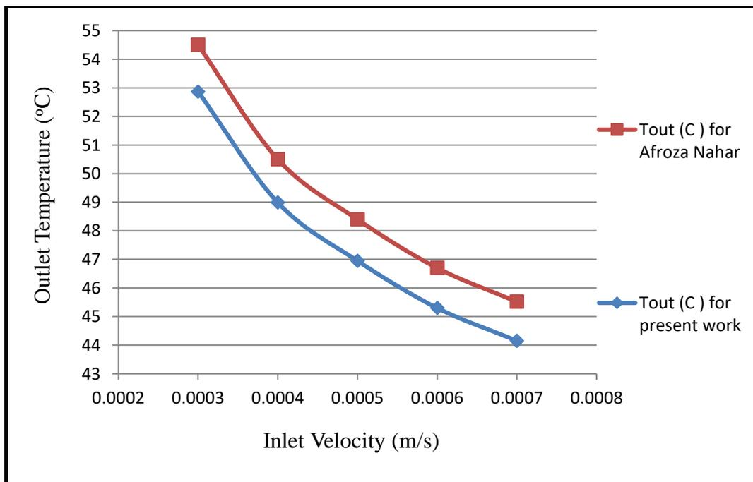
Figure3-4 Outlet water temperatures according to variable mass flow rates for the CFD validation results compared with results regenerated from [53]
