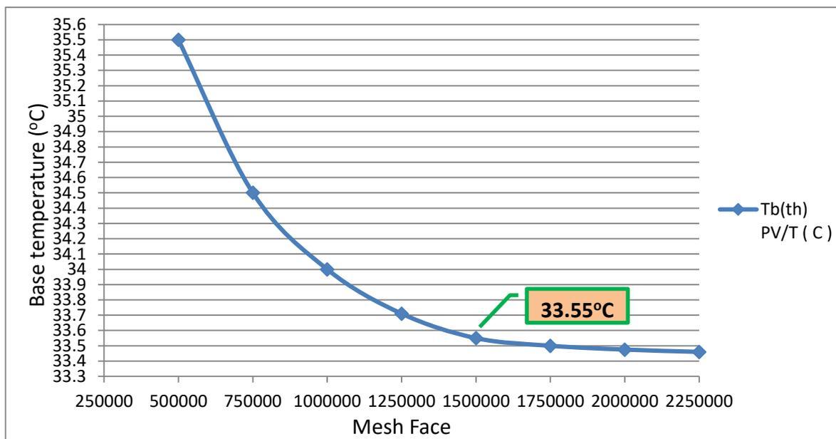
Figure 3-2 Average base temperature of the PV/T system versus a number of the mesh faces for grid independence test.
