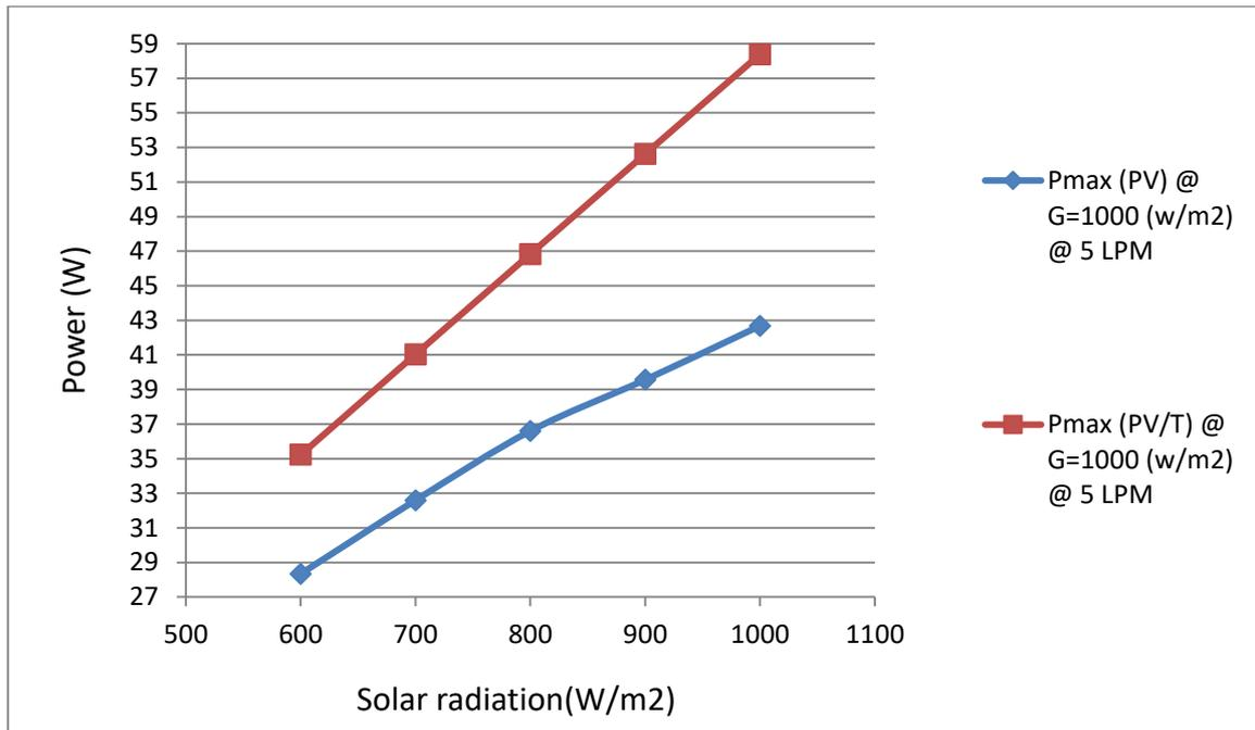
Figure 5-19 The comparison of PV/T water system with traditional PV module on the  $P_{max}$  with various solar radiation at flow rate of 5 LPM.
