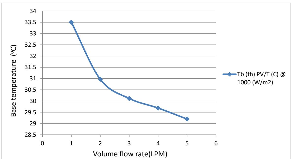
Figure 5.6 Base PV panel temperature  $T_b$  against water flow rate (1to5) LPM at 1000 (W/m<sup>2</sup>).
