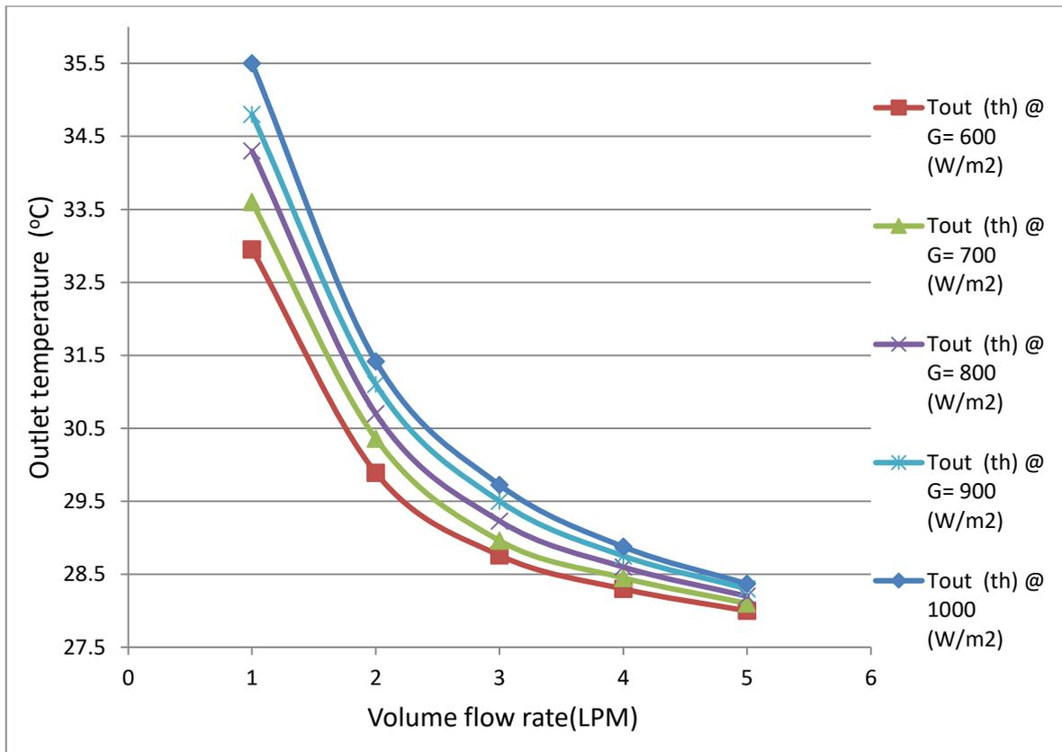
Figure 5.5 Outlet water temperature  $T_o$  against (solar radiation and flow rate) different
