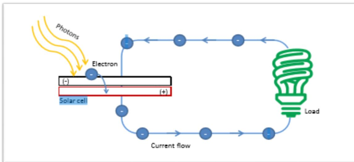
Figure1-2 Electricity generation from a (PV) cell [4]
