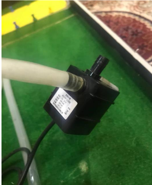
Figure 3.15. Submersible water pump
