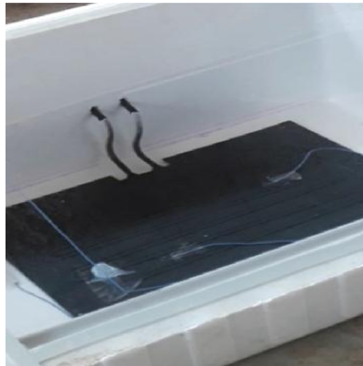
Figure 4.8 Photograph of the heat exchanger
