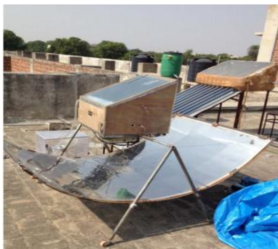
Figure 2.11 Shown experimental work for PTC with single slope solar still.[44]
