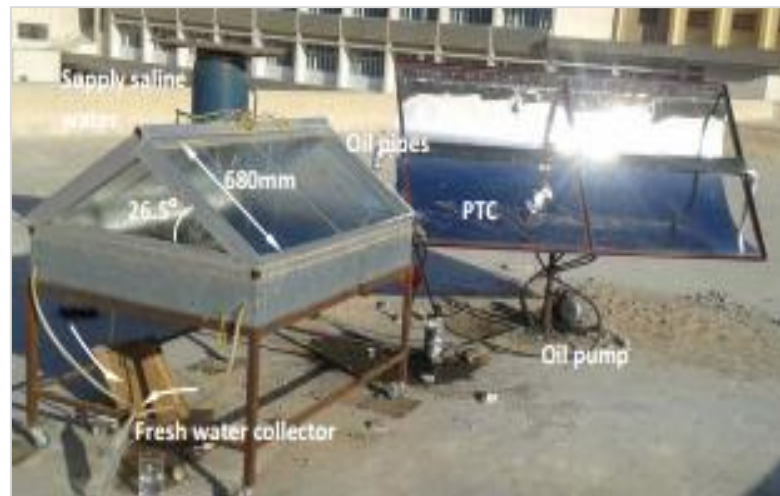
Figure 2.12 Shown components of the systems.[45]
