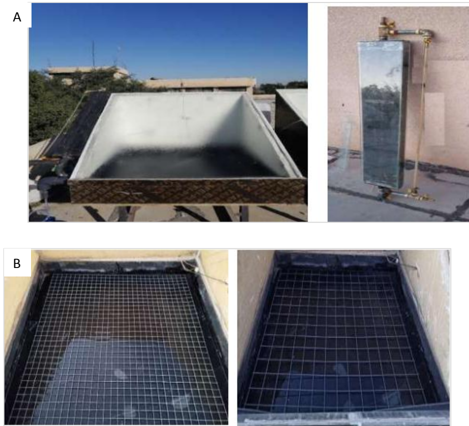
Figure 2.8 (A) Solar energy tank with a solar still. (B) Iron wicks of two different sizes in side solar still. [35]
