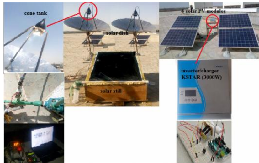
Figure 2.6 Shown the proposed solar water desalination system.[33]
