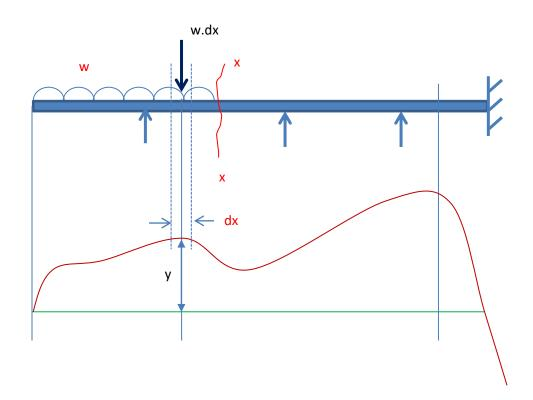
Divide the uniform load into infinite number of small loads{ w.dx at position x}. The magnitude of the influence at section x-x due to (w.dx) will be :
