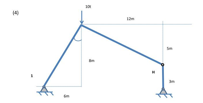
Hint: Separate the structure into two segments at the hinge H. After finding  $V_H$  and  $H_H$  , resolve into  $N_H$  and  $F_H$  .
