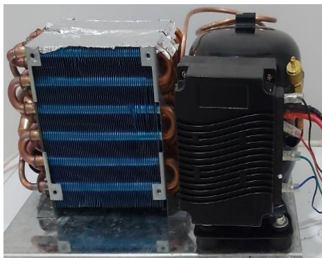
Fig 1: Refrigerated AWG System
