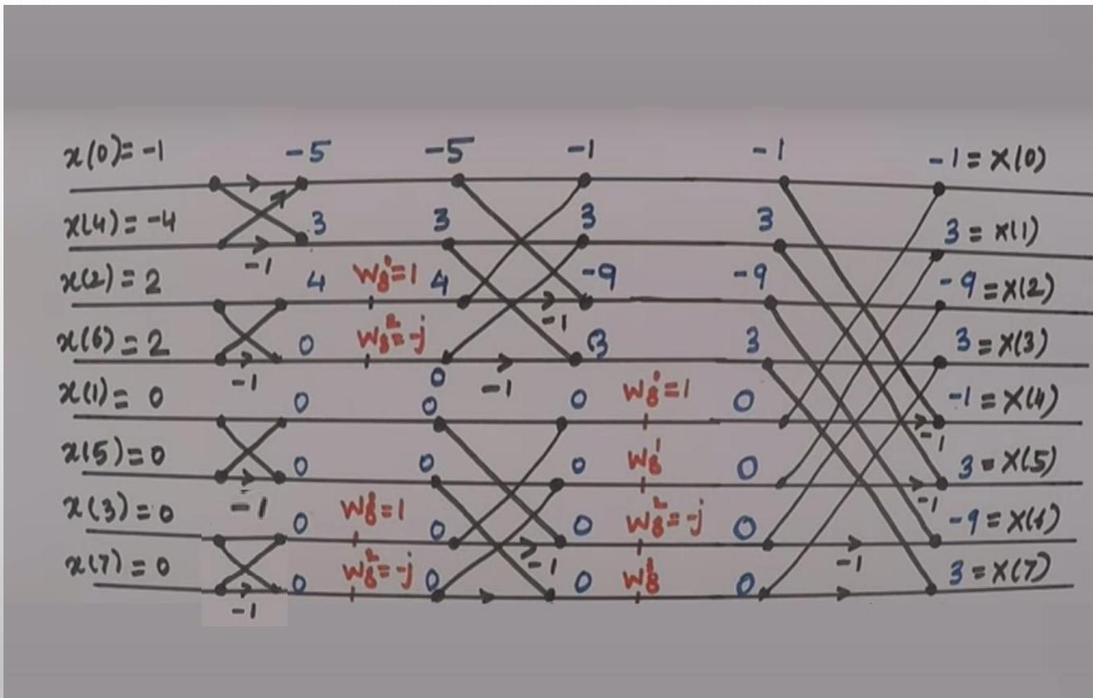
$$X(k) = [ -1 \quad 3 \quad -9 \quad 3 \quad -1 \quad 3 \quad -9 \quad 3 ]$$
