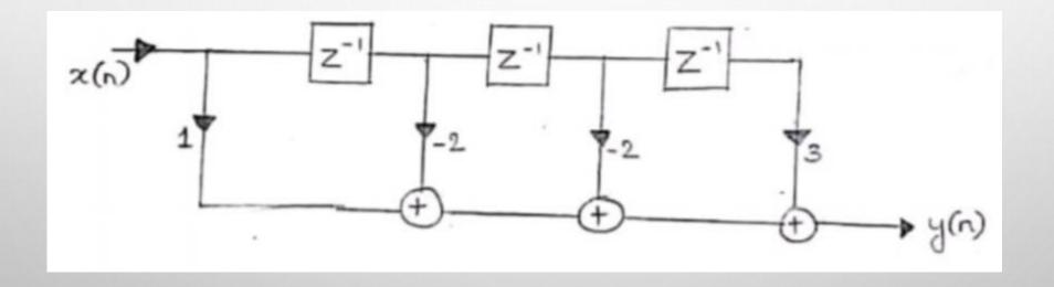
Draw the direct form structure for the FIR filter represented by the following transfer function
