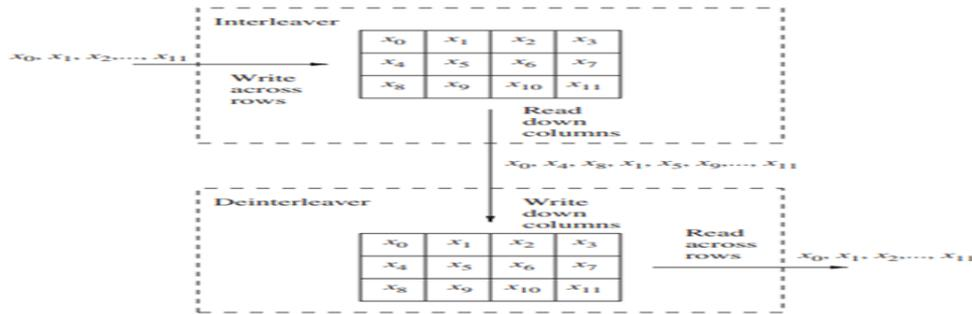
Figure 2.14: Block Matrix interleaver  $3 \times 4$  interleaver and deinterleaver.
