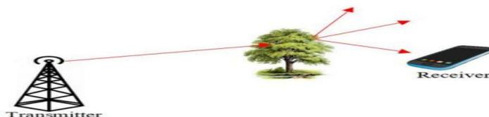
Figure 2.10: Scattering of the propagated signal.
