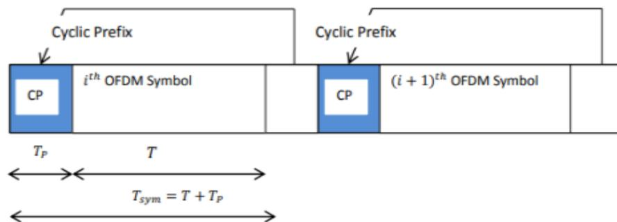
Figure 2.5 OFDM symbols with the cyclic prefix [21]
