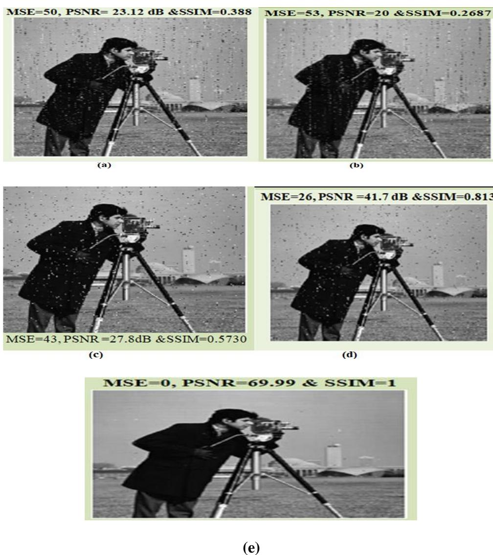
Figure 4.20 Sent Cameraman Image by Chaotic Interleaver in RS-OFDM Rayleigh fading channel (a)SNR=10 db (b)SNR=20 db (c) SNR=30db (d)SNR=40db (e) SNR=50db
