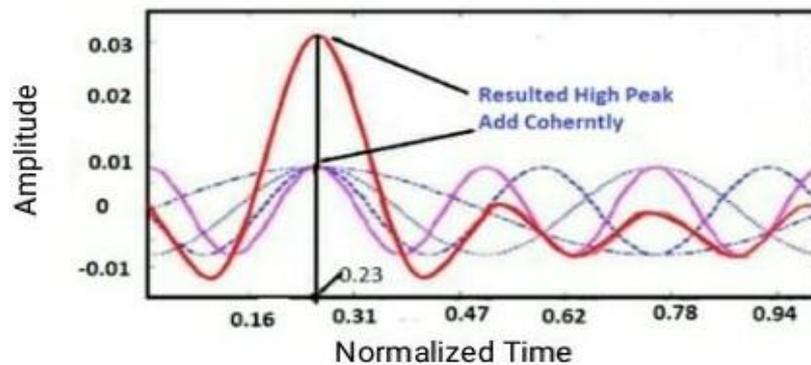
Figure 2.6: High Peak on OFDM System [44].
