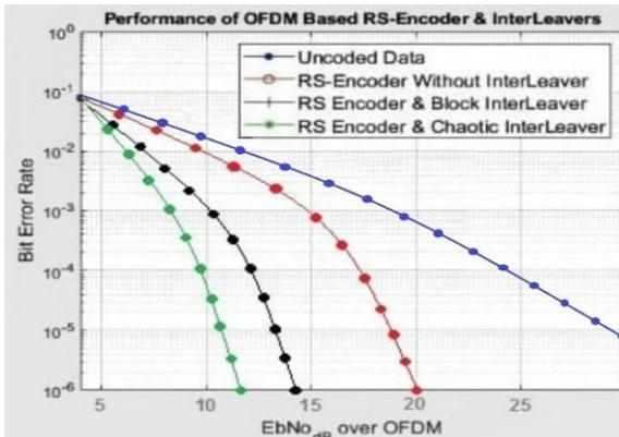
Figure 4.12 BPSK – RS OFDM with and without interleaver
