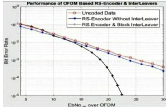
Figure 4.3 BER & SNR Interliver with RS-OFDM in 16-QAM
