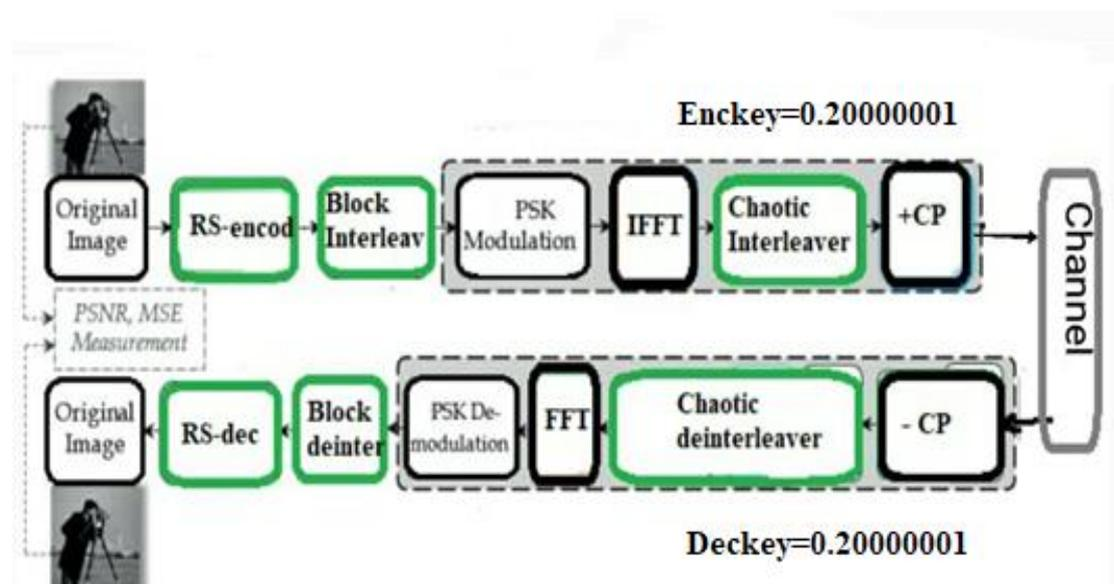
Figure 2.17 Show sent image in RS-OFDM with two interleaver
