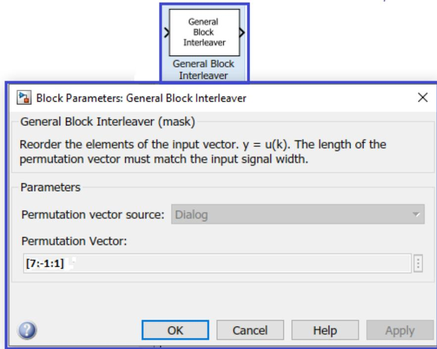
Figure 3.5 Block Interleaving
