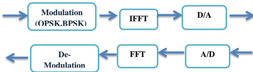
Figure 2.4 Basic model OFDM transmitter and receiver
