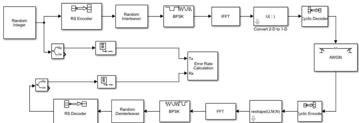
Figure 3.18 Simulink RS code OFDM with two interleaver
