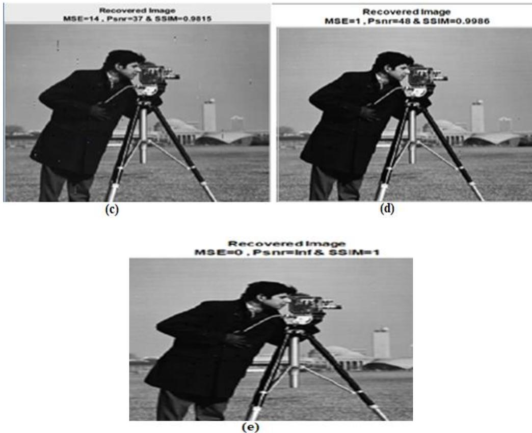
Figure 4.19 Sent Cameraman Image by Chaotic & Block Interleaver in RS-OFDM AWGNchannel (a)SNR=10 db (b)SNR=20 db (c)SNR=30db (d)SNR=40db (e) SNR=50db
