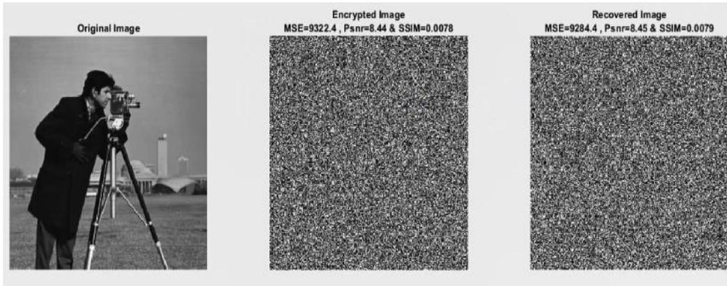
Figure 4.18 Sent cameraman image by Chaotic interleaver used Deckey=0.2000000
