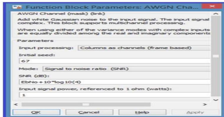
Figure 3.11 AWGN Parameters for OFDM Simulation
