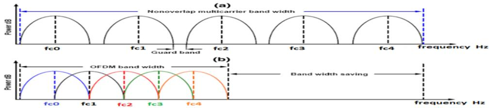
Figure 2.1 A comparison of single carriers and multicarrier techniques
