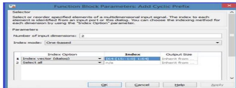
Figure 3.10 “Add Cyclic Prefix” Block Parameters
