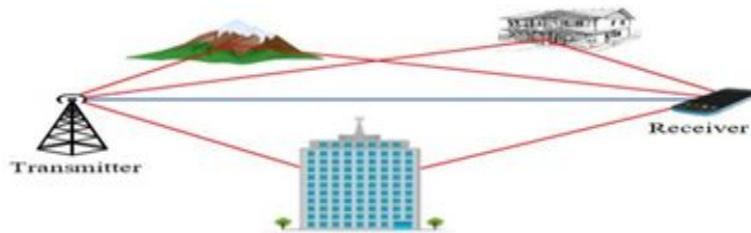
Figure 2.7 Multipath propagation. The blue line represents the LoS while the red one represents the NLoS[38]
