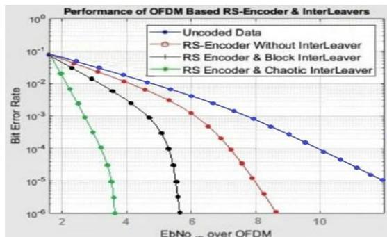
Figure 4.9 16PSK RS-code OFDM with and without interleaver
