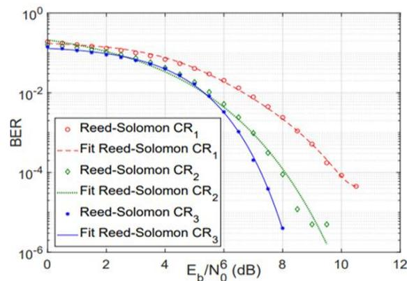
Figure 4.1 BER performance of the Reed-Solomon code for different coding rates  $CR_1$ ,  $CR_2$ ,  $CR_3$
