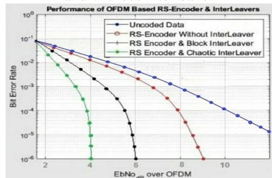
Figure 4.10 32 PSK RS-code OFDM with and without interleaver
