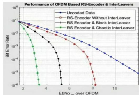
Figure 4.8 QPSK RS-code OFDM with and without interleaver
