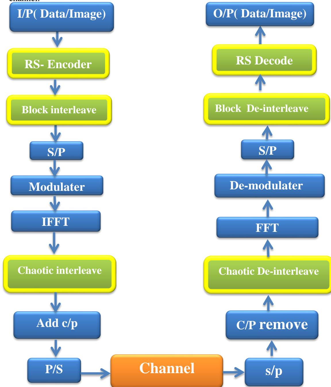
Figure 2.11 shows the improvement added to the system (OFDM)
