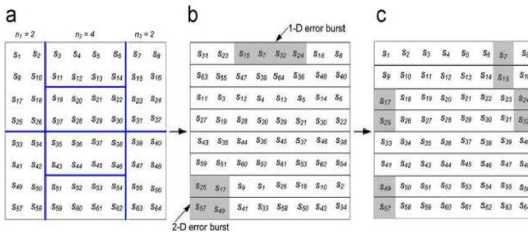
Figure 2.16 shows an example of the chaotic interleaving of an  $(8 \times 8)$  square matrix (i.e.  $N=8$ ). The secret key,  $S_{key}=[n_1, n_2, n_3]=[2,4,2]$ .
