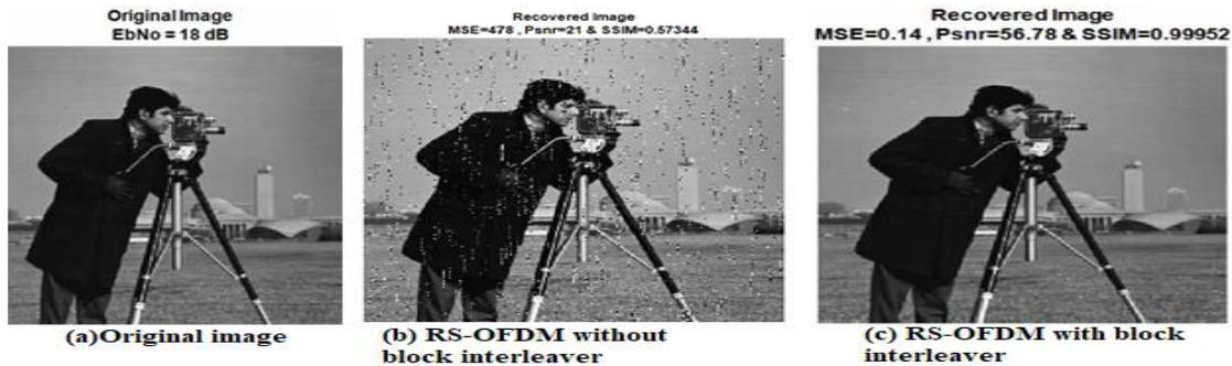
Figure 4.6 Sent cameraman image in 18 db in RSOFDM with Block Interleaver
