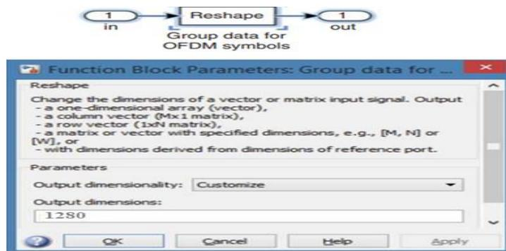
Figure 3.15 OFDM Symbols Block and Associated Parameters
