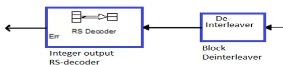
Figure 3.17 RS-decoder with Block de-interleaver
