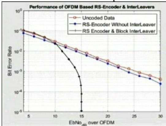
Figure 4.4 BER & SNR Interliver with RS-OFDM in QPSK
