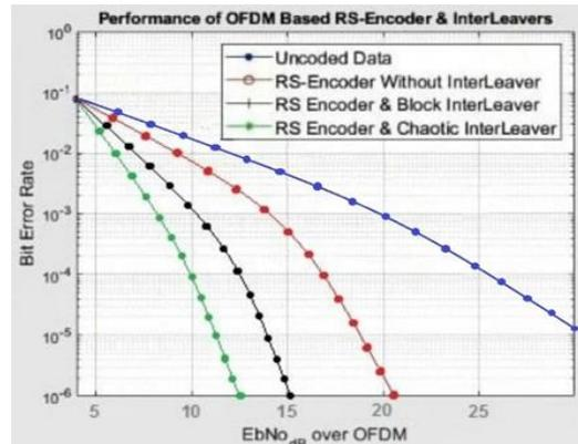
Figure 4.13 QPSK RS OFDM with and without interleaver
