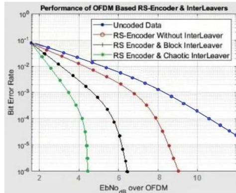
Figure 4.11 64 RS-code OFDM with and without interleaver
