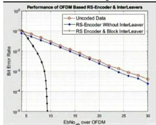
Figure 4.5 BER & SNR Interliver with RS-OFDM in BPSK
