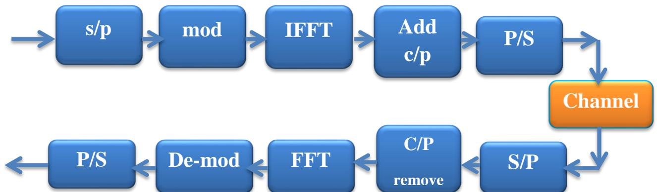
Figure2.2 Basic OFDM Transmitter and Receiver
