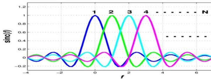
Figure 2.3 Frequency response of 4 subcarriers of OFDM signal
