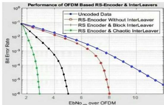
Figure 4.7 BPSK RS-code OFDM with and without interleaver
