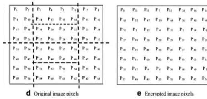
Figure 2.18 shows the chaotic interleaving of an (8 X 8) square matrix (i.e.
