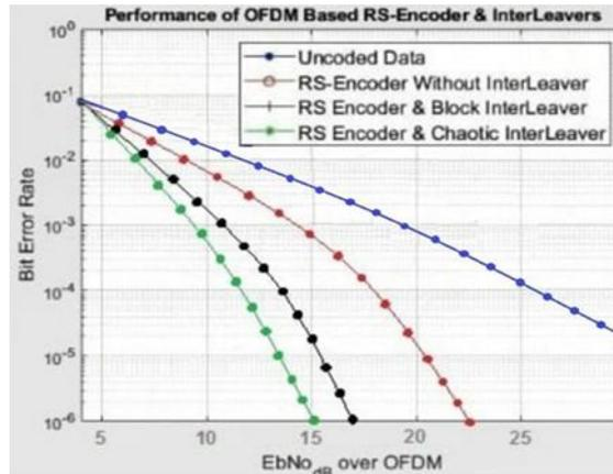
Figure 4.16 64-PSK RS OFDM RS-code OFDM with and without interleaver
