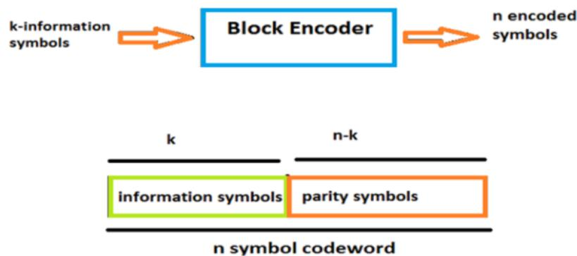
Figure 2.12: A block encoder and coding codeword
