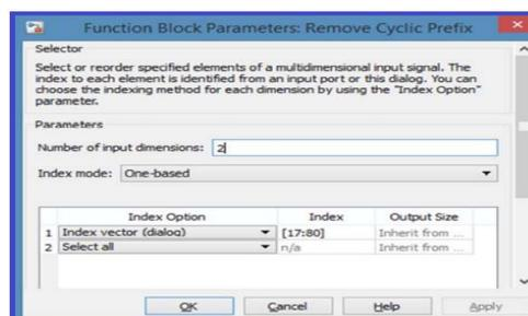
Figure 3.12 “Remove Cyclic Prefix” Block Parameters
