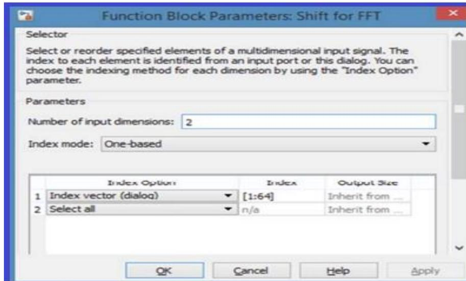
Figure 3.8 Selector Block, Shift for IFFT
