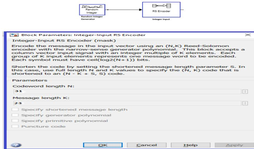
Figure 3.4 Setting of the RS encoder block
