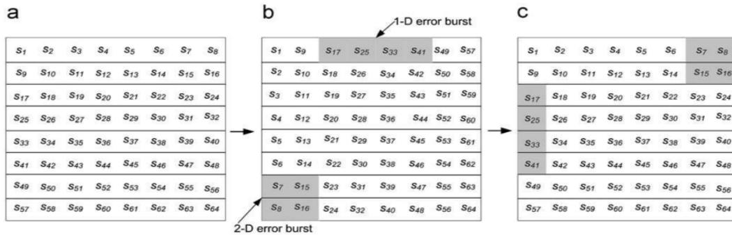
Figure 2.15 Block interleaving of an 8X 8 matrix.
