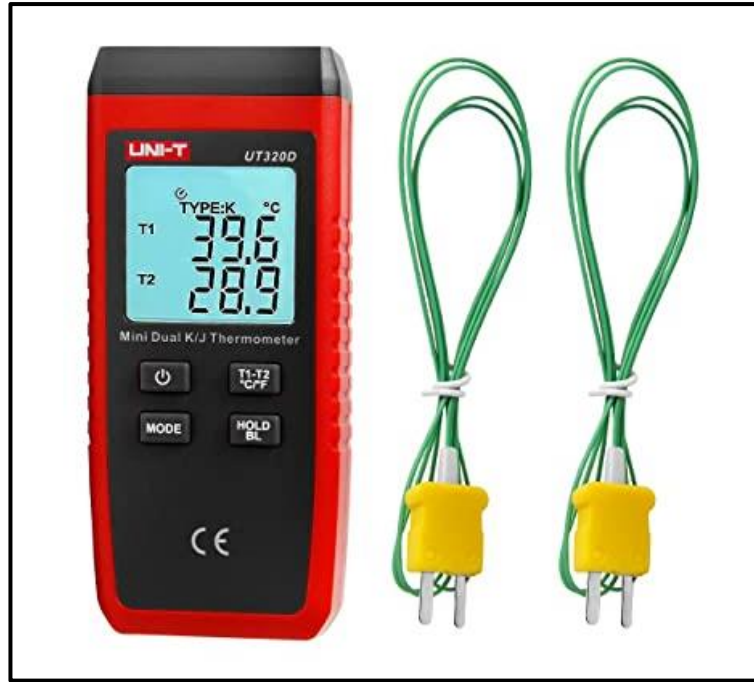
Figure 4.14. Mini Dual-channel K/J Thermometer, UT-320D type.
