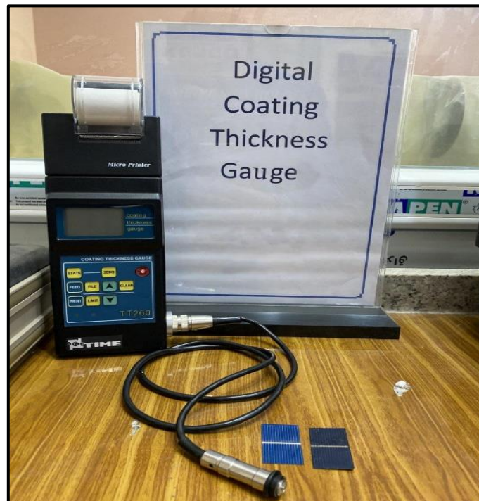
Figure 4.11. Digital coating thickness gauge TT-260.
