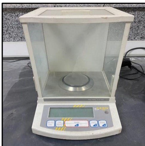
Figure 4.8. KERN-ABS Sensitive electronic scale
