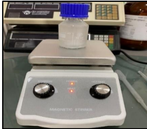
Figure 4.9. The magnetic stirrer, model SH-2.
