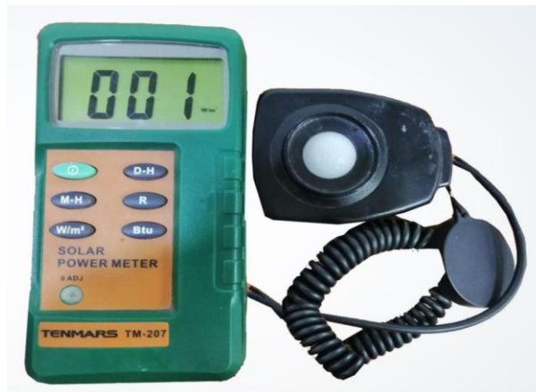
Figure (4.9) Solar radiation measurement device (Pyranometer)
