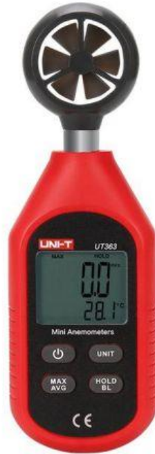
Figure (4-11) Air flowmeter
