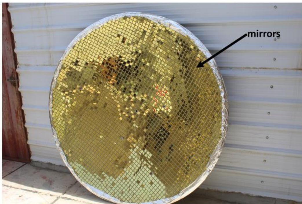
Figure (4.5): Parabolic dish after covering its surface with glass mirrors
