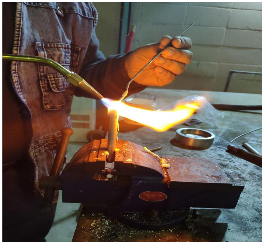
Figure (4.10): The process of welding the fins after filling them with nanomaterial
