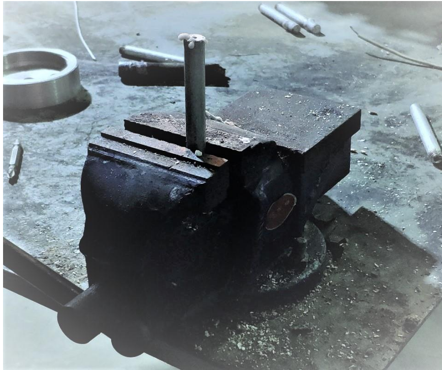
Figure (4.9): The process of filling nanomaterial into the inner holes of the fin
