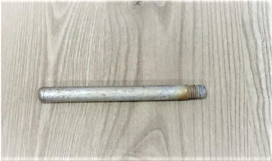
Figure (4.11): The final shape of the fin after filling it with nano-material and welding it
