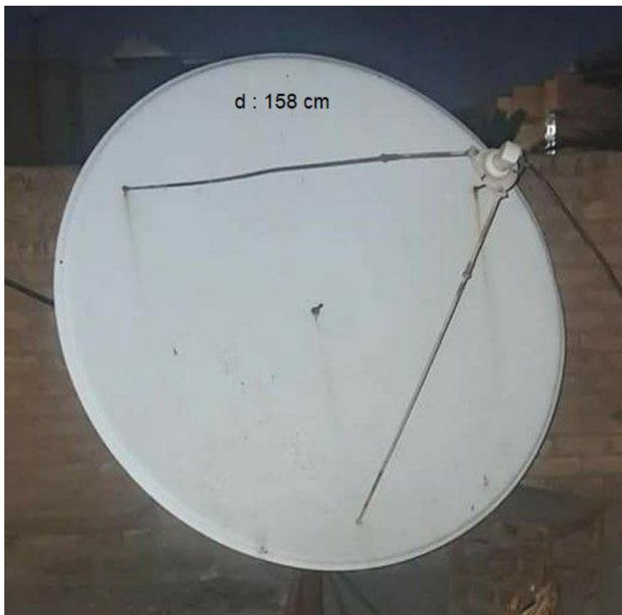
Figure (4.4): Photograph of a parabolic dish (antenna)
