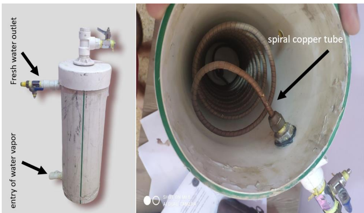
Figure 4.18: a steam condensing system.
