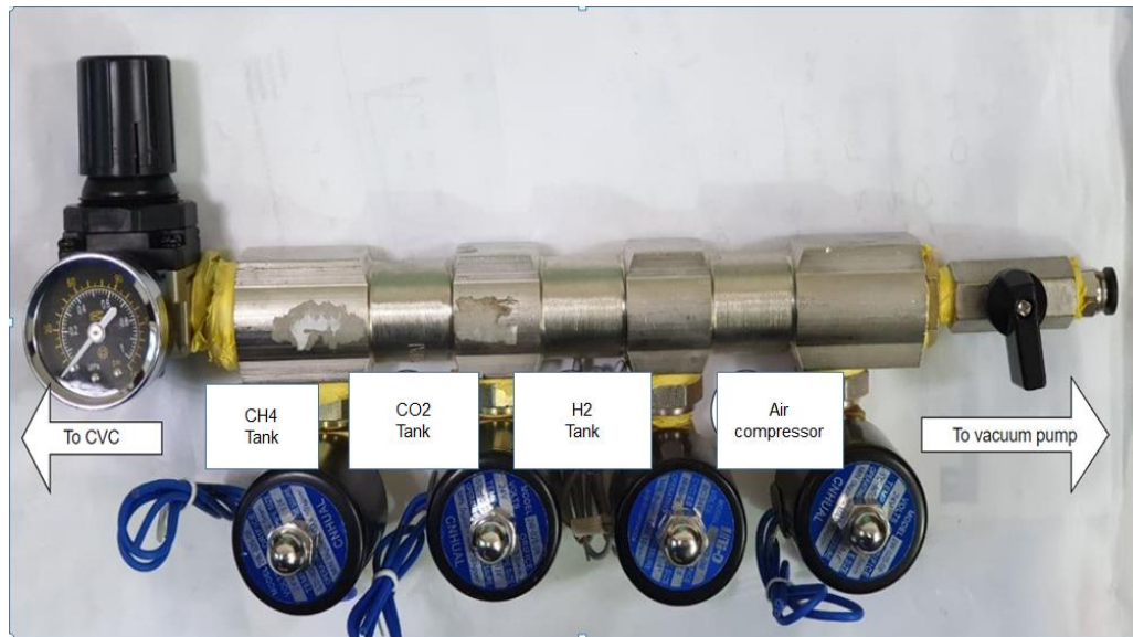
Figure 3.8- The gas manifold.
