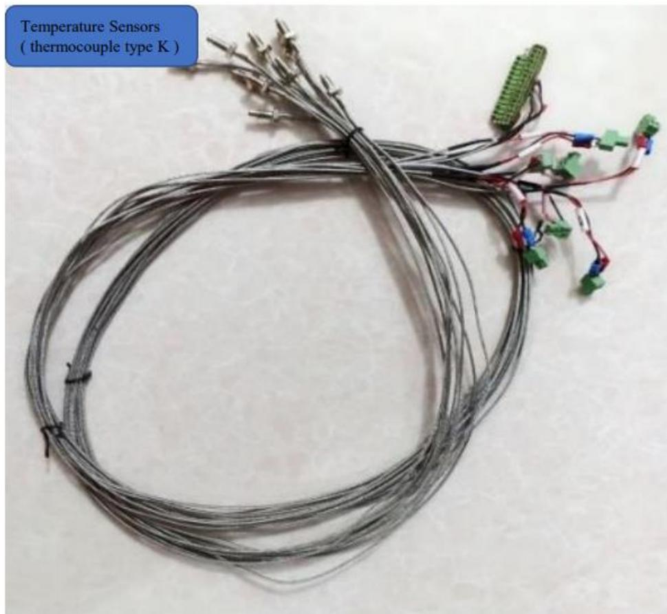
Fig. 4.13: Seventeen temperature sensors type K
