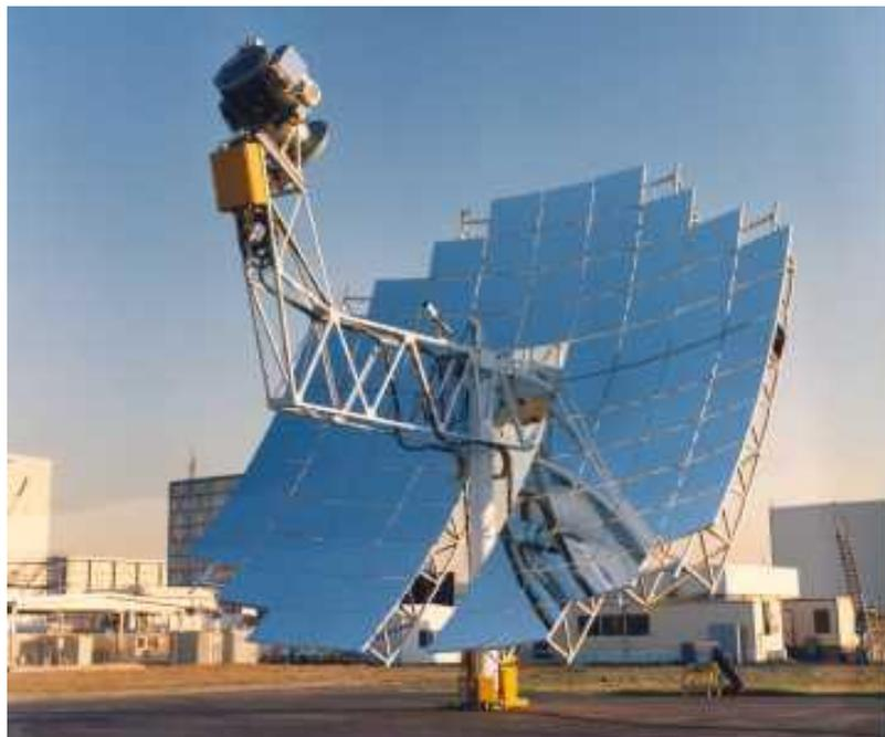
Fig. 1.4: A point focus solar collector [4]
