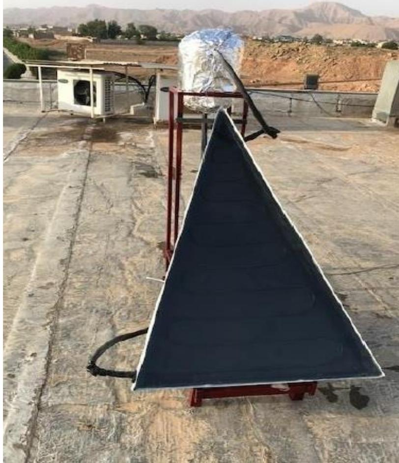
Fig. 2.8: Photo of the triangular flat plate collector [12].
