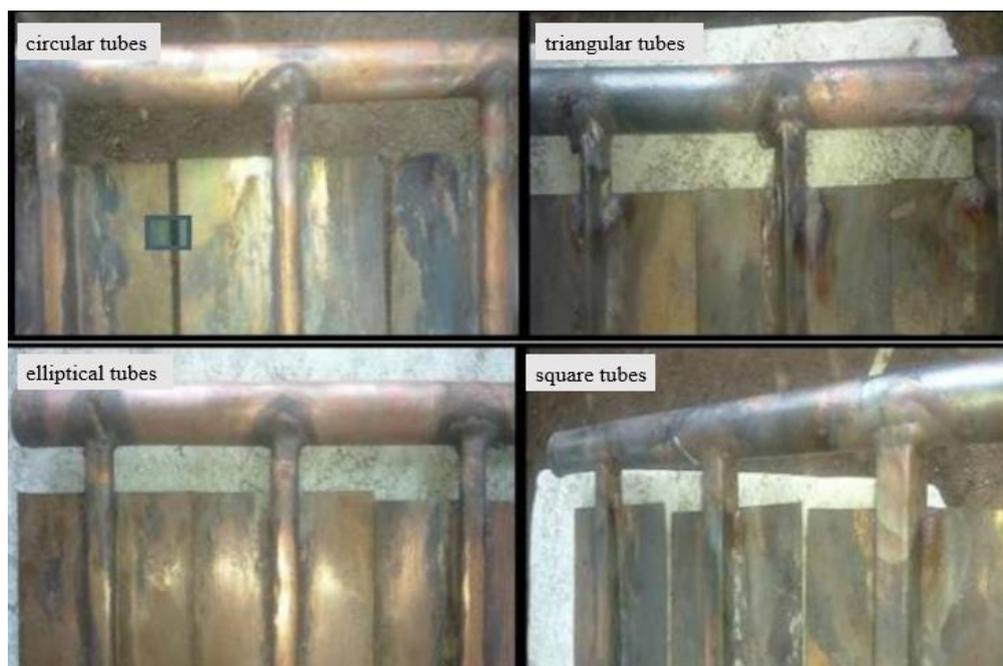
Fig. 2.5: various shapes of tubes circular, elliptical, triangular & square [9].
