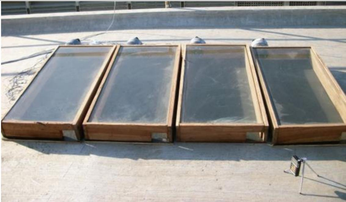
Fig.2.19:Solar collector models with 3,4,5, and 6 mm glass thick, respectively[24].
