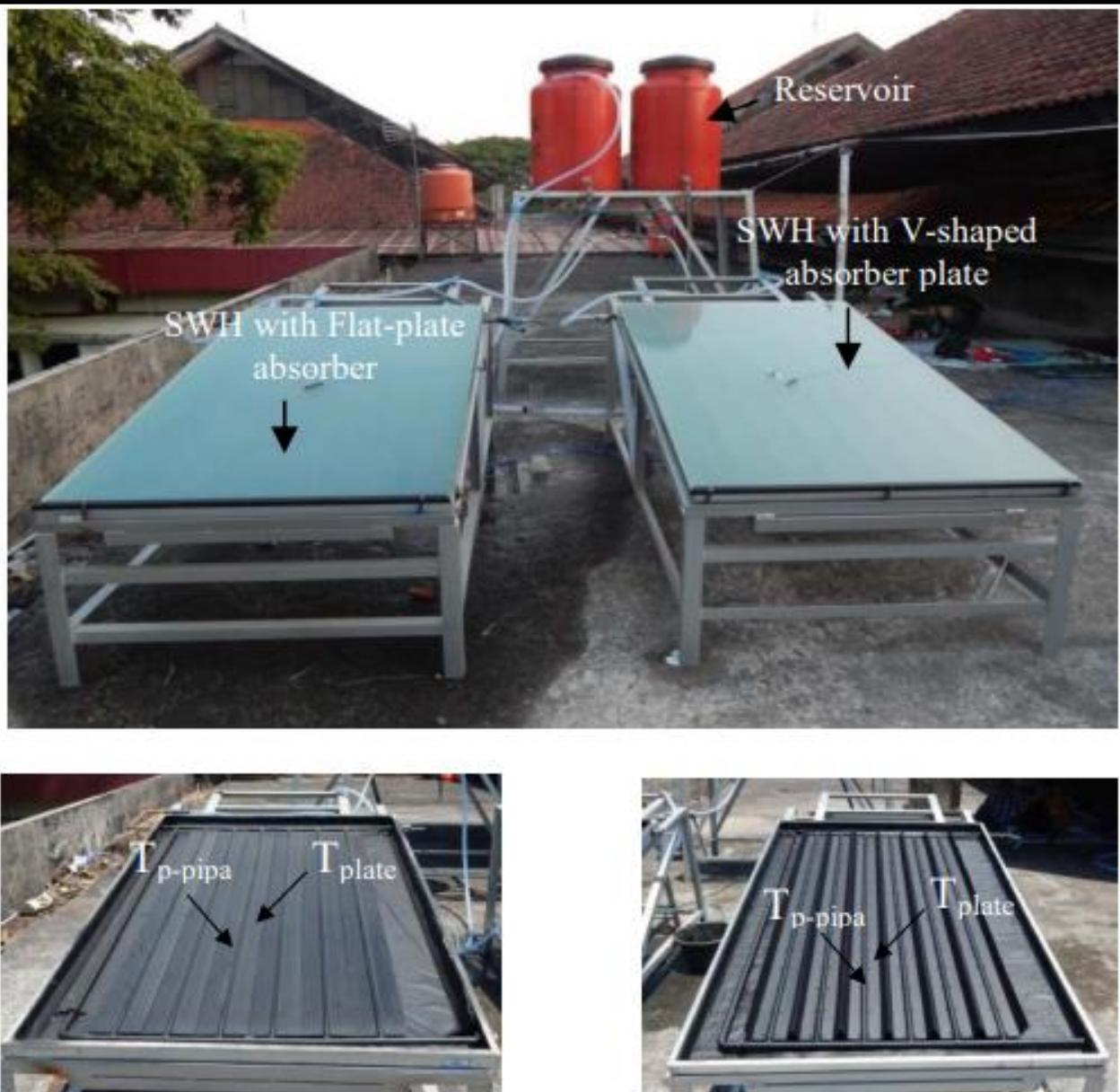
Fig. 2.12: Solar water heating system with (a) flat-plate absorber plate(b) V-shaped absorber plate [16].
