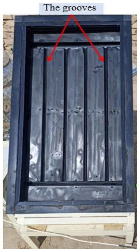
Fig. 3.2: The V- grooves absorber plate
