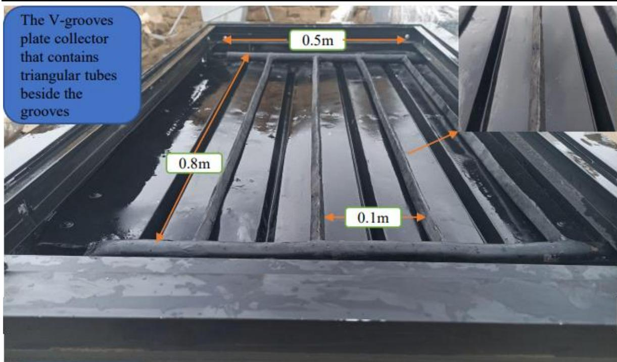
Fig. 4.7: The V-grooves plate solar collector that contains triangular tubes beside the grooves
