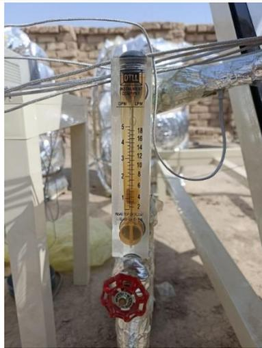
Fig. 4.15 Volumetric water flow meter
