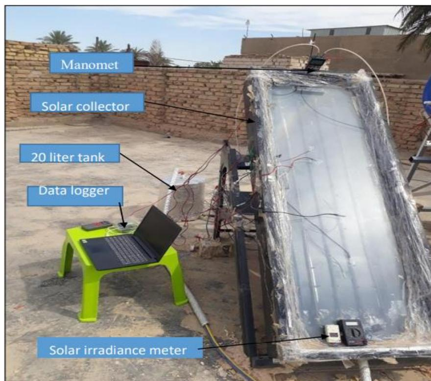
Fig. 2.25: flat plate solar collector [31].
