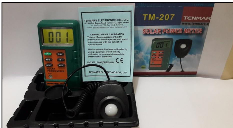
Figure (4-9): Solar power meter.
