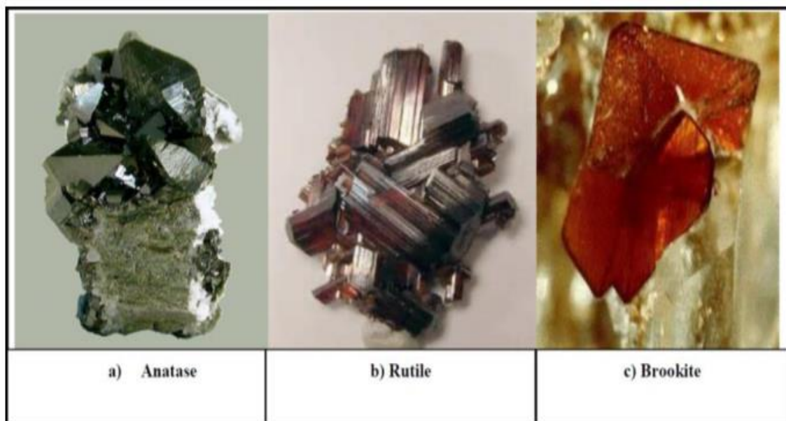
Figure 4. 2: Crystalline Forms of Titanium Dioxide, Anatase, Rutile, and Brookite [81].
