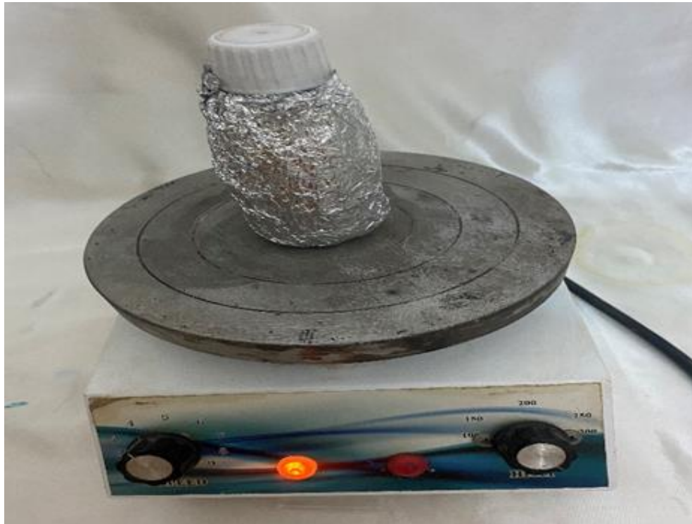
Figure 4. 10: stirring electrolytes in a dark container using a magnetic stirrer.
