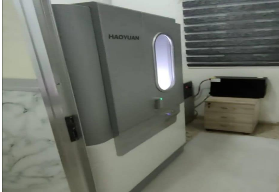
Figure 4. 25: X-Ray device is used to diagnose the crystal structure of membranes.
