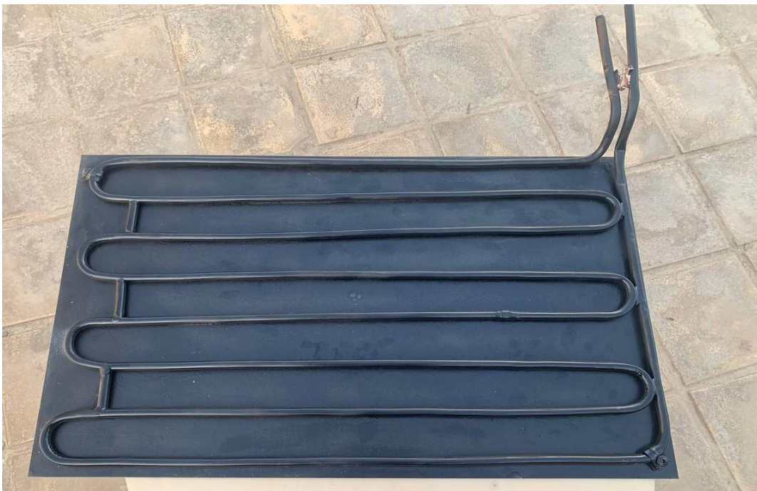
Figure. (3.11): Images of heat exchanger with galvanized plate.
