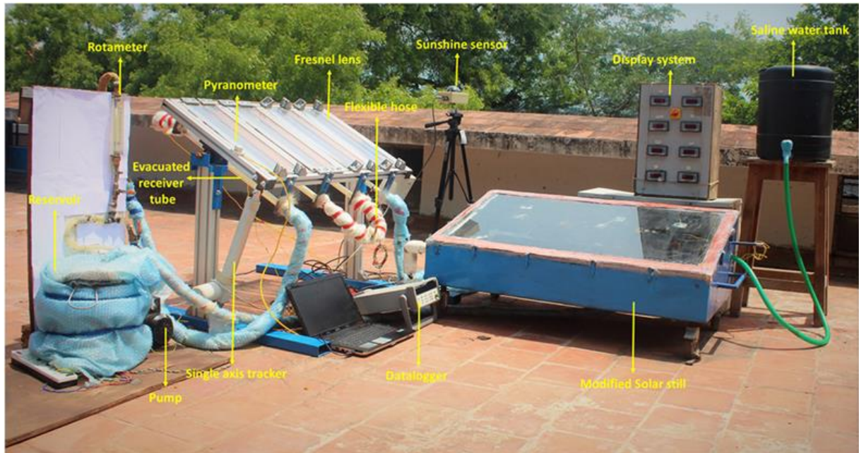
Figure (2.4): Pictures of a modified solar distillation system (MSDS) [37].
