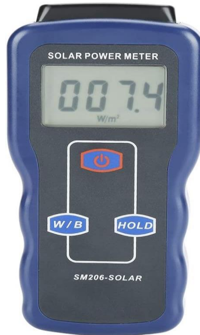
Figure (3.20): Measure the intensity of solar radiation.
