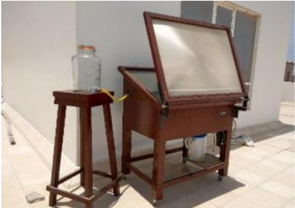
Figure (2.5): Photograph of a solar still with a Fresnel lens [39].
