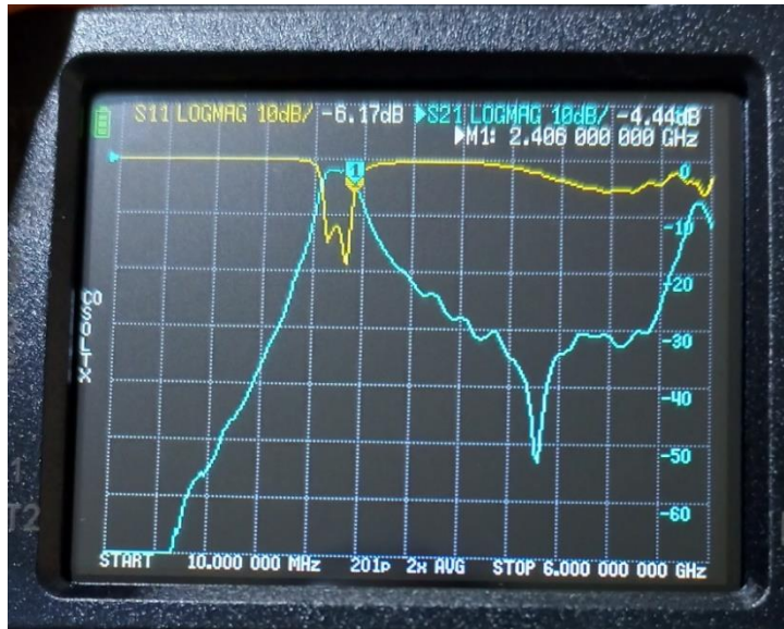
Figure 3.22. Measuring S-Parameters with VNA
